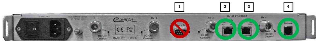
**Figure 5-1. CDD-564A/L Rear Panel Connections to User PC**
