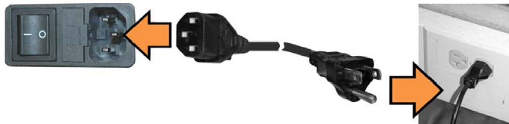
Figure 3-11. AC Power Connection
