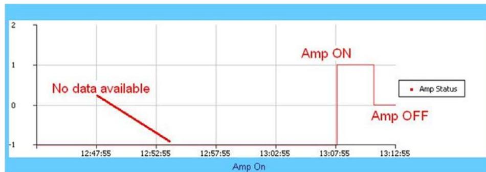
This graph displays the state of the RF amplifier (**On/Off**). As per this example:
