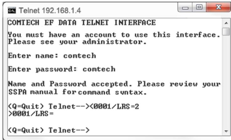
Figure 4-5. Telnet Login and Remote Command Execution
