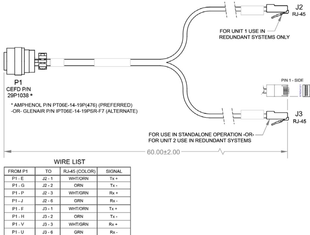
**Figure A-2. Ethernet Interface Cable (CEFD P/N CA-0000352, part of KT-0000203)**
