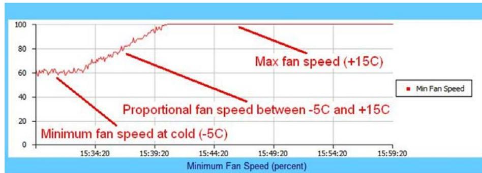
This graph displays the slowest fan speed of any of the fans installed in the system. This example demonstrates the fan running at minimum, proportional, and maximum speeds. Note that:
