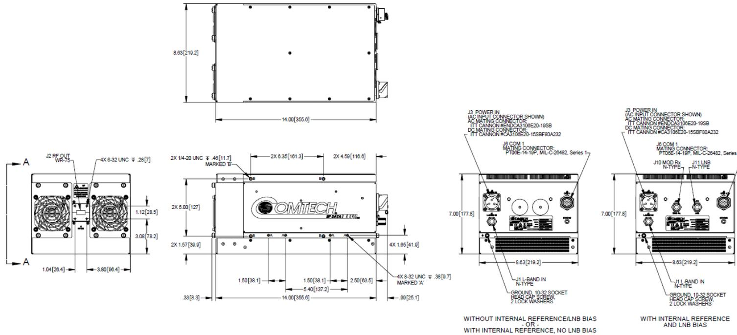
Figure 1-5. L-GaN 100 W Ku-Band Dimensional Envelope (1 of 2)
