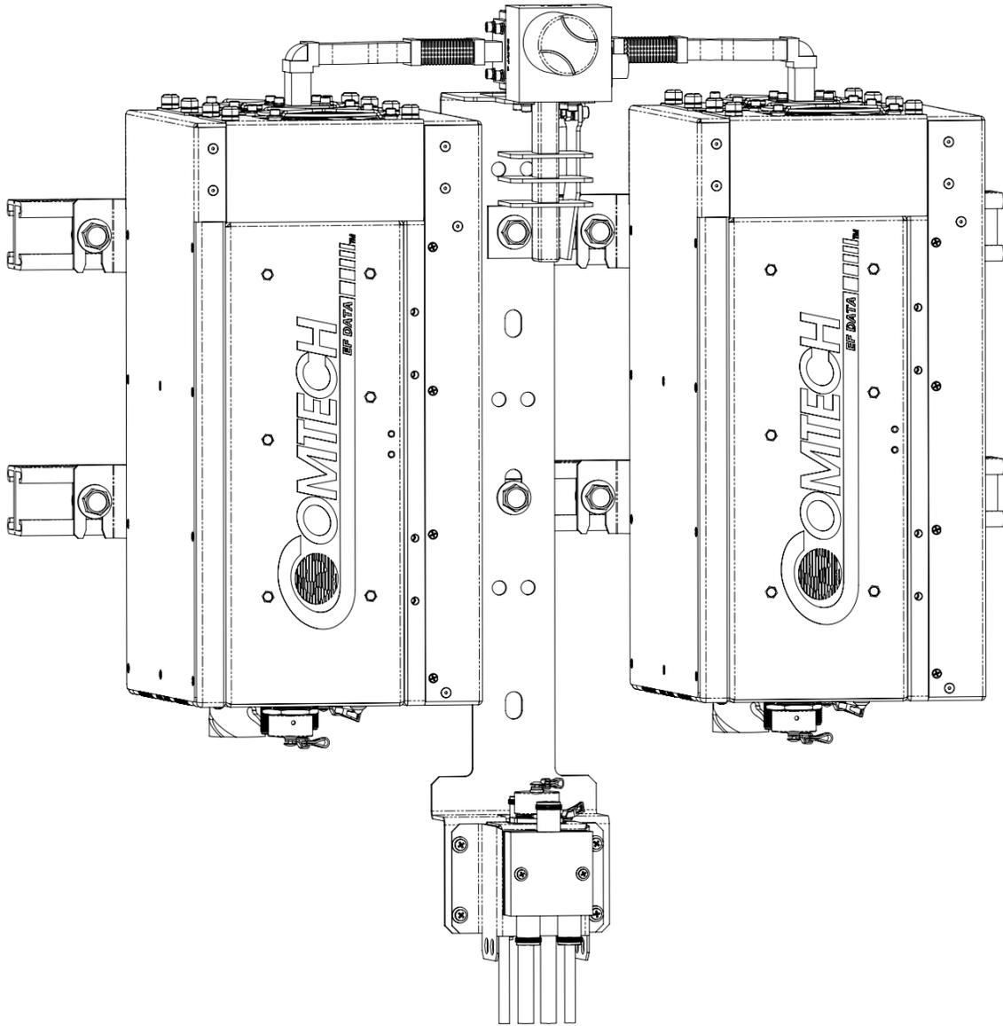
**Figure B-15. KT-0021435 LGaN 100 W 1:1 Redundant Ku Switch and Mounting Kit – Assembled Isometric View**
