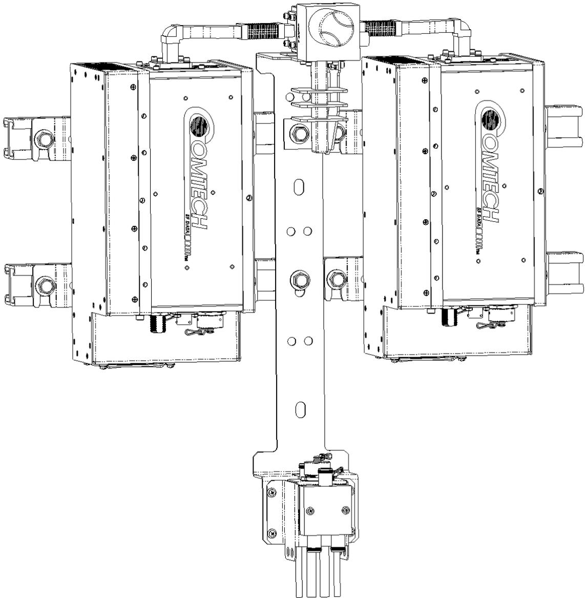
**Figure B-13. KT-0021223 LGaN 50 W 1:1 Redundant Ku Switch and Mounting Kit –
