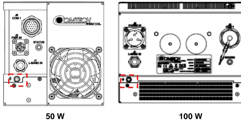
Figure 2-5. LGaN Ground Connector Locations
