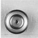
The RF input connector is a Type 'N' female connector. Labeled '**J1 | LBAND IN**' on the L GaN 50 W and 100 W models, typical input levels (-30 dBm) depend on desired output power and unit attenuation. To prevent damage to the L GaN, RF input levels should not exceed +15 dBm.
