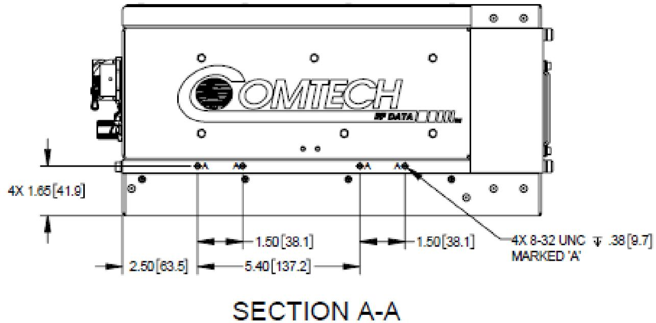
Figure 1-6. L-GaN 100 W Ku-Band Dimensional Envelope (2 of 2)
