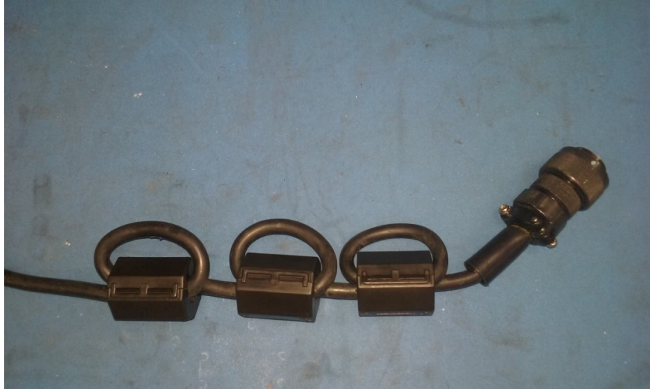
Figure 2-3. Ferrite Beads added to AC Power Cable
