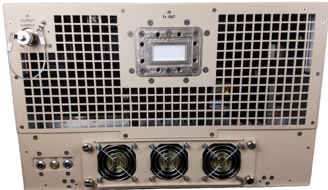
Figure 1-1. TRP1000-4450-OD C-Band Outdoor Amplifier
