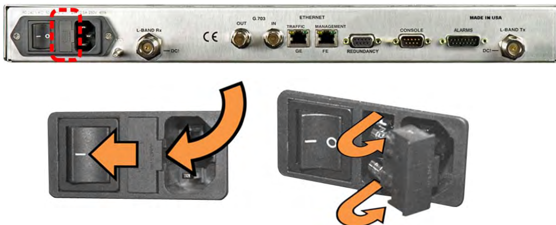
Figure 3-7. Replace the AC Fuses
