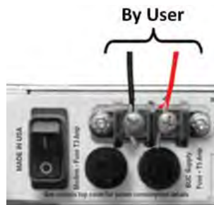
Figure 3-9. Apply DC Power to the Unit
