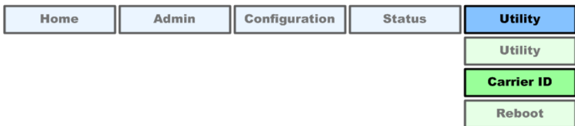
Figure F-1. CDM-840 HTTP Interface and Menu Tree – Carrier ID Operation (FW Ver. 1.6.2.X)
