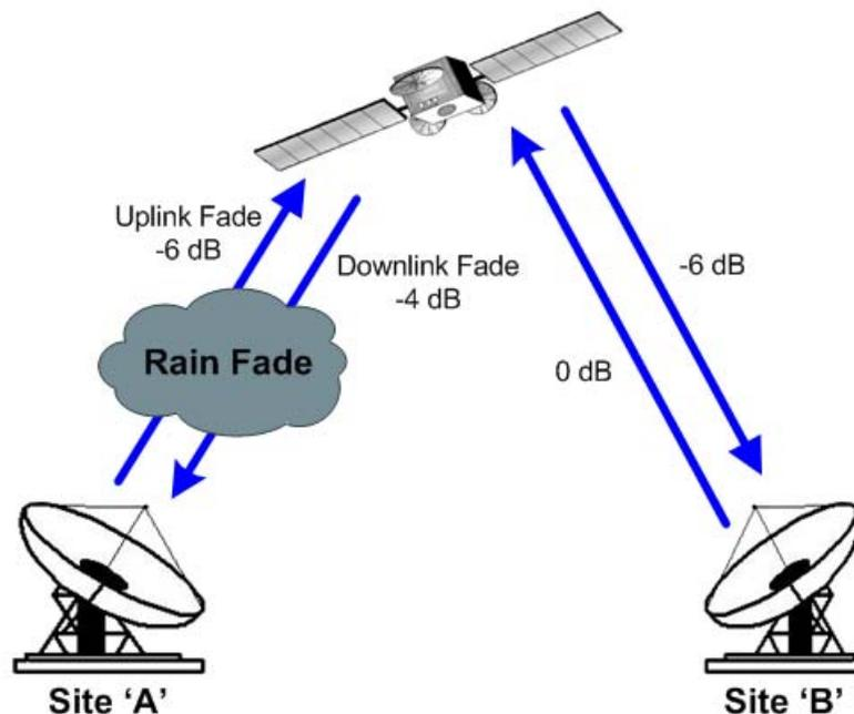
**Figure 9-12. Link With Fading At Site 'A'**
