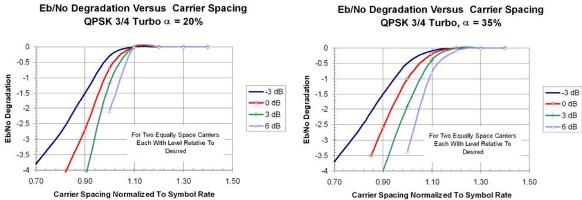
Figure 9-4. QPSK 3/4 Turbo degradation versus relative carrier spacing (for two adjacent carriers)
