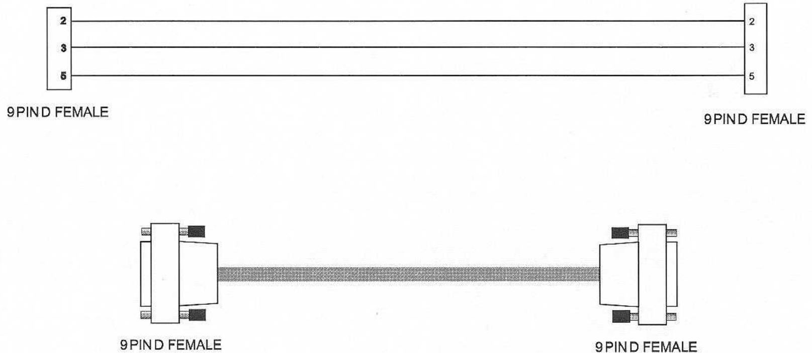
**Figure A-4. Switch Programming Cable**
