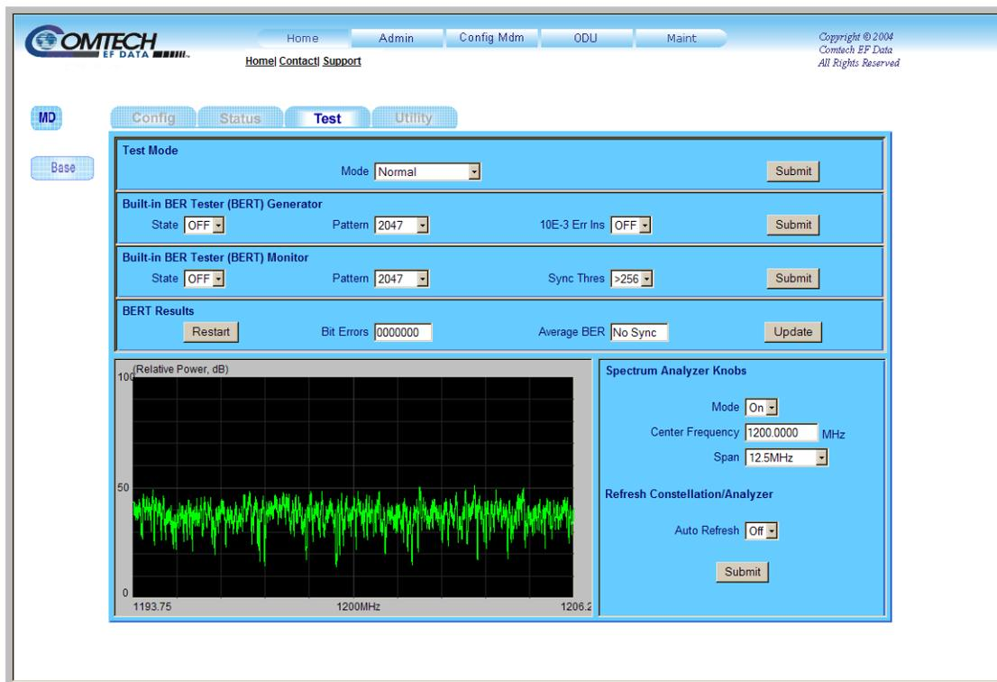
Figure 6-14. Nested Test Page with Spectrum Analyzer Mode 'On' – Rx, MD
