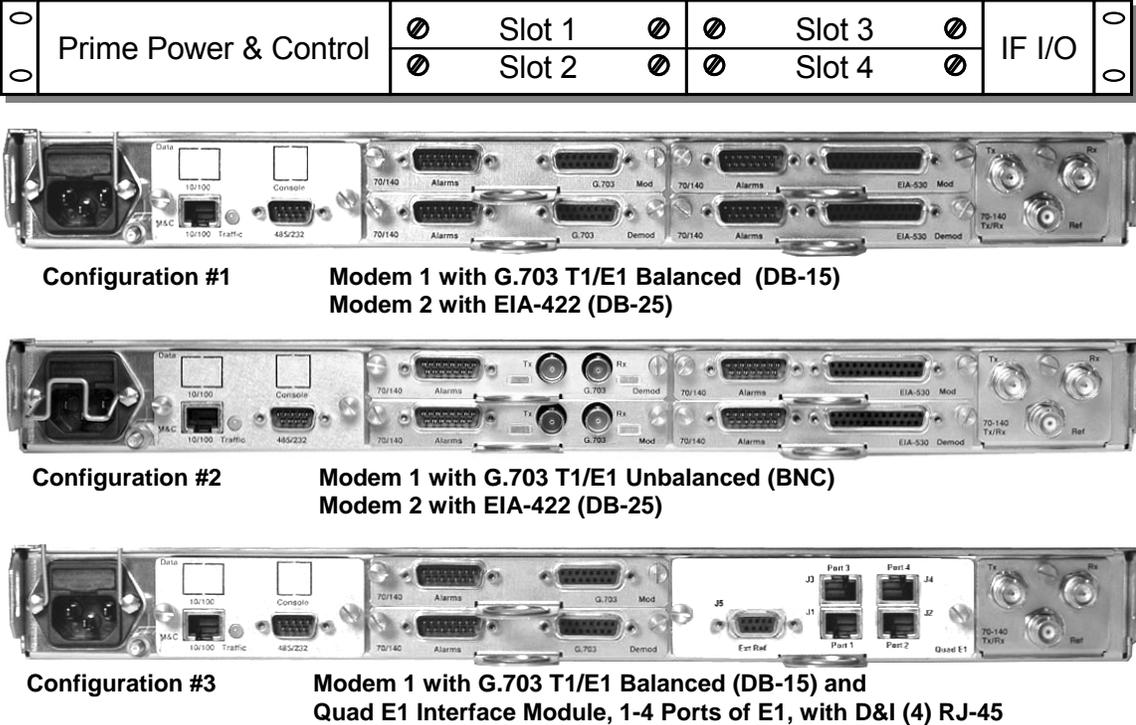
Figure 3-1. CDM-Qx/QxL Rear Panel Configuration Examples
