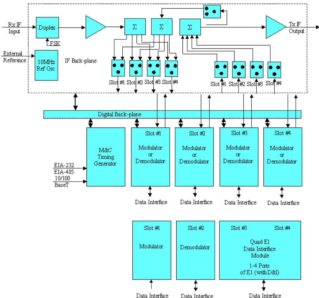
**Figure 1-2. CDM-Qx/QxL Open Network Satellite Modem Block Diagrams**
