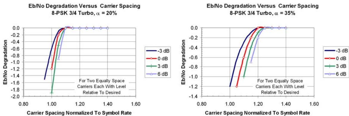
Figure 9-5. 8-PSK 3/4 Turbo degradation versus relative carrier spacing (for two adjacent carriers)
