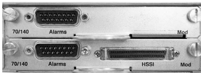
Figure 3-3. HSSI Interface Example
