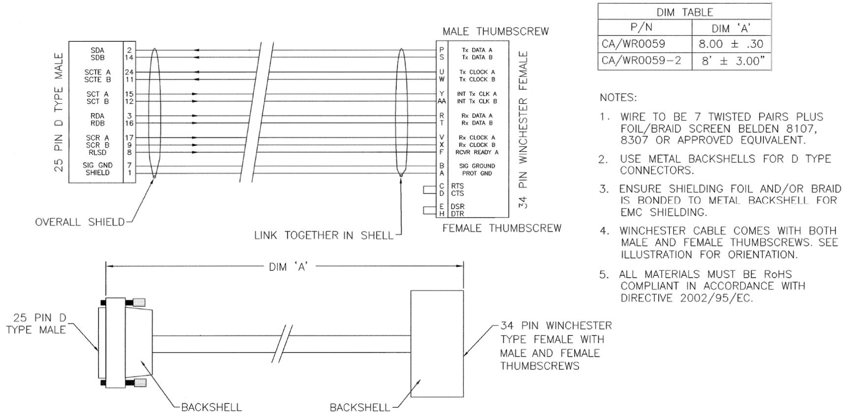
Figure A-2. : EIA-530 to V.35 DCE Conversion Cable (CA/WR0059)
