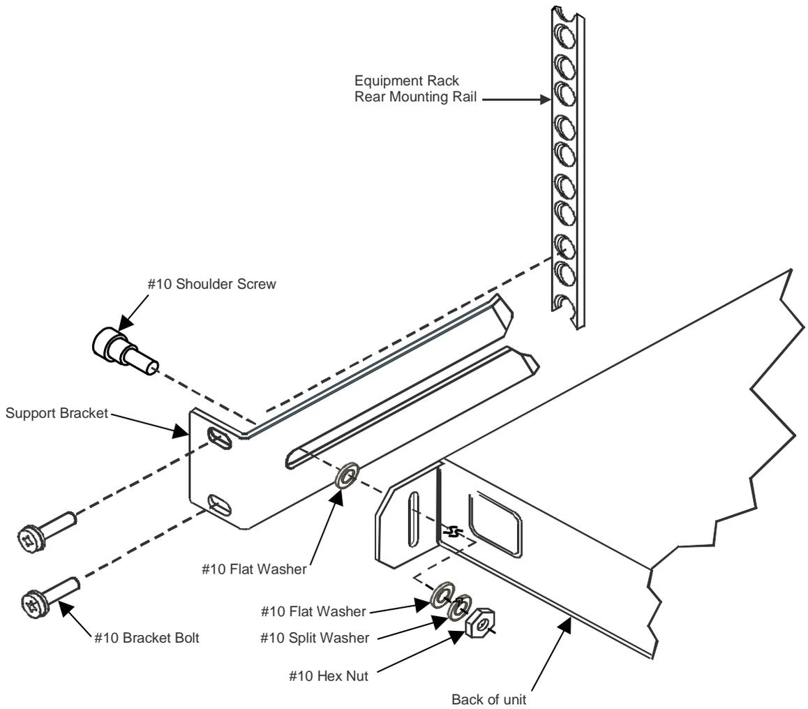
**Figure 2-1. Installation of Optional Rear-Mounting Support Brackets**
