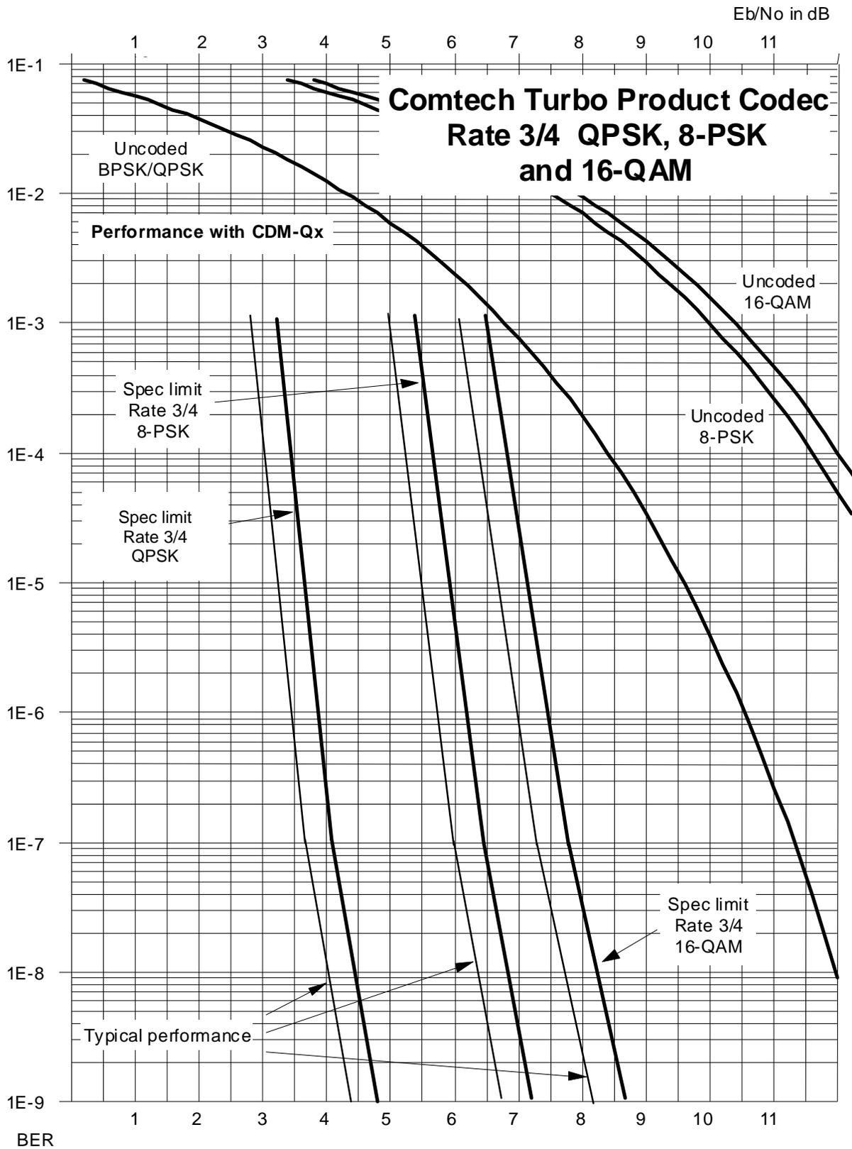
Figure 6-4. Comtech EF Data Turbo Product Codec Rate 3/4 QPSK, 8-PSK and 16-QAM
