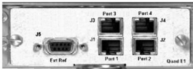
The Quad E1 Data interface card allows the user to connect one to four different terrestrial E1 ports, with each port independently configurable for full E1 (framed or unframed E1 data), or fractional E1 (with D&I). These four RJ-45 ports – labeled **J1 Port 1** through **J4 Port 4**, respectively, on the interface card – must be synchronized to each other.
