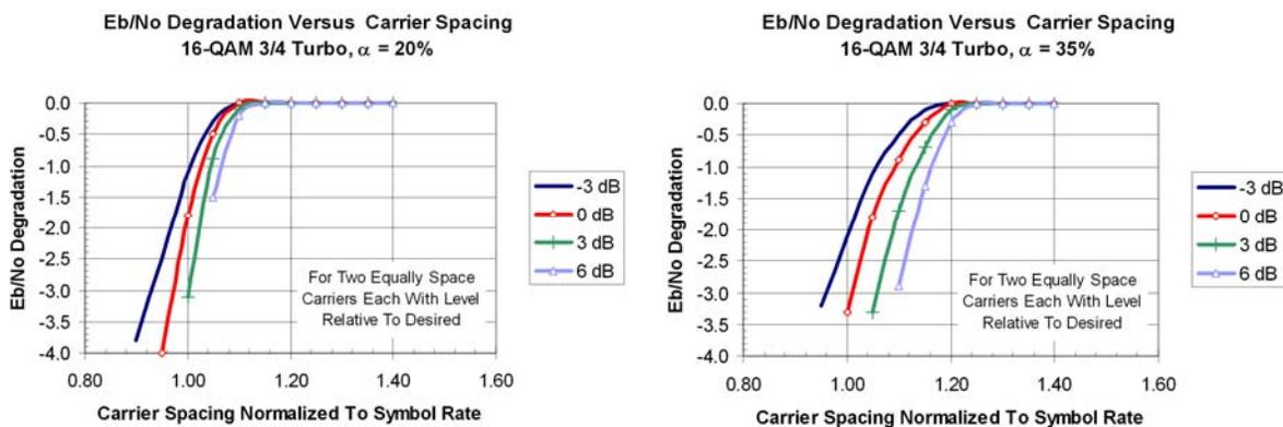
Figure 9-6. 16-QAM 3/4 Turbo degradation versus relative carrier spacing (for two adjacent carriers)
