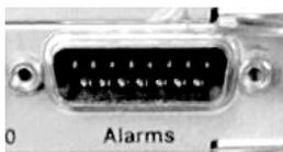
All available data interface modules contain a 15-pin 'D' type male (DB-15M) **Alarms** connector. The Alarms connector provides the user with access to the Form-C relay contacts, which indicate the fault status of the unit. These are typically connected to an external fault monitoring system, often found in satellite earth stations.
