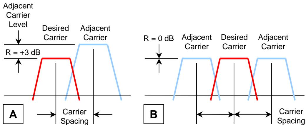
**Figure 9-3. Adjacent Carrier: Case A (As Tested) and Case B (As Plotted)**
