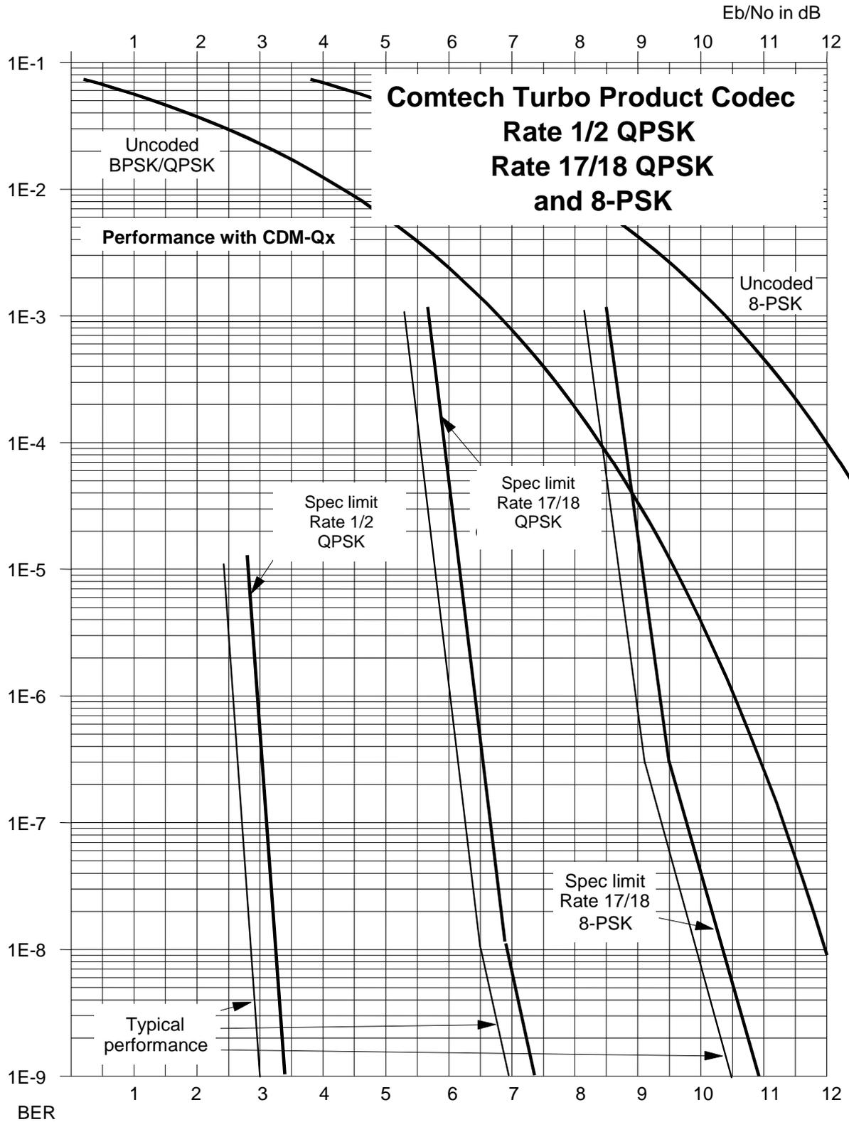
Figure 6-6. Rate 1/2 QPSK, Rate 17/18 QPSK and Rate 17/18 8-PSK
