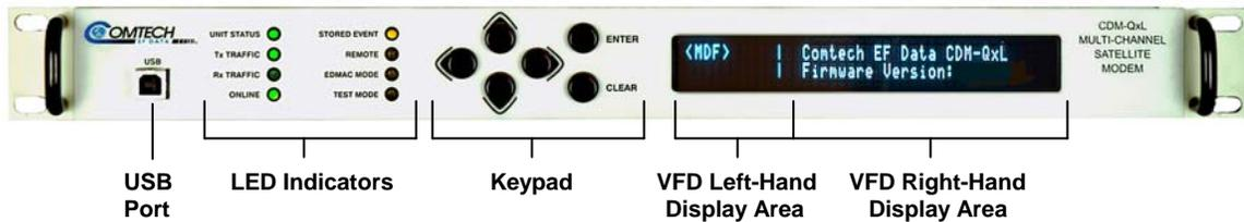
**Figure 5-1. CDM-Qx/QxL – Front Panel View**
