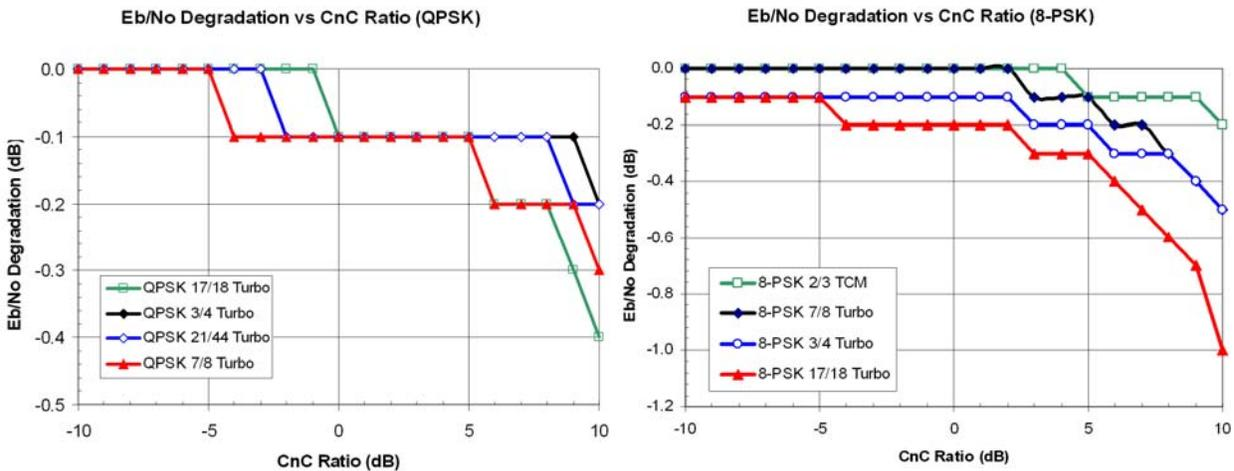
**Figure 9-9. CnC Ratio For QPSK and 8-PSK**
