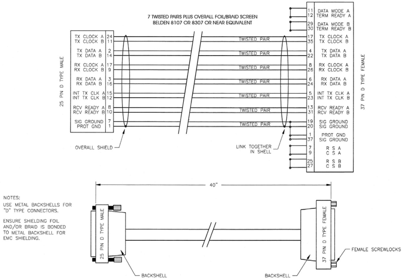
Figure A-1. : EIA-530 to RS-422/449 DCE Conversion Cable (CA/WR0049)
