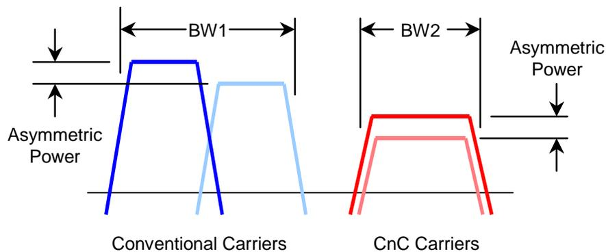
**Figure 9-13. Asymmetric Link (Same Data Rate, Different Antennas)**
