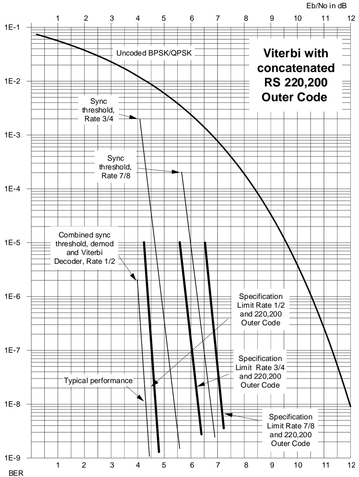
Figure 6-2. Viterbi with Concatenated R-S Outer Code
