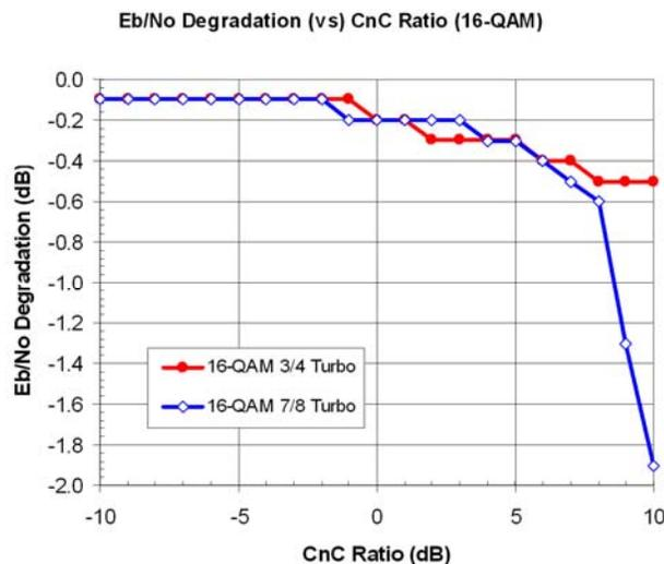
**Figure 9-10. CnC Ratio For 16-QAM**
