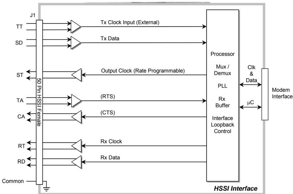
**Figure 3-2. HSSI Interface Block Diagram**
