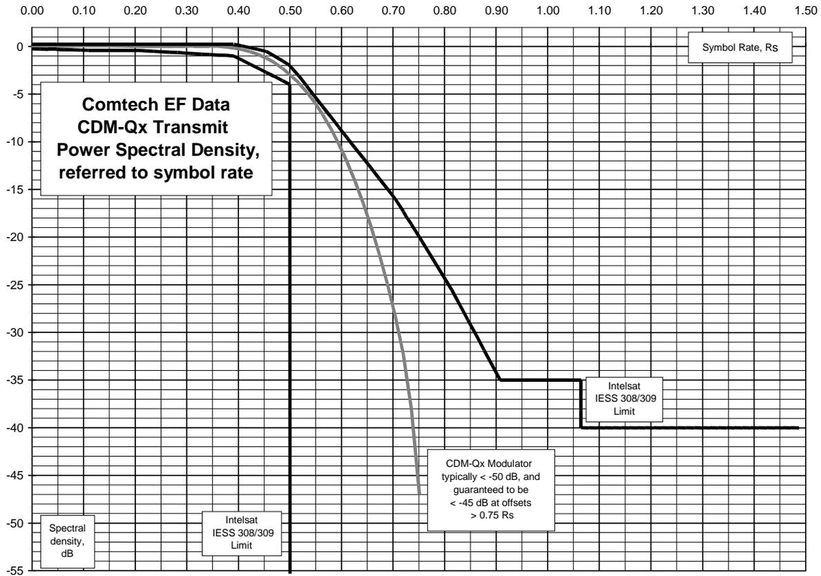
Figure 1-6. Power Spectral Density Chart
