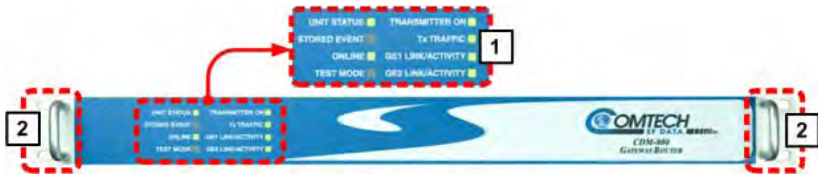
Figure 1-13. CDM-800 – Front Panel View
