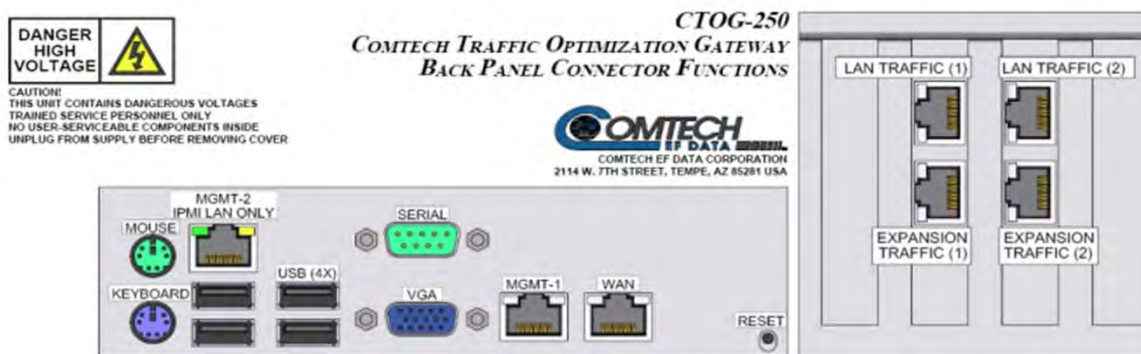
Figure 3-6. CTOG-250 Back Panel Connectors Diagrams – Enlarged Detail
