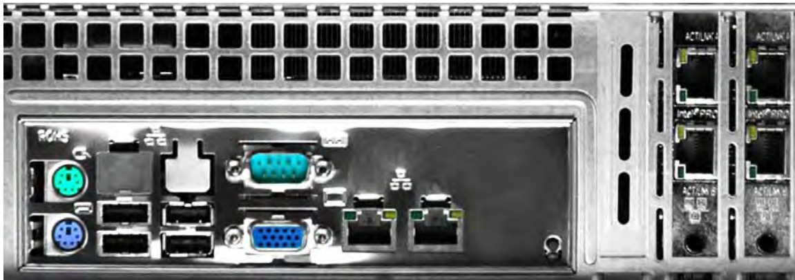
Figure 1-12. CTOG-250 Unit Back Panel Traffic and Management Connectors
