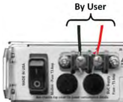
Figure 3-18. Apply DC Power to the CDM-800
