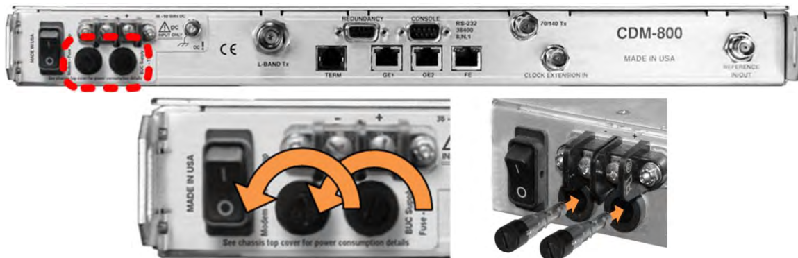
Figure 3-19. Replace the CDM-800 DC Fuses
