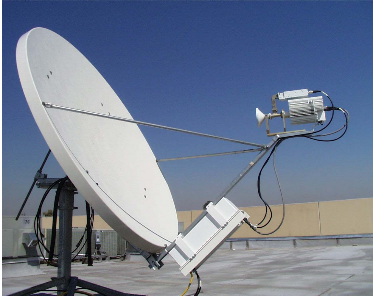
Figure C-1. KST-2000A Single Thread System Installed on Spar Arm.
