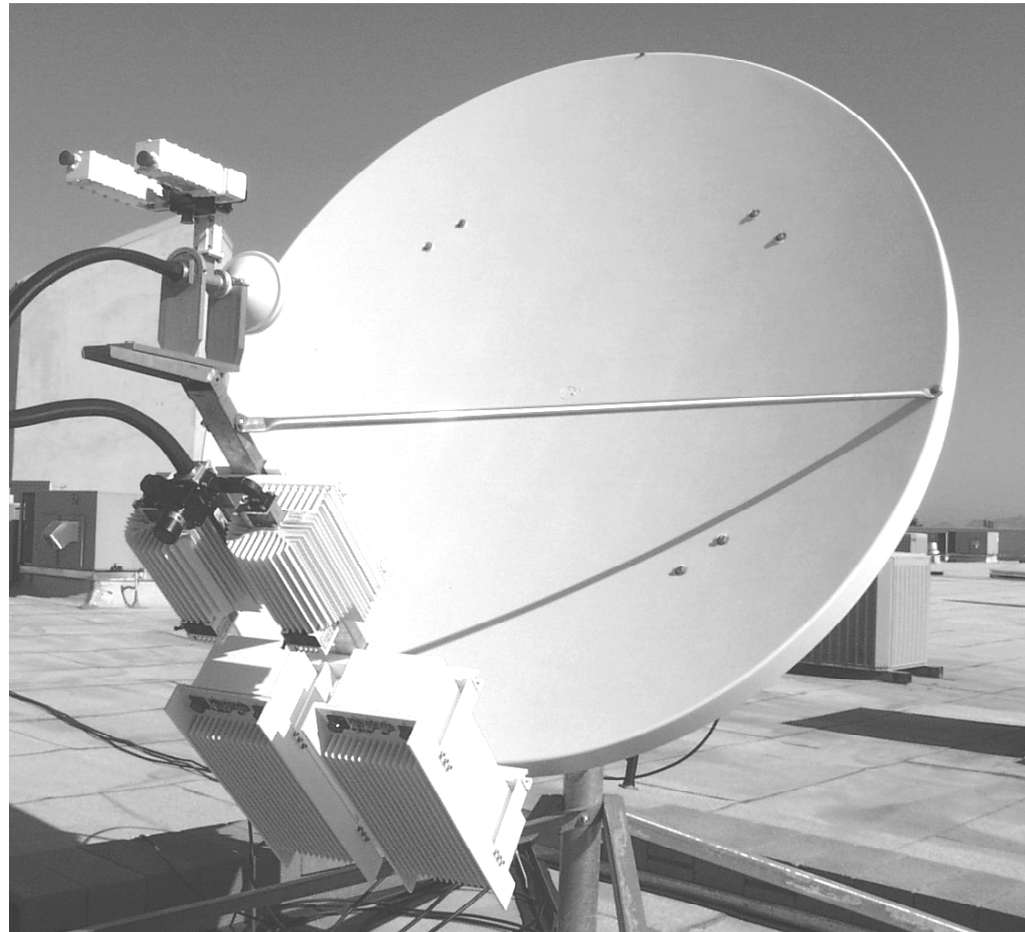
Figure D-1. 1:1 System Installed on Spar Arm
