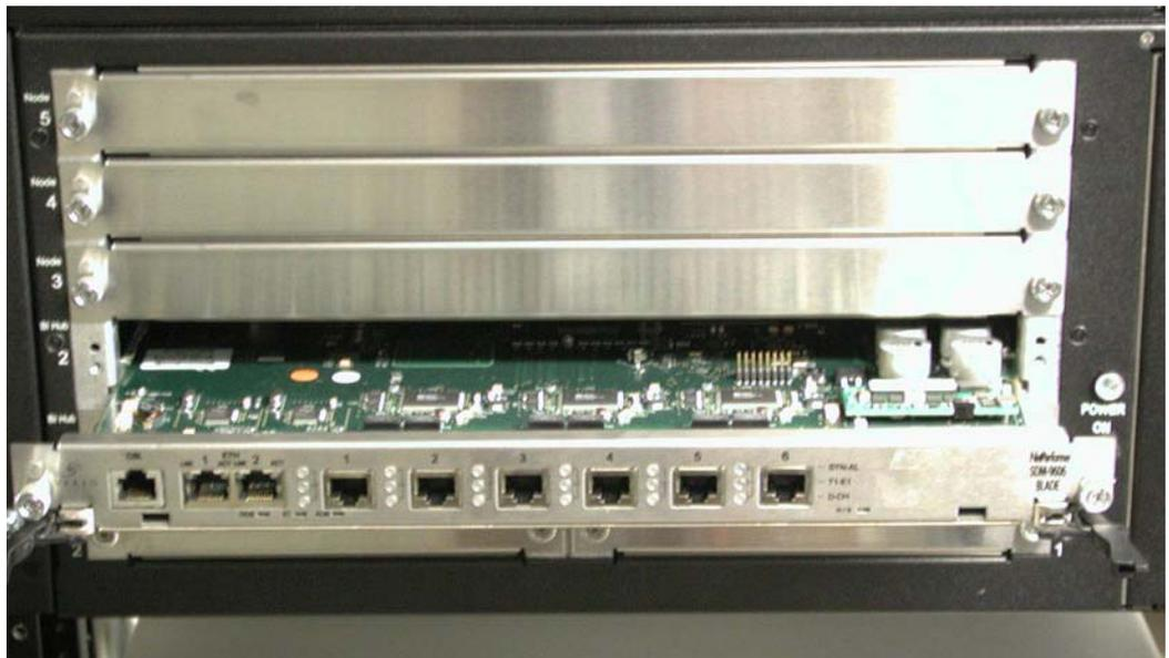
*Figure 3-5: Installing an SDM-9606 Blade in the SDM-9600 Chassis*
