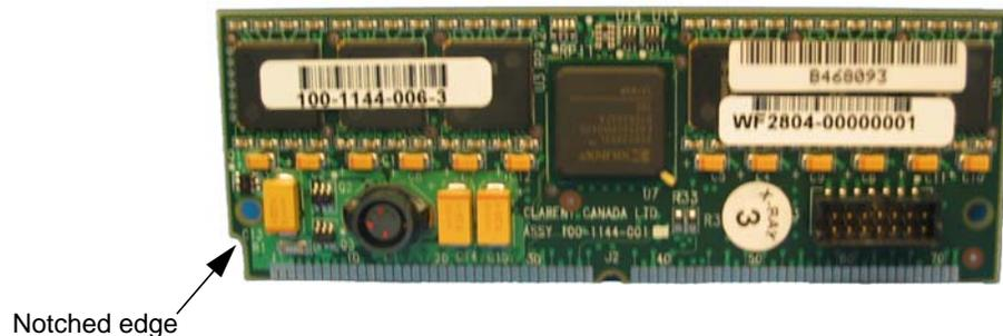
Figure 4-6: Synchronous High-density DSP Module
