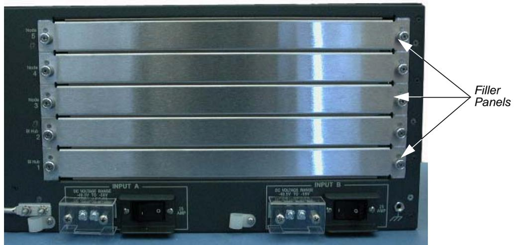
Figure 3-7: Rear View of the SDM-9600 Chassis with Filler Panels
