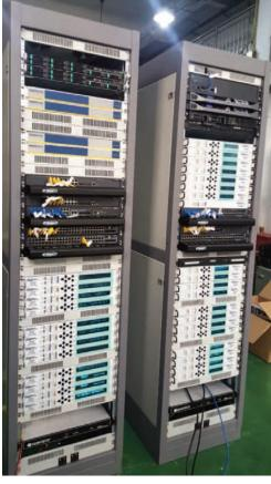
CDM-570A, CDM-625A and Memotec Equipment. Image is courtesy of Comtech EF Data
