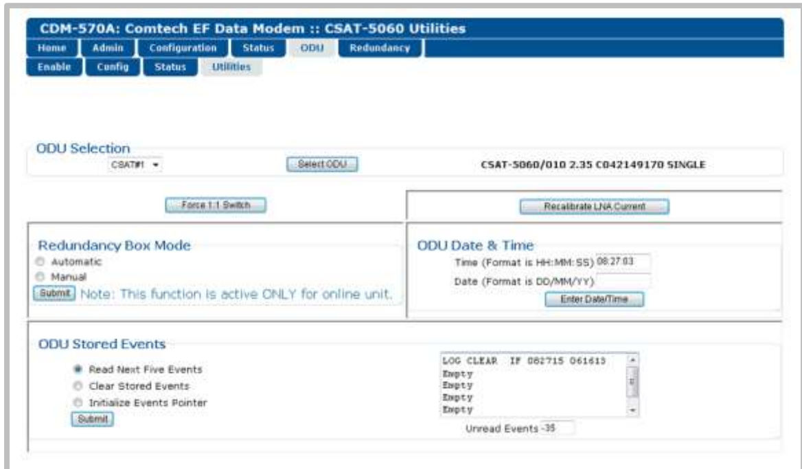
Figure 10-11. ODU | Utilities Page (CSAT-5060)
