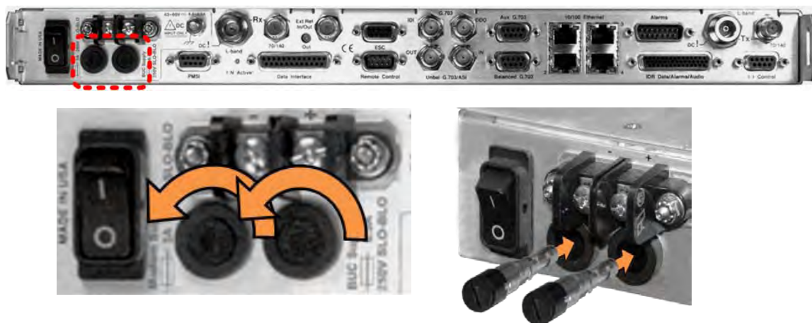
Figure 3-14. Replace the CDM-625A Optional DC Chassis Fuses
