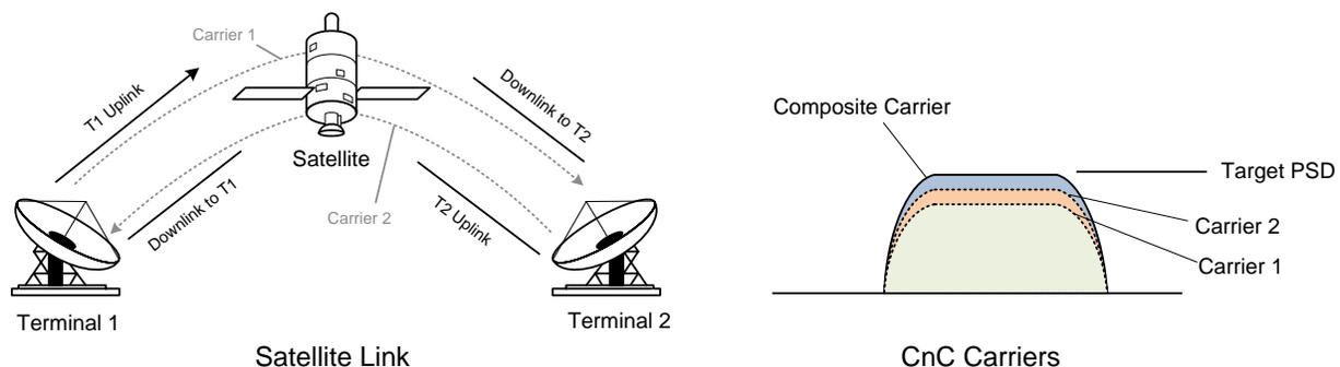
**Figure 1: Point-to-Point Carrier-in-Carrier Satellite Link**
