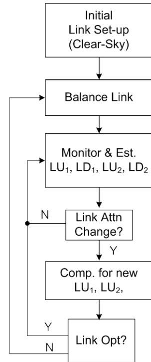
Figure 3: ACPC Logic Flow Diagram
