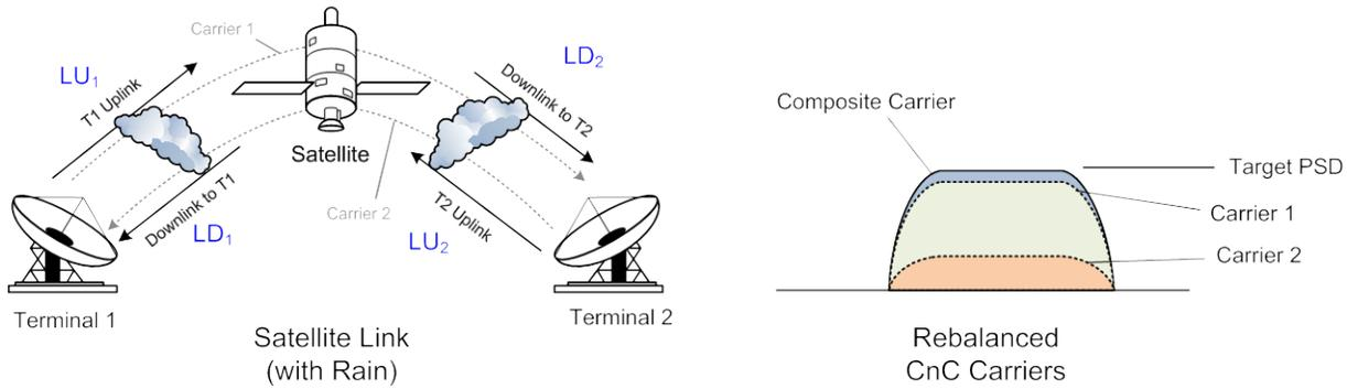
Figure 2: Point-to-Point Satellite Link with Rain
