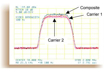
Figure 2 - Duplex Link with DoubleTalk Carrier-in-Carrier
