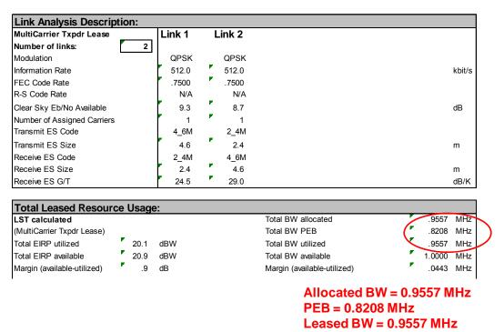
Carrier-in-Carrier link design involved trying different Modulation & FEC Code Rates to find the optimal combination:
