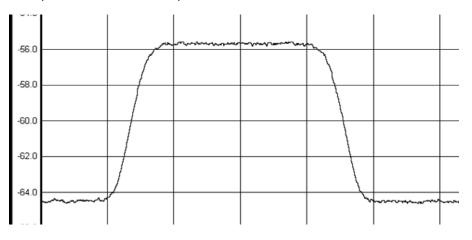
Figure 6: Test Link (With Carrier-in-Carrier) On a Spectrum Analyzer
