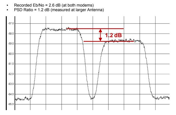
Figure 5: Test Link (Side-by-side) On A Spectrum Analyzer
