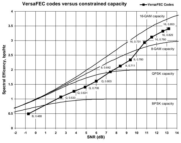
Figure 2. VersaFEC versus constrained capacity
