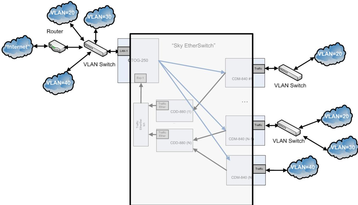
**Figure 1. Advanced VSAT Network with VLAN**
