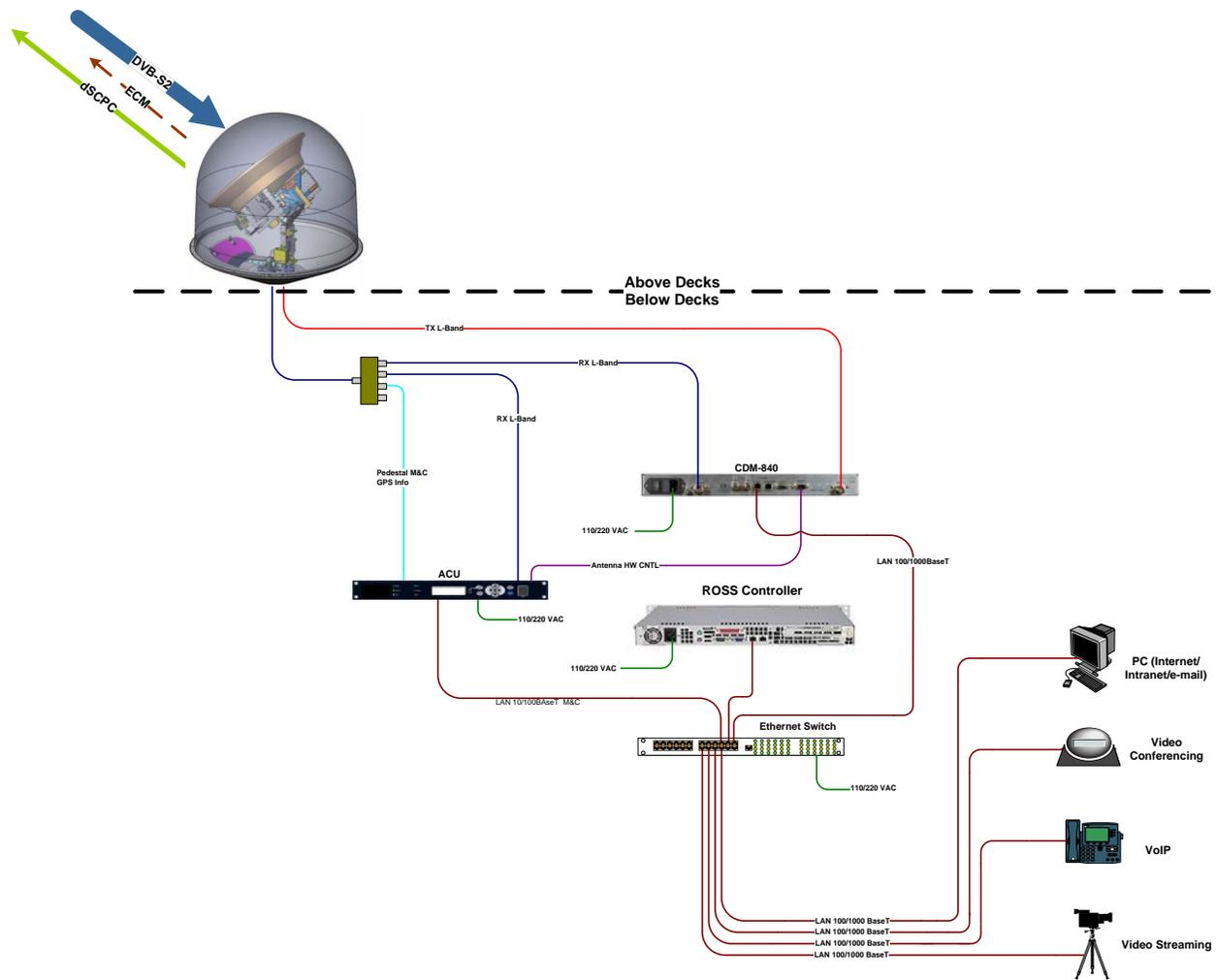
**Figure 5. Terminal Configuration**
