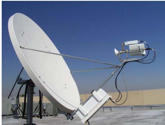
**Figure 6-1. KST-2000L System Installed on Spar Arm**
