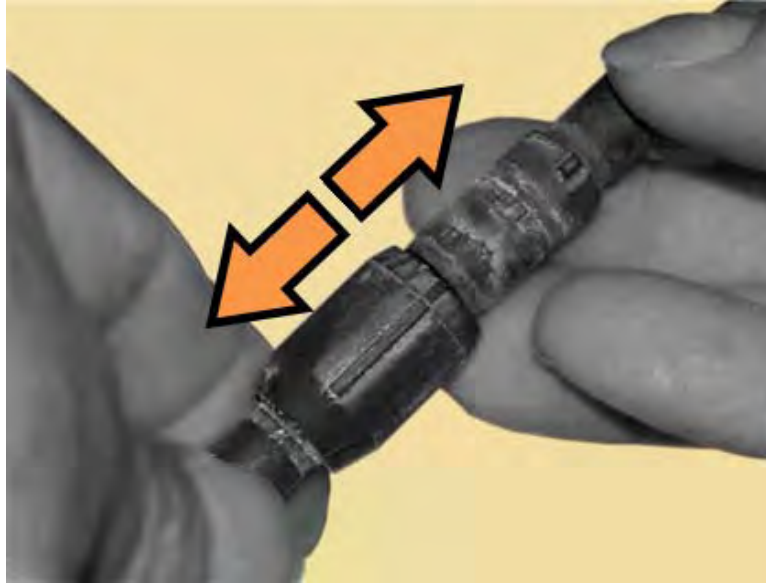
Figure C-15. Disconnect the Fan Power Supplies
