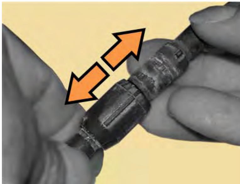
Figure C-10. Disconnect the Fan Power Supplies
