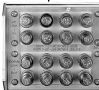
Figure 3-1. ICS-75 Front and Rear Panel Connectors (8-input configuration shown)
