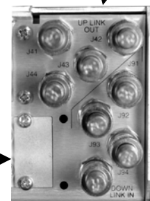
Figure 3-1. ICS-75 Front and Rear Panel Connectors (8-input configuration shown)
