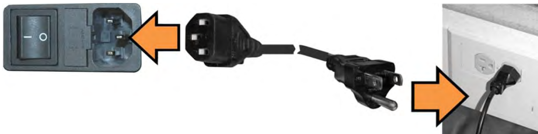
Figure 3-6. Apply AC Power to the Unit
