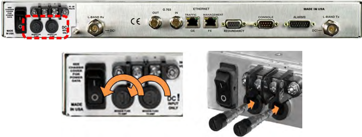
Figure 3-10. Replace the DC Fuses
