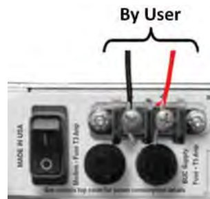
Figure 3-9. Apply DC Power to the Unit
