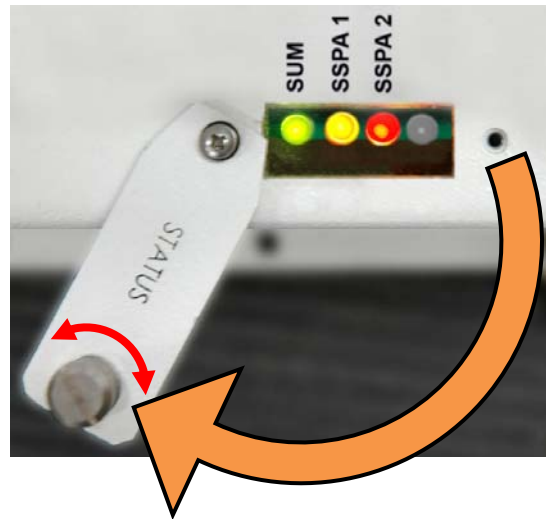
Figure 3-4. PCCB LED Display Window
