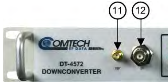
Figure 4-14. Front Panel Sample Test Point Connections
