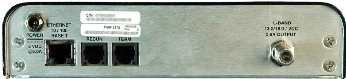
Figure 3-1. Digicast Media Router S2 Receiver – Rear Panel
