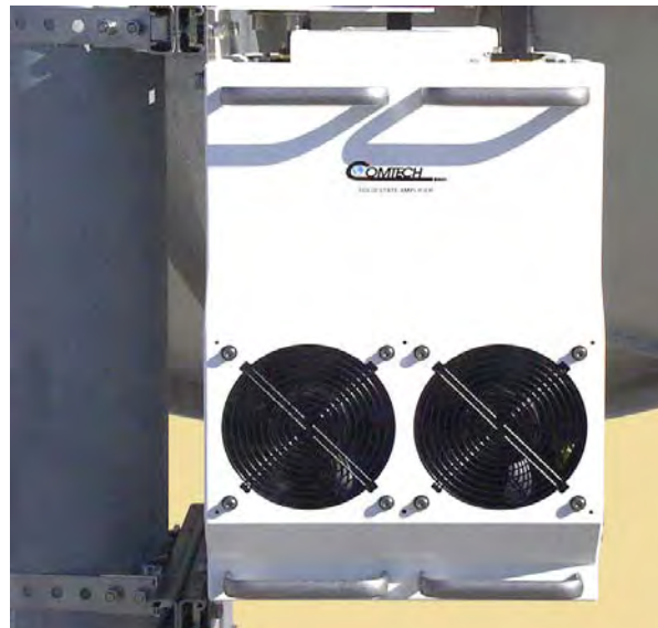
Figure 5-11. Installed CSAT (100W/125W Unit Shown, Side view)
