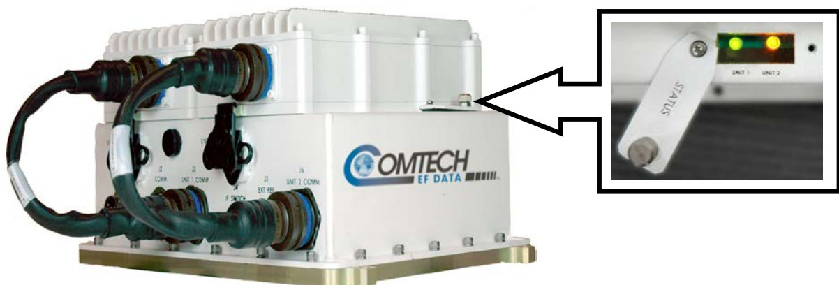
Figure 4-1. MBT-4000 Multi-Band RF Transceiver LED Indicators
