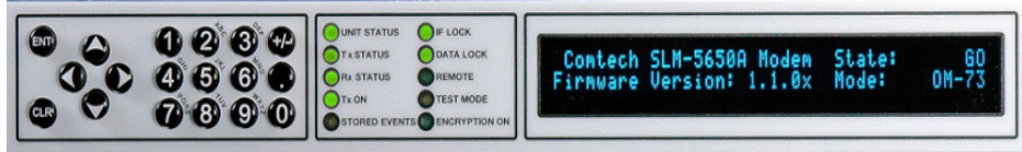
Figure 2-3 Front Panel, SLM-5650A Modem
