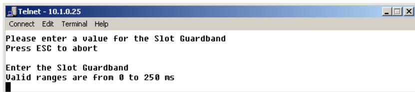
**Figure 3-16** Slot Guardband prompt
