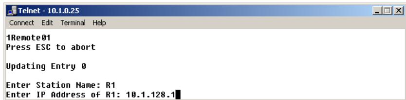
**Figure 3-21** Adding a Remote to the STDMA group
