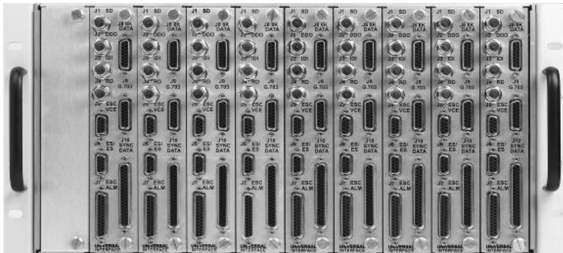
Figure 5-7 DDS20 Universal Switch – Front Panel Data Switch Modules
