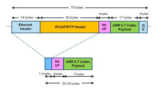
Our second generation **Payload Compression** processor is implemented directly in the hardware for increased performance and efficiency. This allows any payload compression with very low jitter and delay, which is particularly critical for 2G/3G traffic to maintain good KPI for voice and data services performance.
