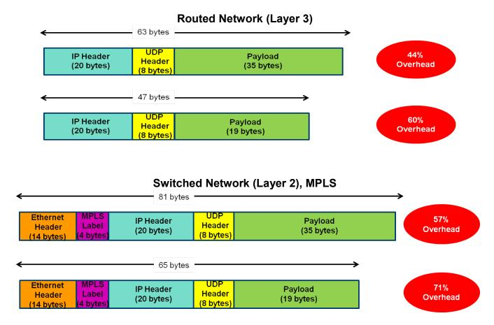
The same considerations apply to 3G IP BTS for voice traffic (at the lub interface) and parts of the data traffic, e.g. TCP ACK packets when the user browses the web or downloads files, which represents most of the mobile data traffic.
