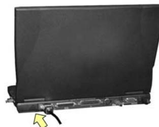
2. Connect the adapter cable circular connector to the mating remote M&C port on the RF unit.
