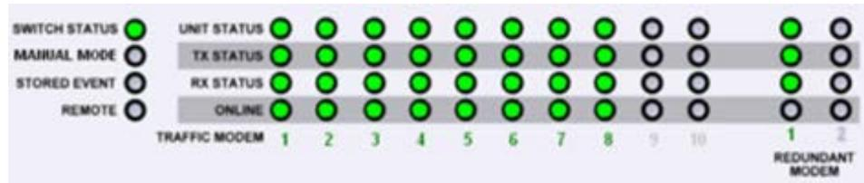
**Figure 8-3. CRS-500 CSU Front Panel – LED Groups**
