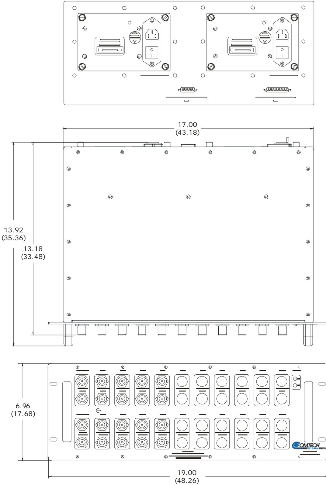
**Figure 2-4. CRS-280L (L-Band) IF Switch (Standard AC Unit Shown)**
