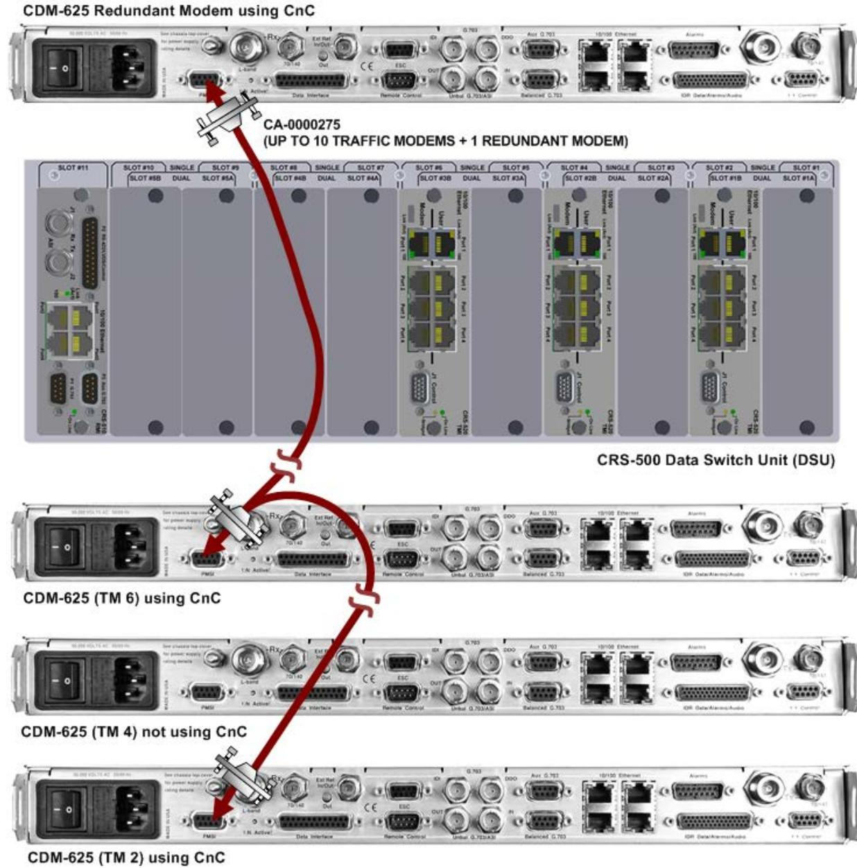
**Figure 5-7. CDM-625/625A → CDM-625/625A CnC® Cable Connection Example
