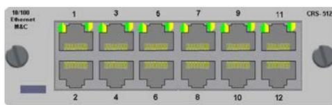
Figure 1-4. CRS-512 Ethernet M&C Module (Feature 2A)
