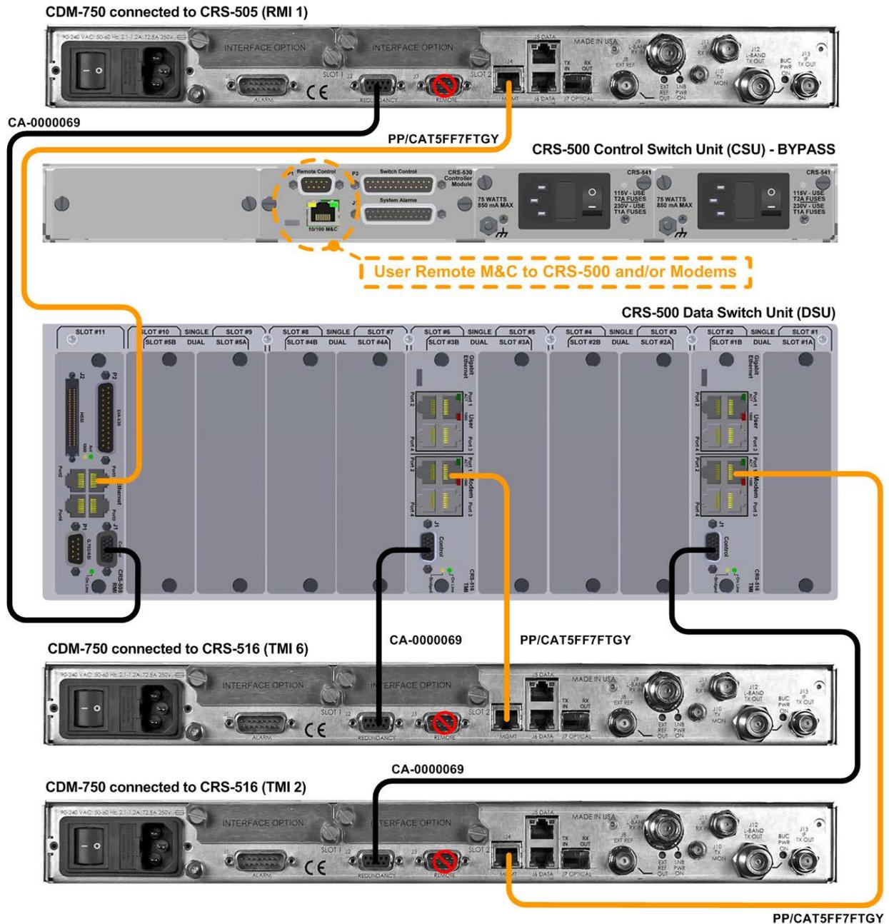
Figure 5-8. CRS-500 → CDM-750/760 Control & Ethernet System Comm Cabling Example – 10/100/1000 GbE Traffic Data (1:N connections shown for TMIs 2 and 6 only)
