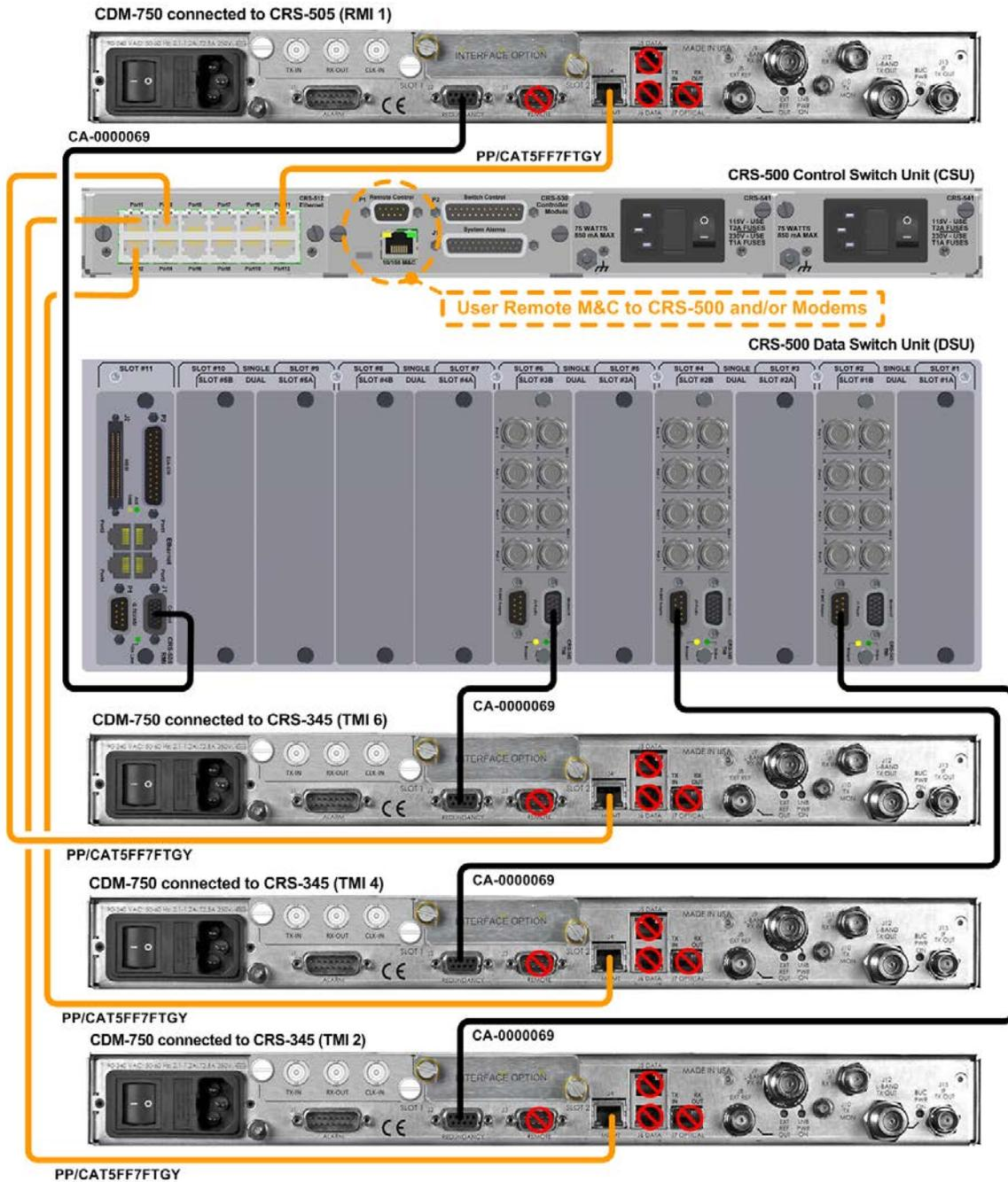
**Figure 5-9. CRS-500 → CDM-750/760 Control & Ethernet System Comm Cabling Example – Unbalanced G.703 Traffic Data (1:N connections shown for TMs 2, 4, and 6 only)**
