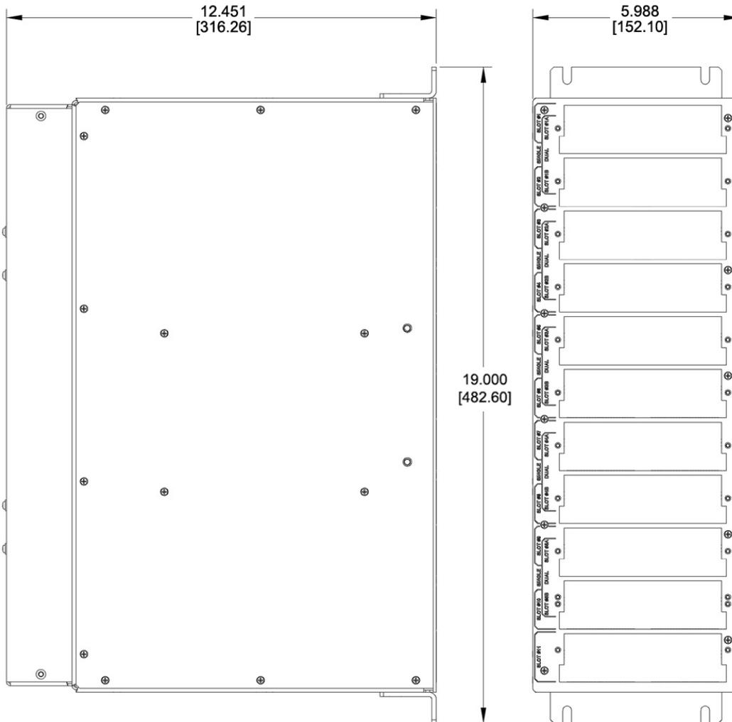
Figure 2-2. CRS-500 DSU Dimensional Envelope
