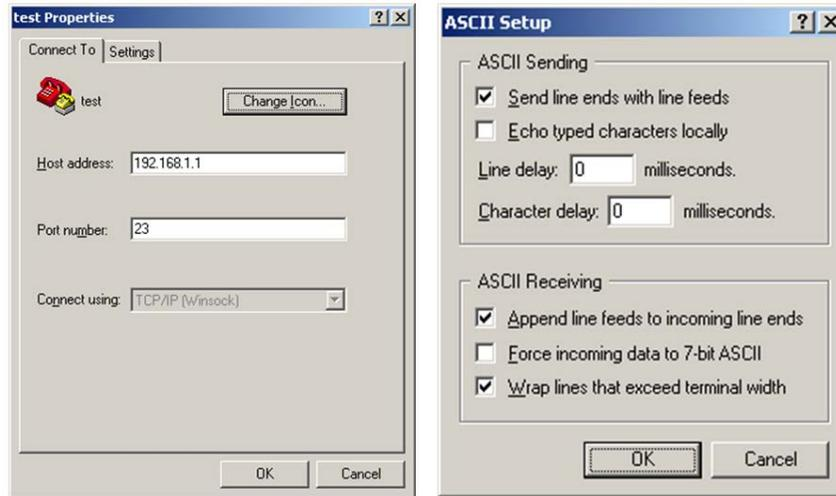
**Figure 9-3. Configure HyperTerminal**
