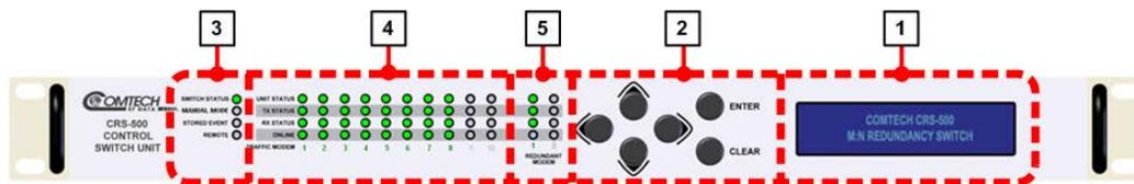
Figure 8-1. CRS-500 CSU Front Panel – M&C Features
