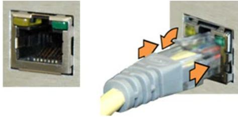
**Figure B-3. RJ-45/RJ-48 Connector Example**
