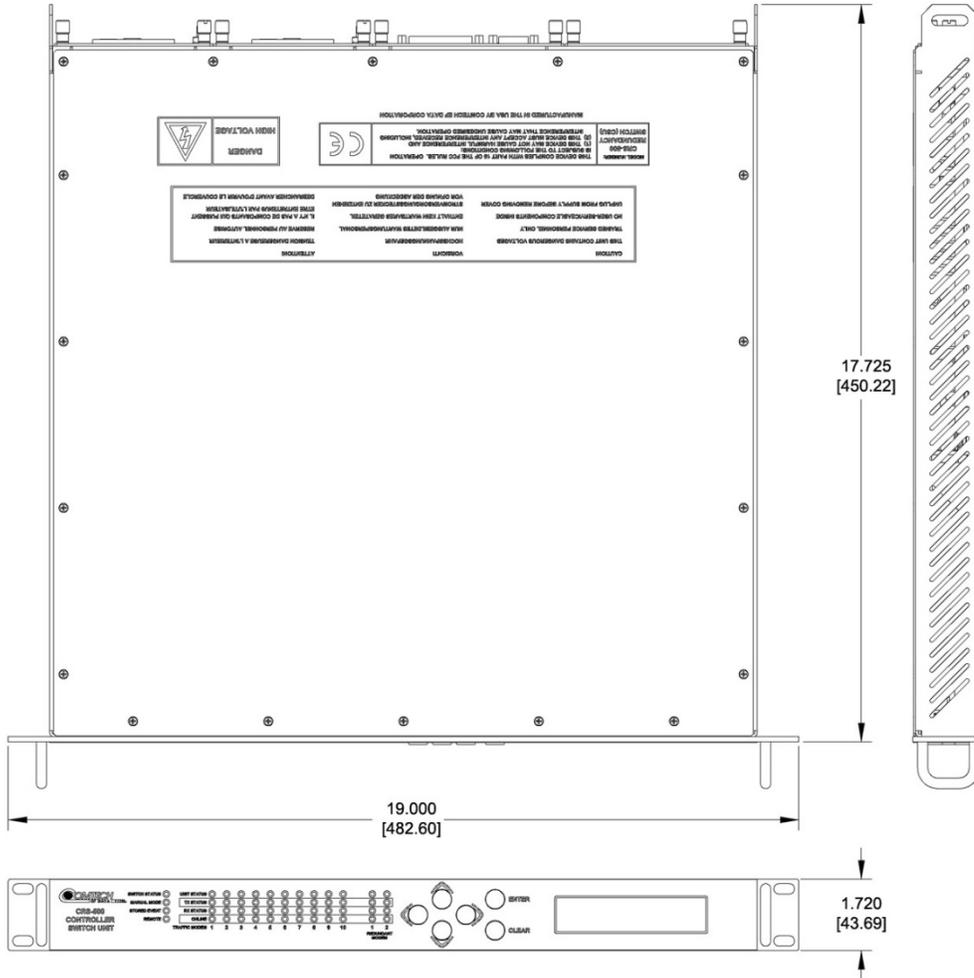
Figure 2-1. CRS-500 CSU Dimensional Envelope
