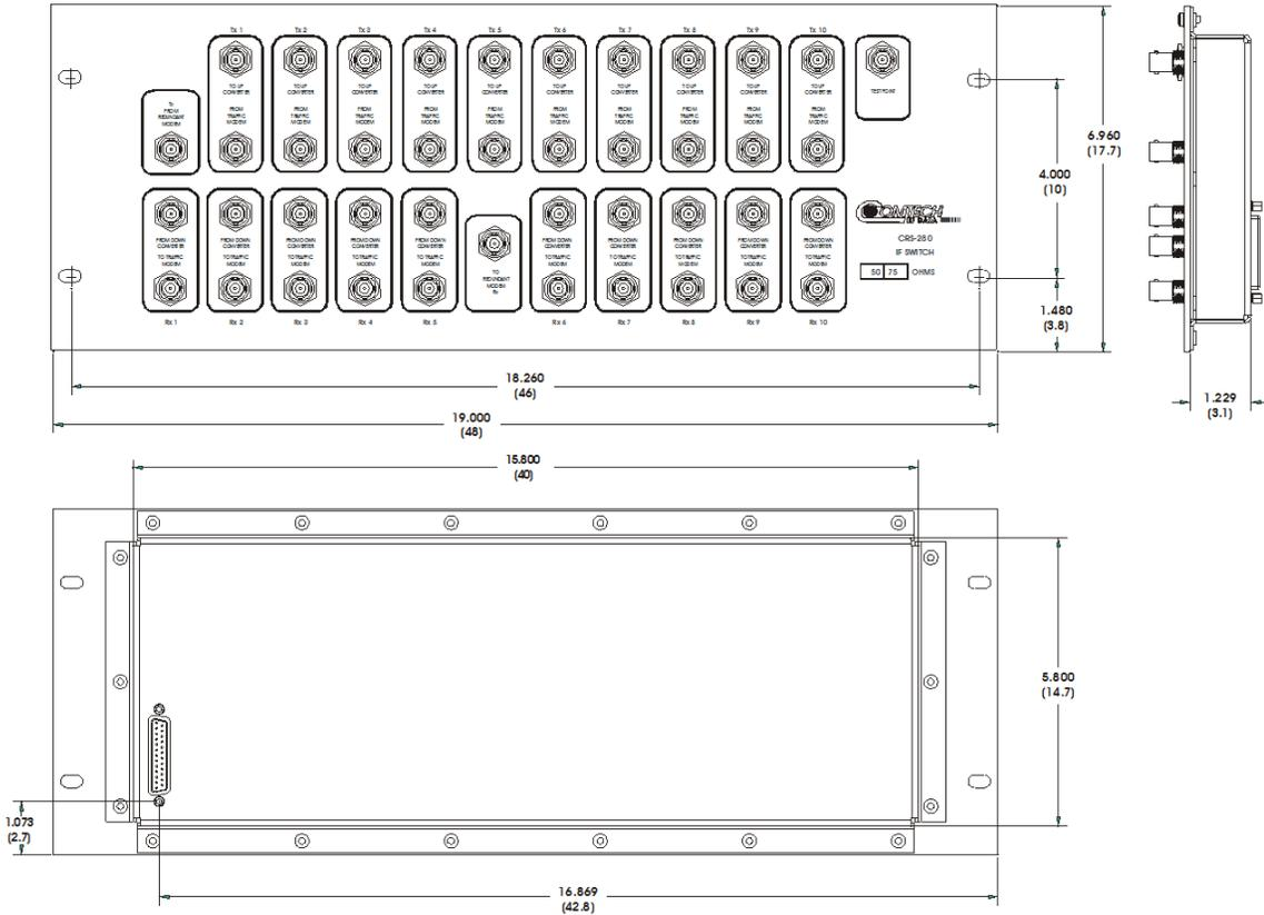
Figure 2-3. CRS-280 (70/140MHz) IF Switch
