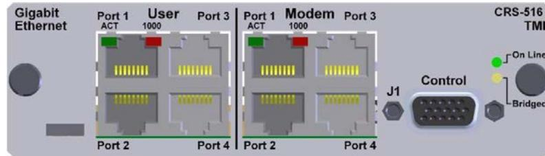
The CRS-516 TMI provides four standard RJ-45F User Interface ports, operating at 10/100/1000 Mbps, full and half duplex, auto-negotiating for Base-T Gigabit Ethernet (GbE).
