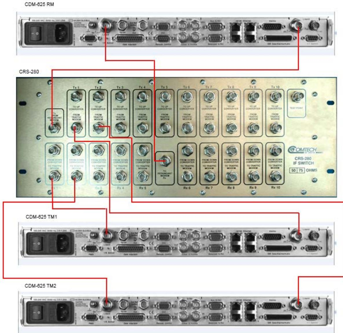
**Figure 5-13. CRS-500 1:N IF Cabling Example 2 – CRS-280 → CDM-625/A**
