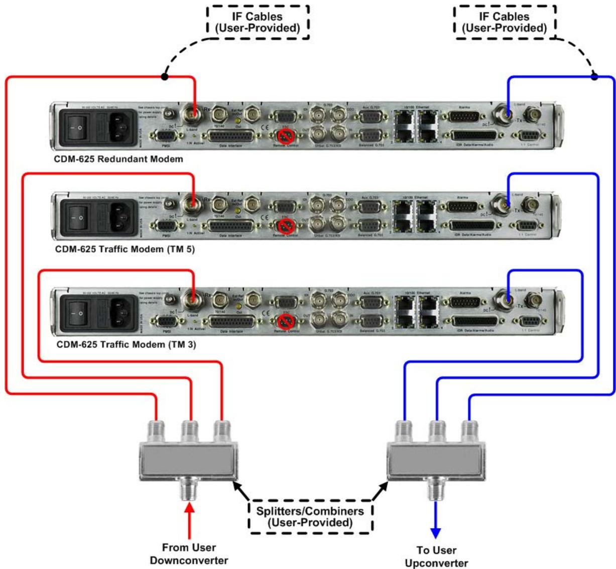
**Figure 5-12. CRS-500 1:N IF Cabling Example 1 – Single Transponder Configuration (No ISU) (Connections shown for TMs 3 and 5 and 8 only)**
