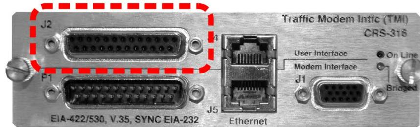
This 25-pin Type 'D' female connector provides the **EIA-232/422/V.35** User Data Interface on the CRS-316 TMI.
