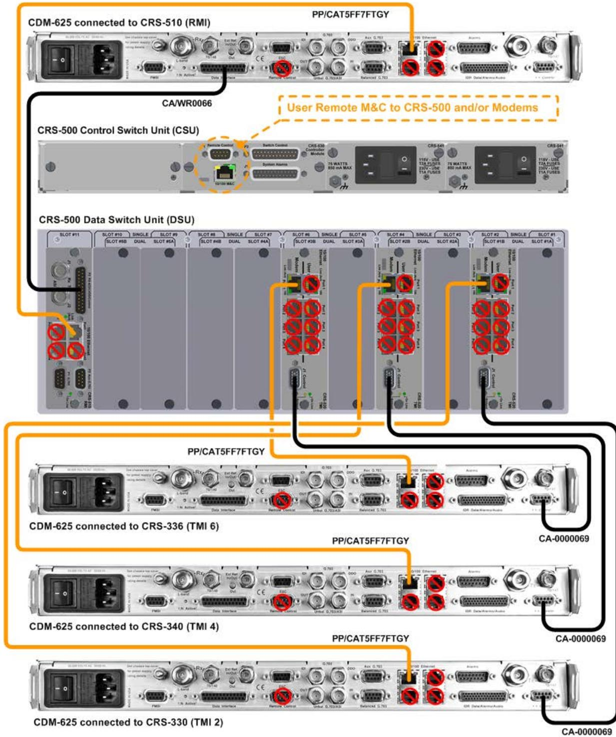
**Figure 5-4. CRS-500 → CDM-625/625A Control & Ethernet System Comm Cabling Example (1:N connections shown for TMIs 2, 4, and 6 only)**
