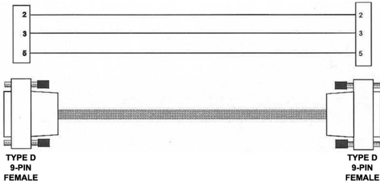
Figure A-1. Switch M&C / Firmware Update Cable
