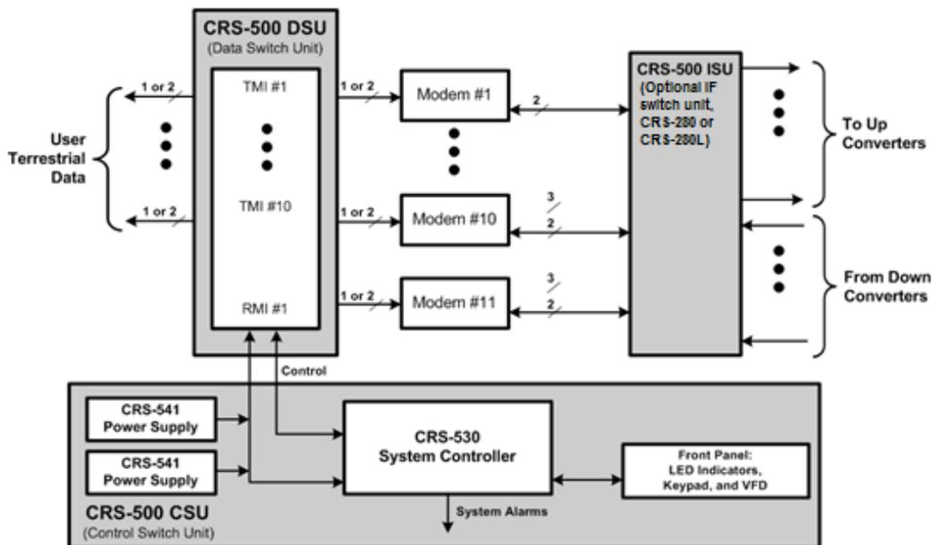
Figure 1-2. Typical CRS-500 Redundancy System – System-Level Block Diagram
