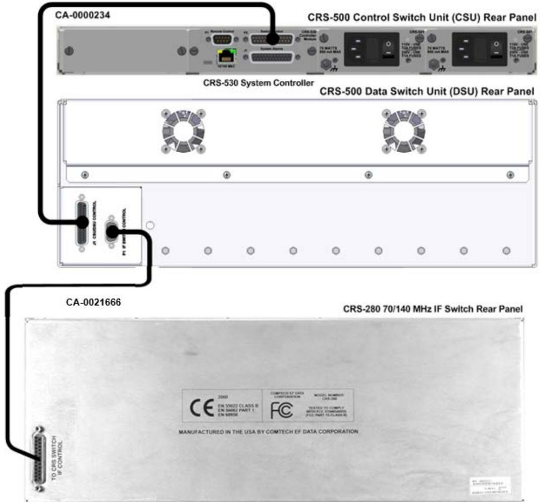
Figure 5-1. Control Cable Connection for CRS-500 to CRS-280 Example
