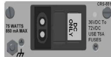
Figure 1-7. Optional CRS-551 DC Power Supply (Feature 2D)
