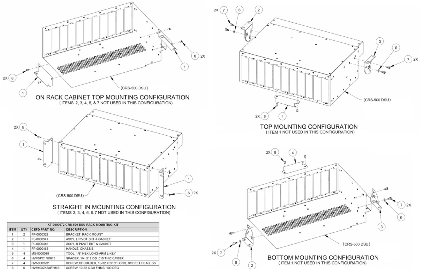
Figure 4-4. CRS-500 Optional DSU Rack Mounting Kit KT-0000072
