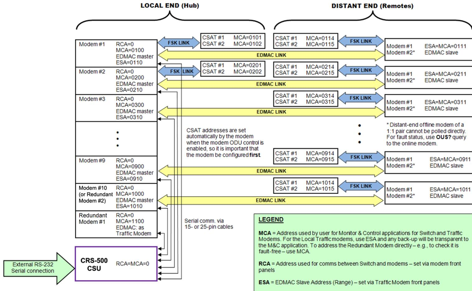
Figure C-1. External EIA-232 with CDM-625/A Modems
