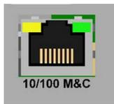
The “**10/100 M&C**” connector is an RJ-45F connector that serves as an Ethernet 10/100 user interface.
