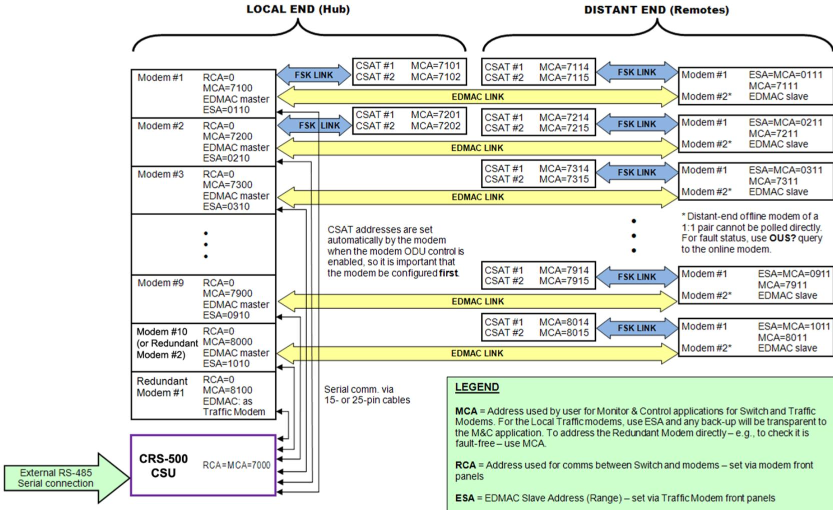
Figure C-2. External EIA-485 with CDM-625/A Modems
