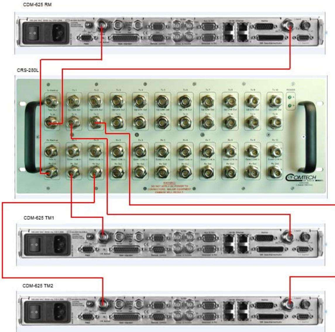
**Figure 5-14. CRS-500 1:N IF Cabling Example 3 – CRS-280L → CDM-625/A
