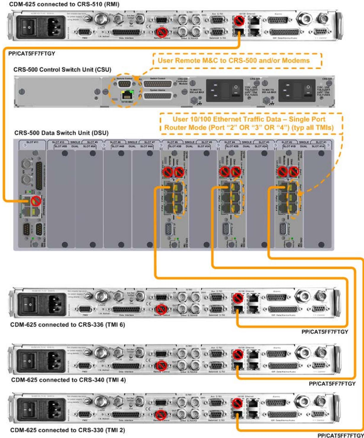
**Figure 5-5. CRS-500 → CDM-625/625A 10/100 Ethernet Traffic Data Cabling Example (Single Port Router Mode, 1:N connections shown for TMs 2, 4, and 6 only)**
