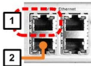
**Figure 5-3. CDM-625/625A 10/100 Ethernet Ports**
