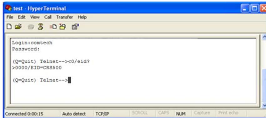
**Figure 9-2. Telnet Interface Example – HyperTerminal**
