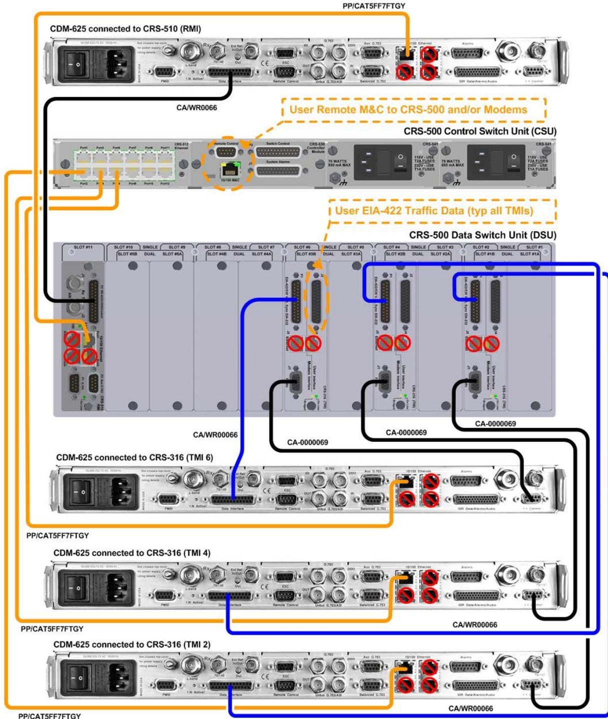
**Figure 5-6. CRS-500 → CDM-625/625A EIA-422 Traffic Data Cabling Example (1:N connections shown for TMs 2, 4, and 6 only)**
