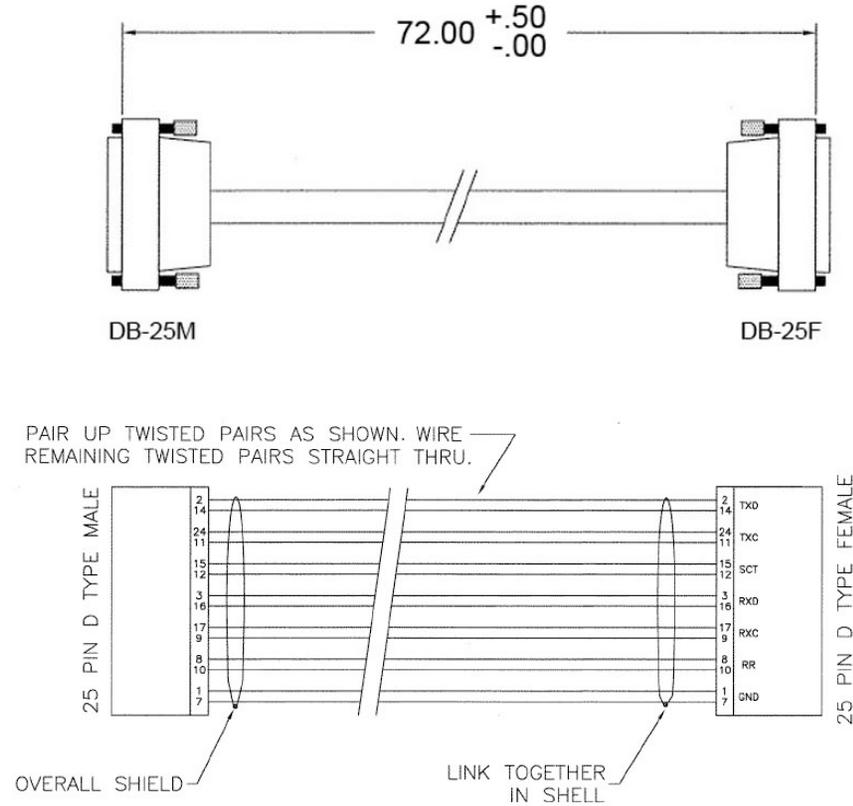
Figure A-4. RMI Control Cable (CEFD P/N CA/WR0066)
