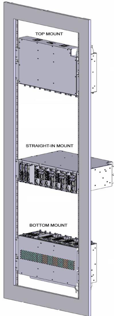
**Figure 4-3. CRS-500 DSU In-Rack Mounting Examples
