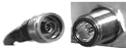
Type 'N' connectors feature a Threaded Coupling design similar to Type 'TNC', Type 'F', and Type 'SMA' connectors.
