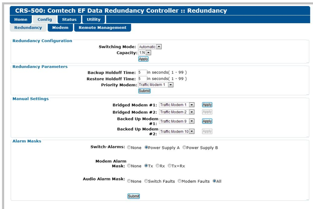
Figure 9-5. 'Config | Redundancy' Page
