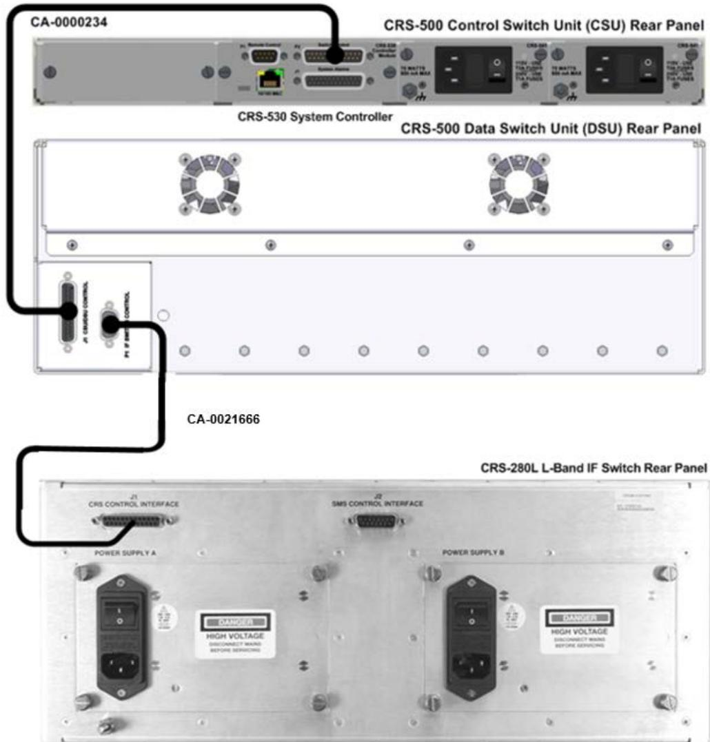
Figure 5-2. Control Cable Connection for CRS-500 to CRS-280L Example
