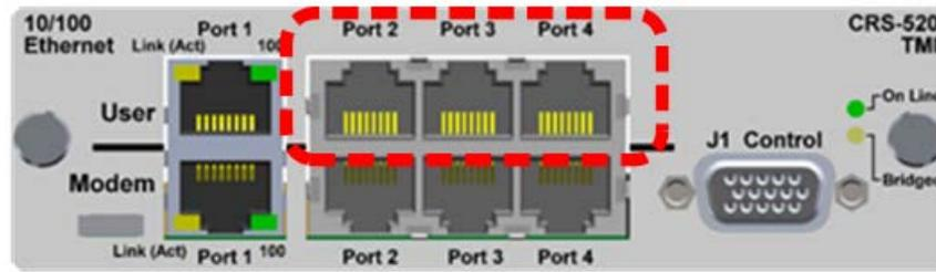
The CRS-520 TMI provides four standard RJ-45F User Interface ports, operating at 10/100 Mbps, half and full duplex, auto-negotiating for Ethernet Router Modes.
