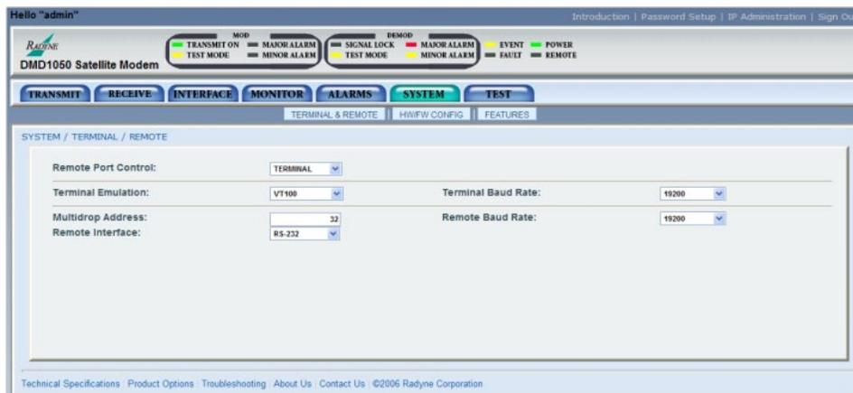
Figure 7-31 System / Terminal & Remote page example
