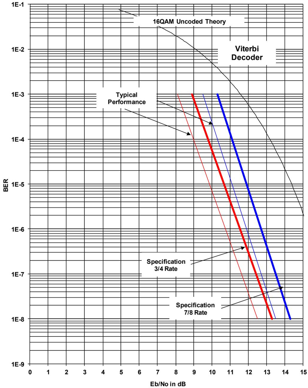
Figure 7-7. DMD2050E 16QAM BER Performance (Viterbi)
