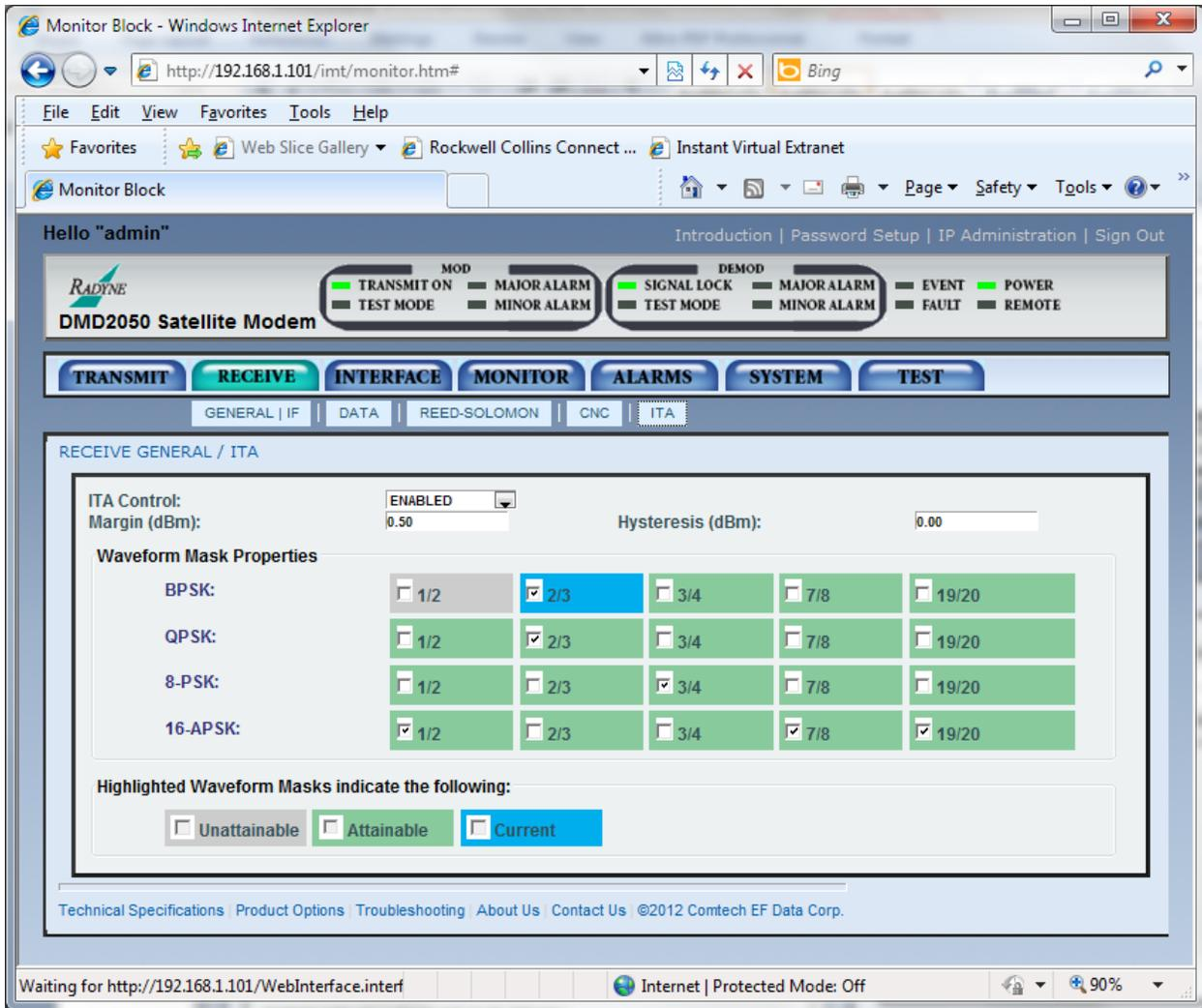
Figure J-10 - Initial Setup DMD2050E, Demodulator ITA (Enabled)
