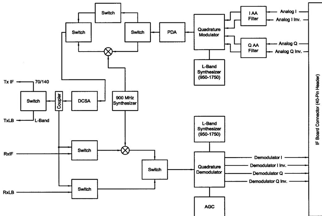
Figure 3-2. IF Card Block Diagram
