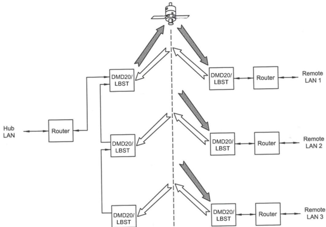
Figure H-1. Point-to-Multipoint with Daisy Chaining
