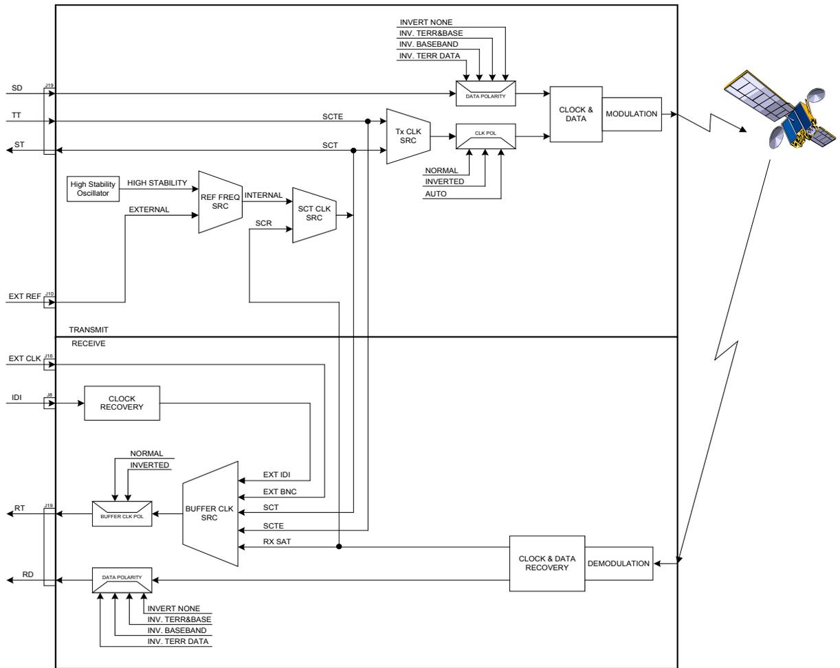
Figure 3-8. Clocking and Polarity Diagram
