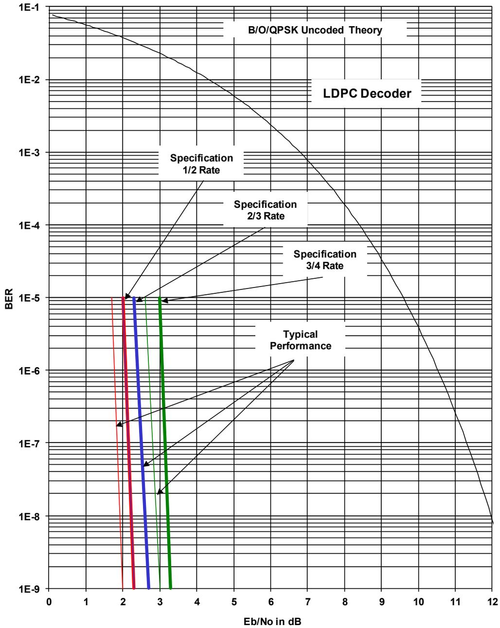
Figure 7-14. DMD2050E B/O/QPSK BER Performance (LDPC)
