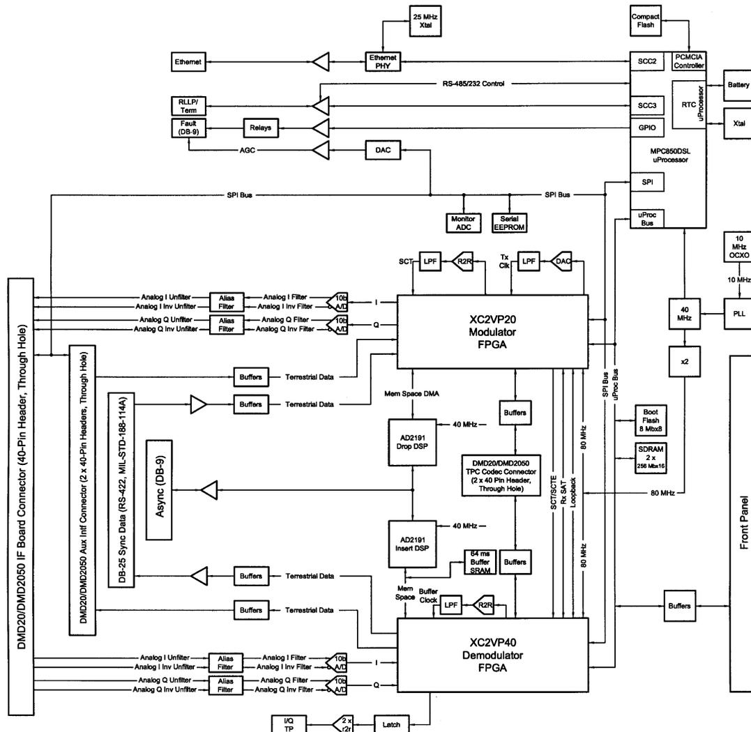
Figure 3-3. DMD2050E Baseband Processing Card Block Diagram
