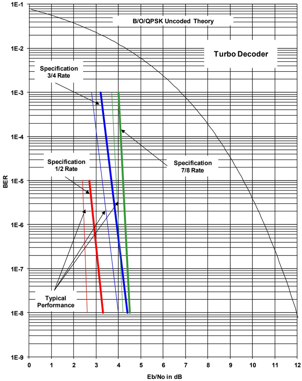
Figure 7-10. DMD2050E OQPSK BER Performance (Turbo)
