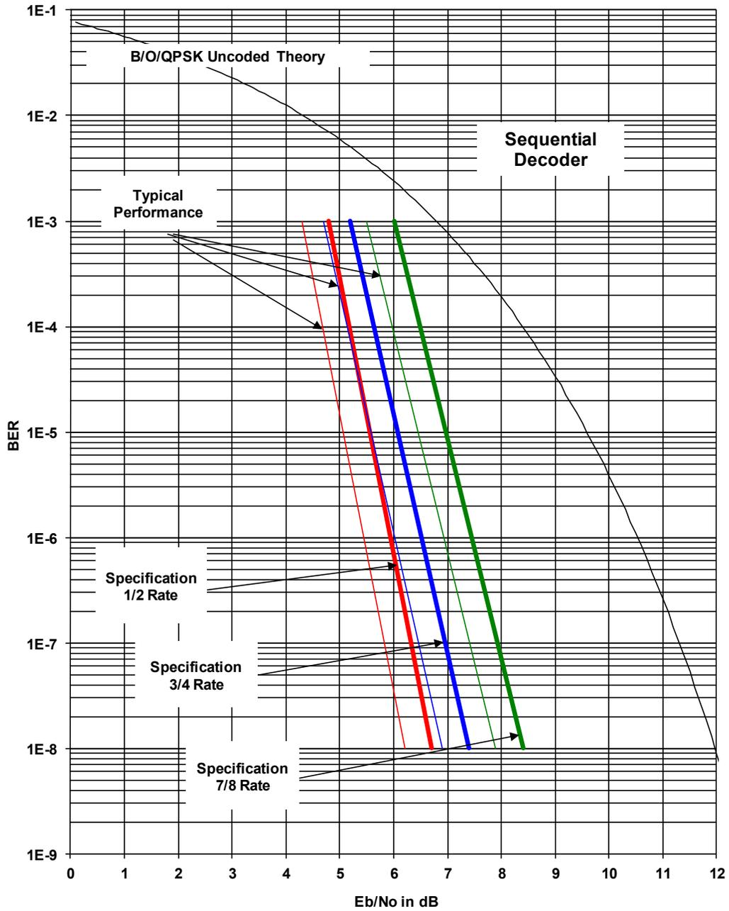
Figure 7-2. DMD2050E B/O/QPSK BER Performance (Sequential)
