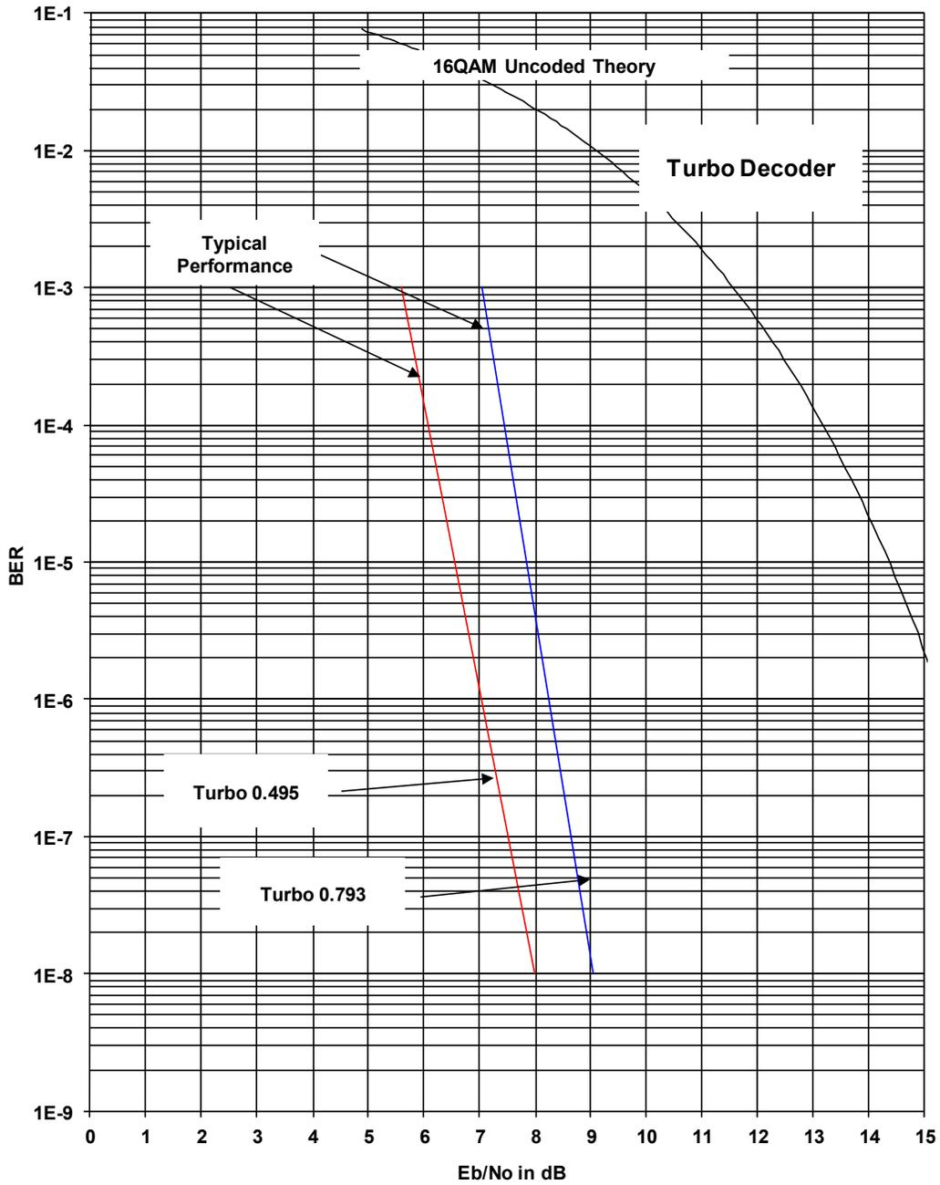
Figure 7-9. DMD2050E 16QAM BER Performance (Turbo)
