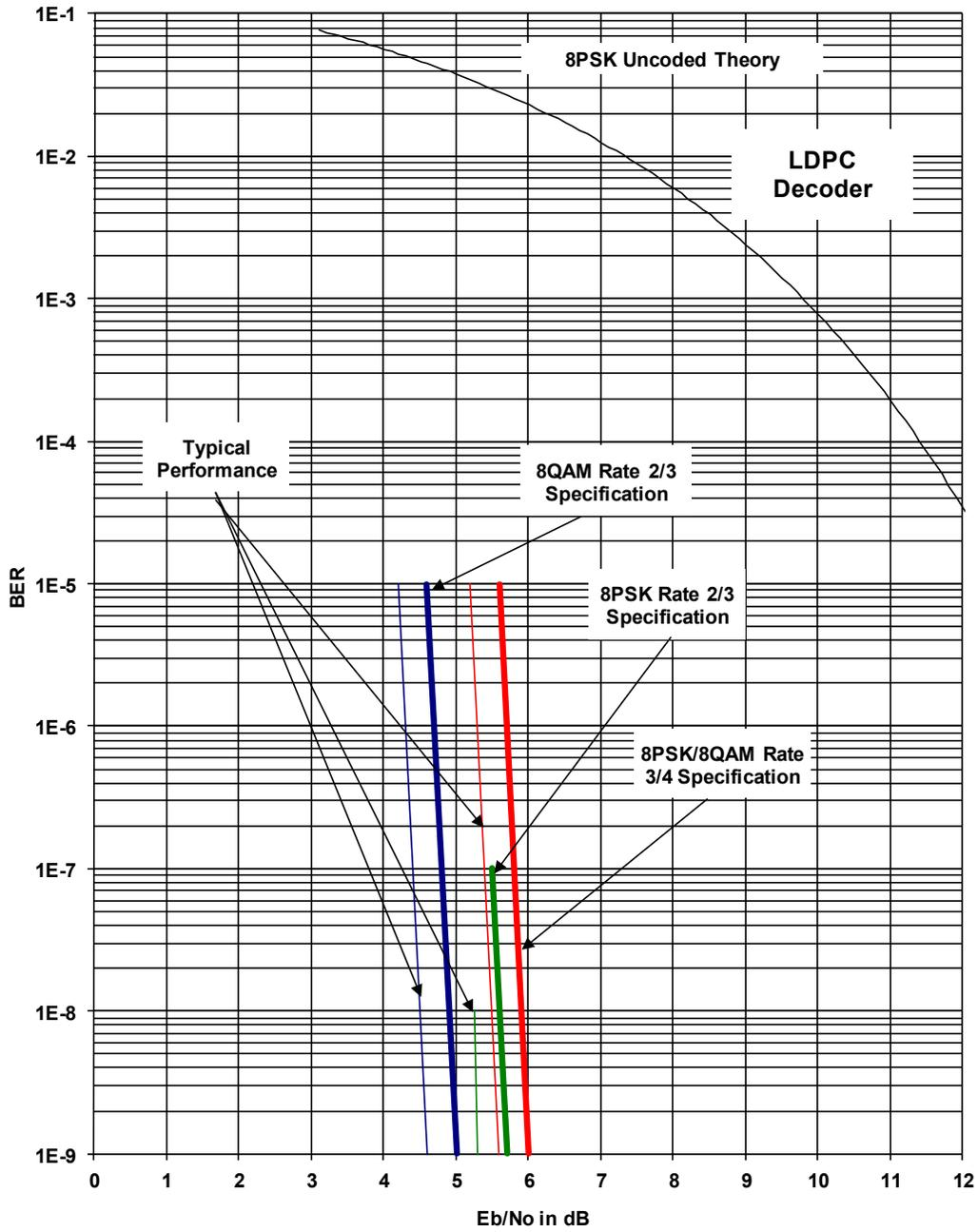
Figure 7-15. DMD2050E 8PSK / 8QAM BER Performance (LDPC)
