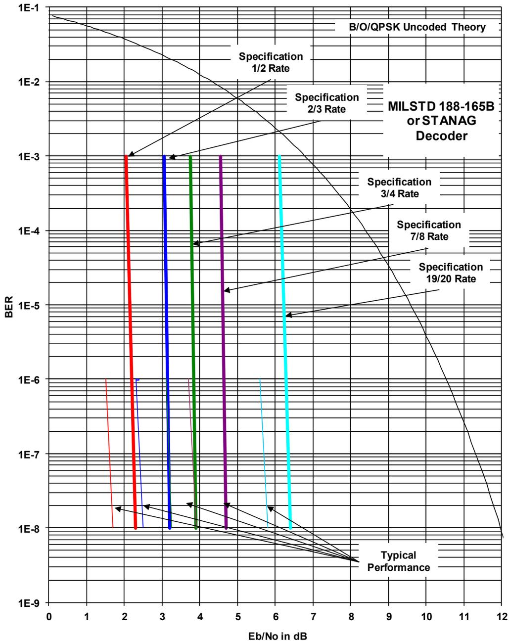
Figure 7-17. DMD2050E BER Performance B/O/QPSK (MILSTD 188-165B or STANAG) Turbo
