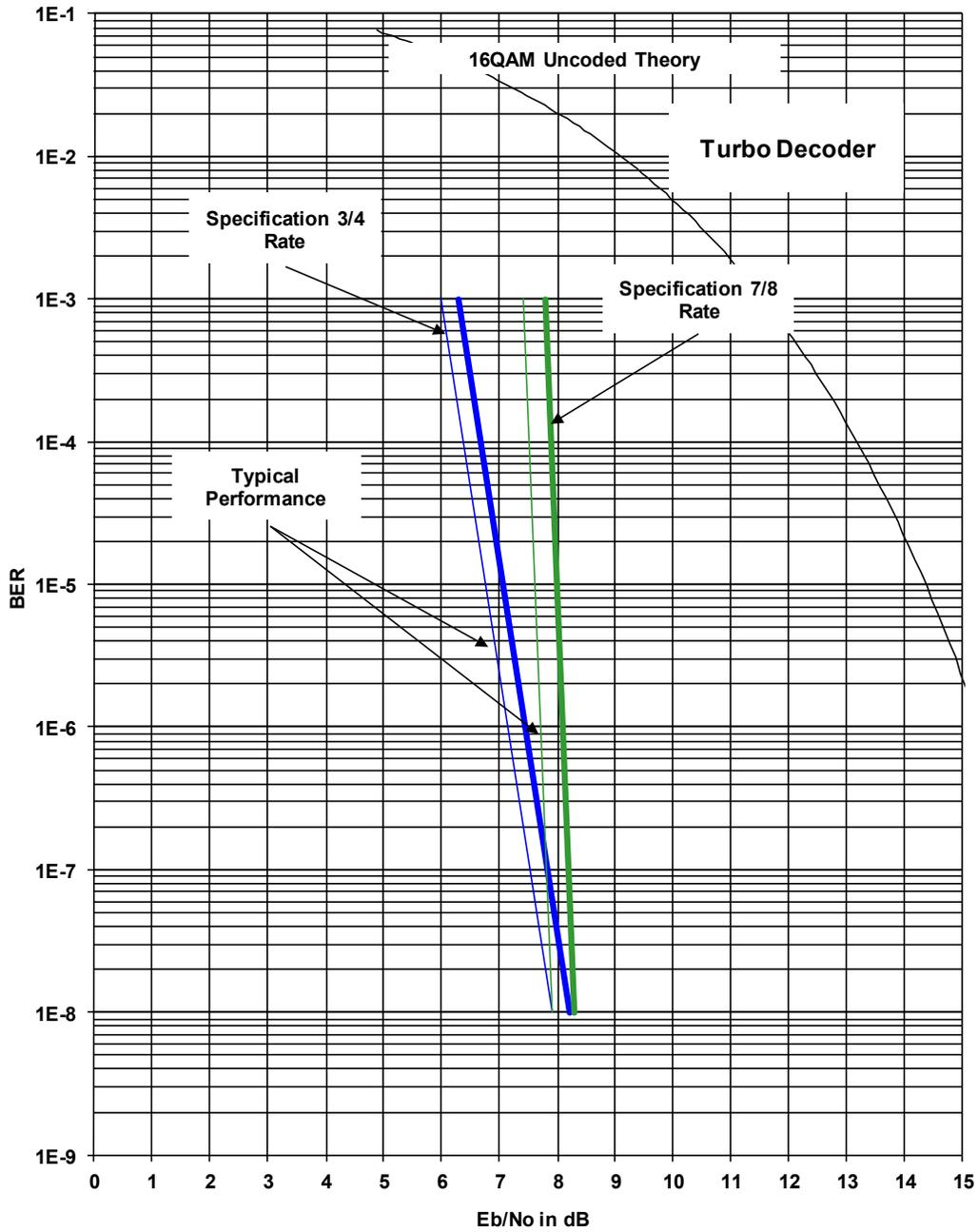
Figure 7-13. DMD2050E 16QAM BER Performance (Turbo)
