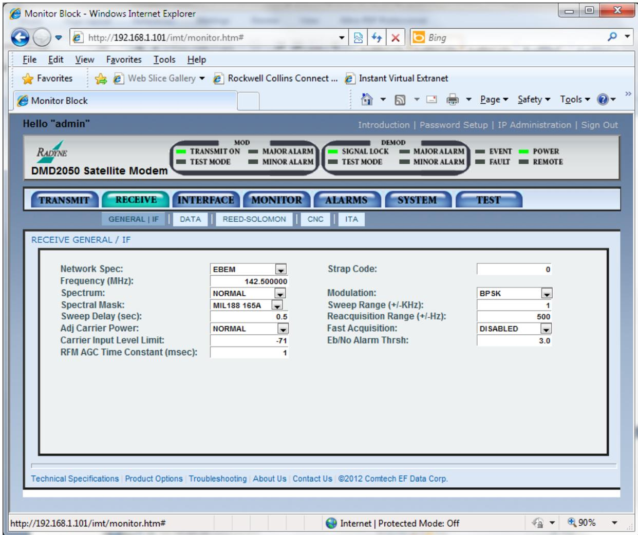
Figure J-4 - Initial Setup DMD2050E, Demodulator IF
