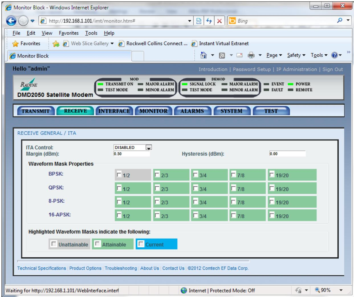
Figure J-6 - Initial Setup DMD2050E, Demodulator ITA
