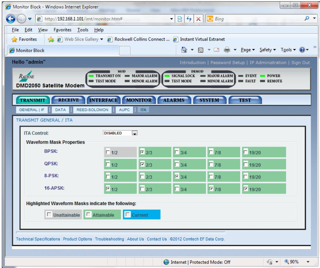
Figure J-7 - Initial Setup DMD2050E, Modulator ITA
