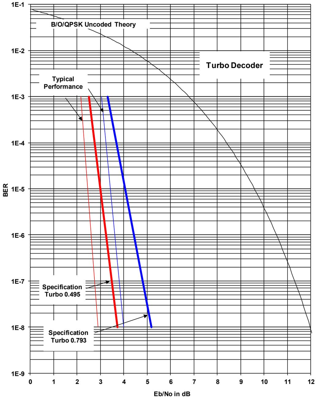
Figure 7-4. DMD2050E B/O/QPSK BER Performance (Turbo)
