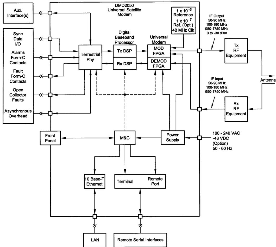
Figure 3-4. DMD2050E Universal Satellite Modem Functional Block Diagram
