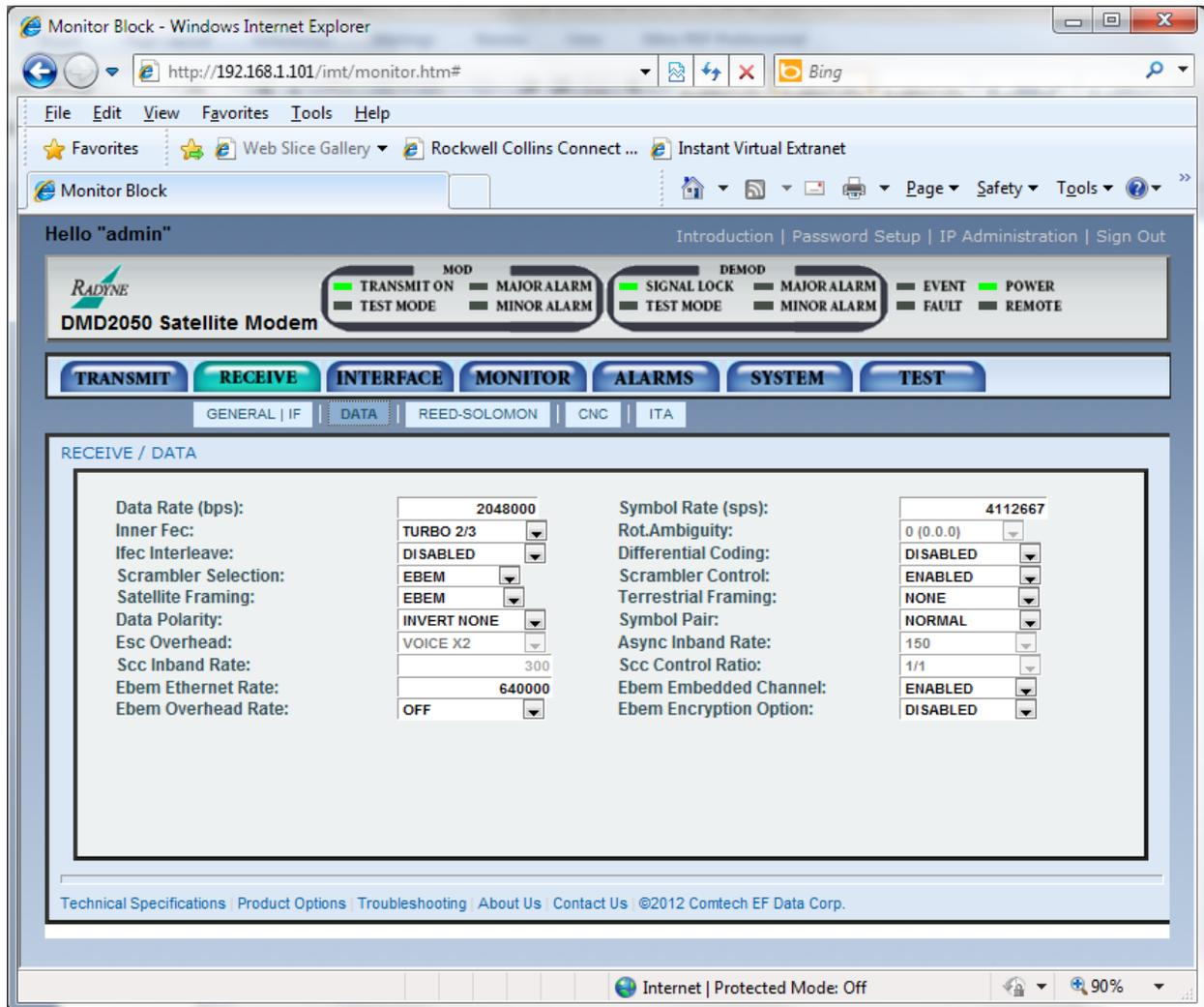
Figure J-5 - Initial Setup DMD2050E, Demodulator Data
