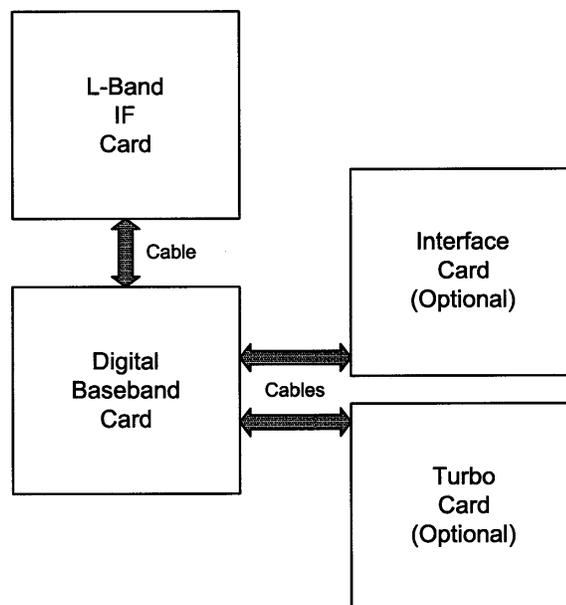
Figure 3-1. DMD2050E Block Diagram
