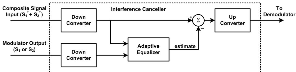
Figure 3-18. Carrier-in-Carrier Signal Processing Block Diagram
