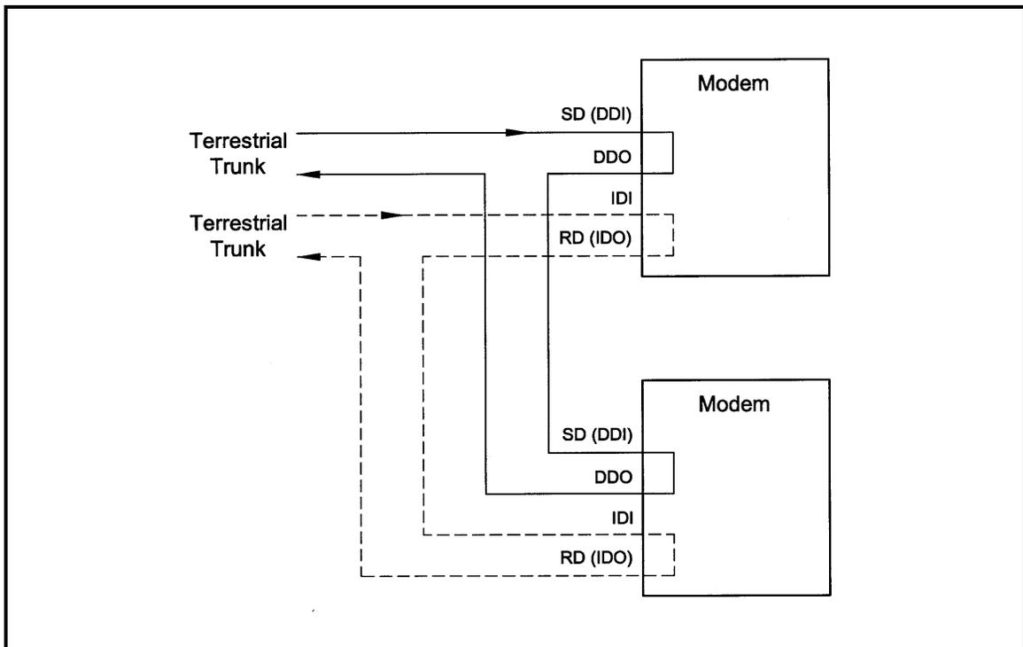
Figure E-2 Looped Modems with Separate D&I Trunks
