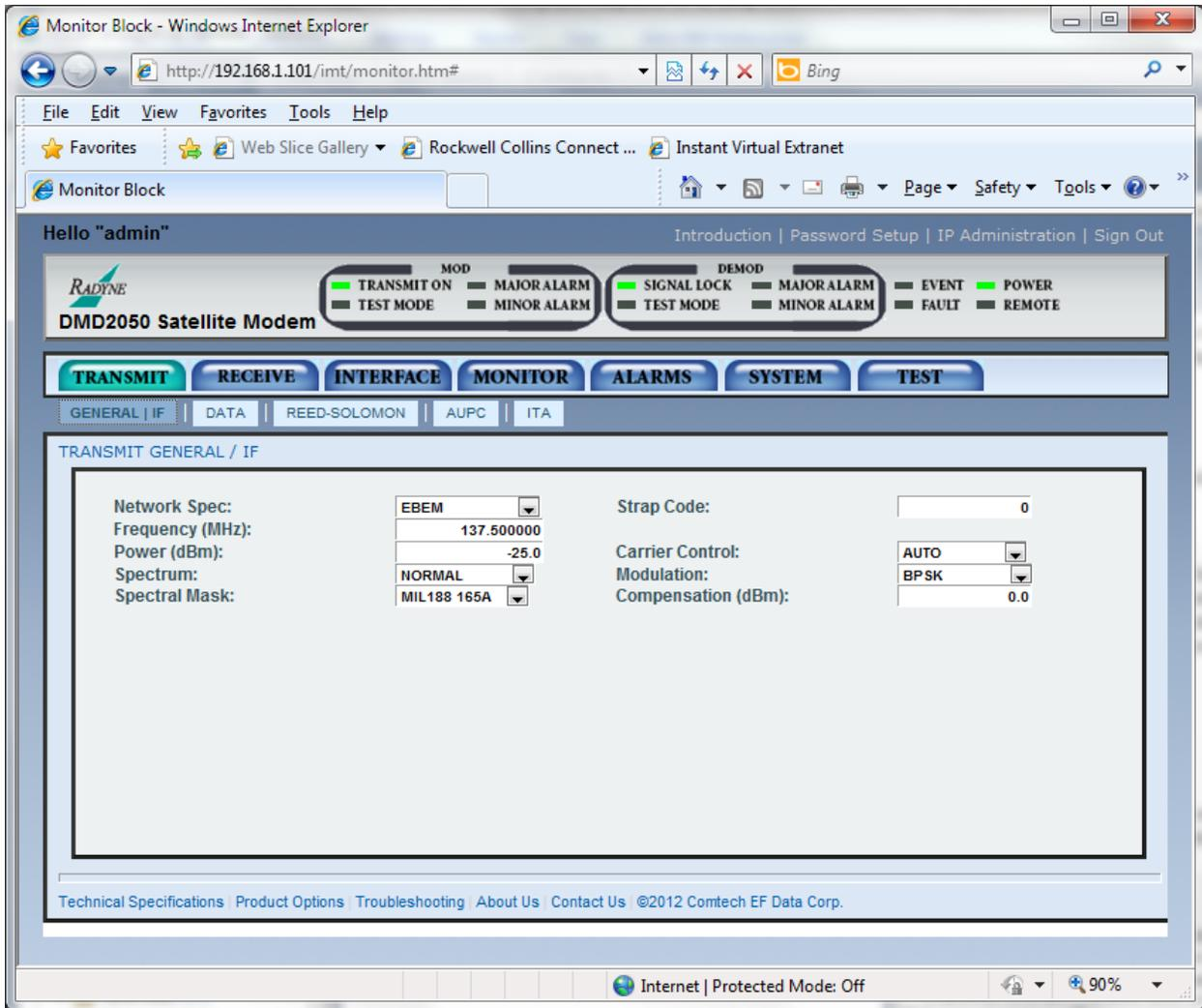
Figure J-1 - Initial Setup DMD2050E, Modulator IF
