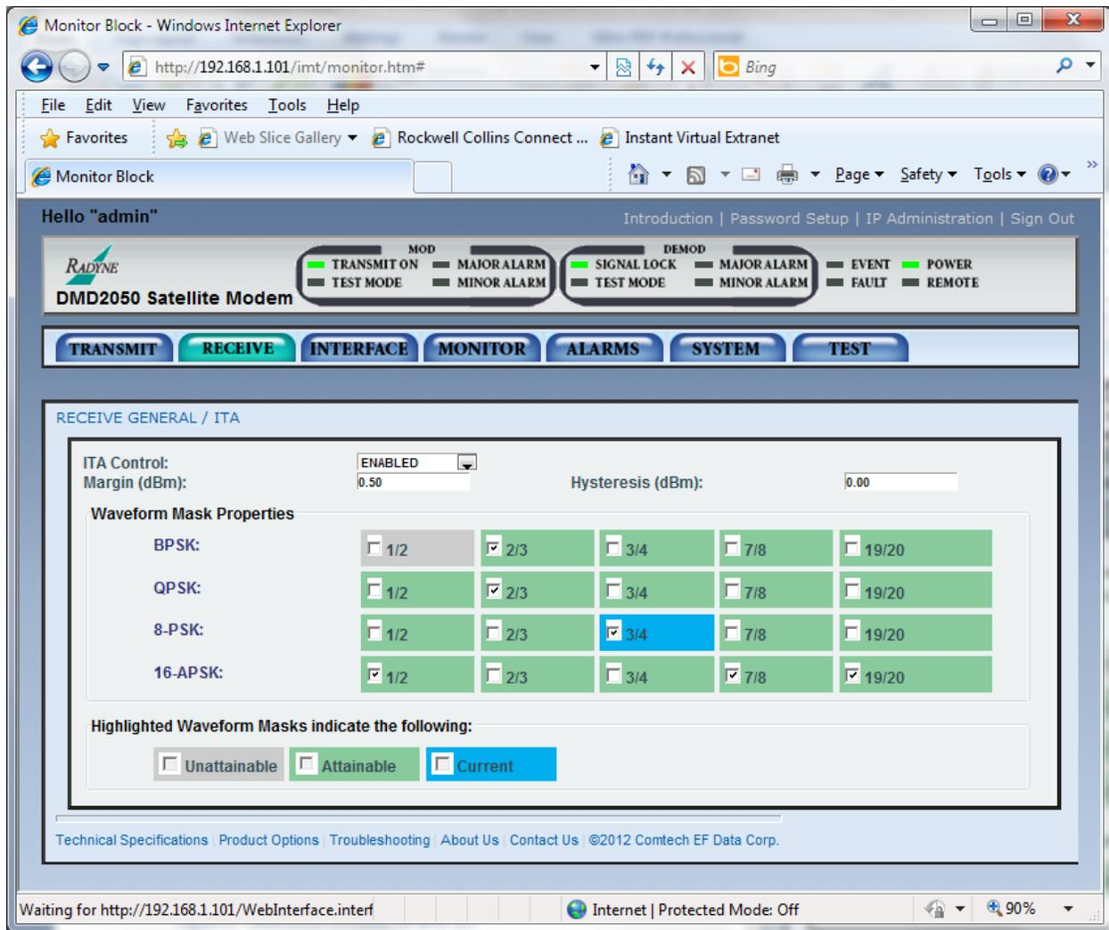
Figure J-16 –DMD2050E ITA Status for 8PSK 3/4
