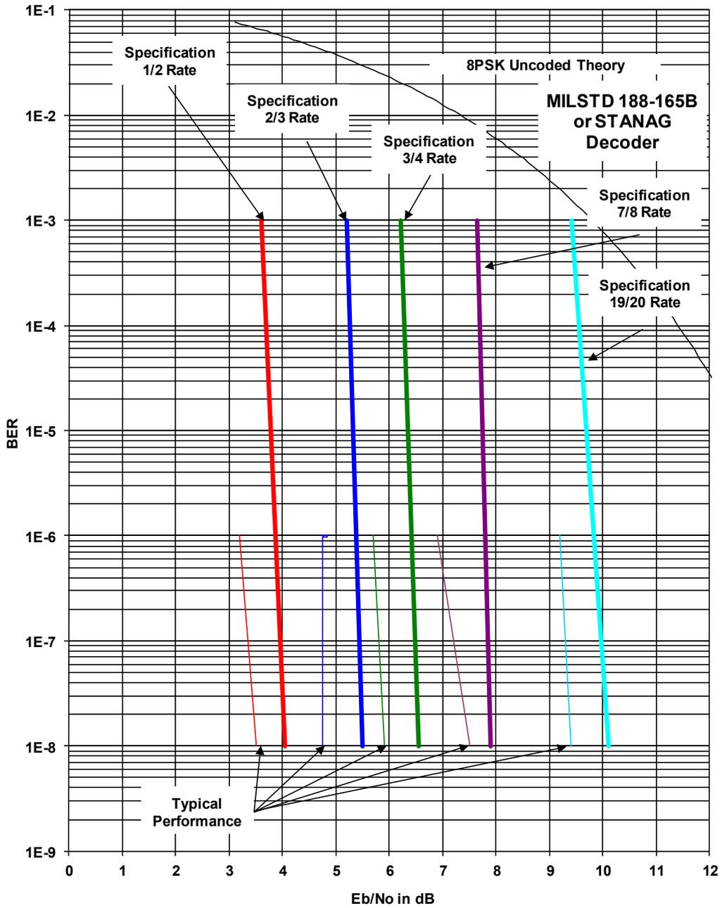
Figure 7-18. DMD2050E BER Performance 8-PSK (MILSTD 188-165B or STANAG) Turbo
