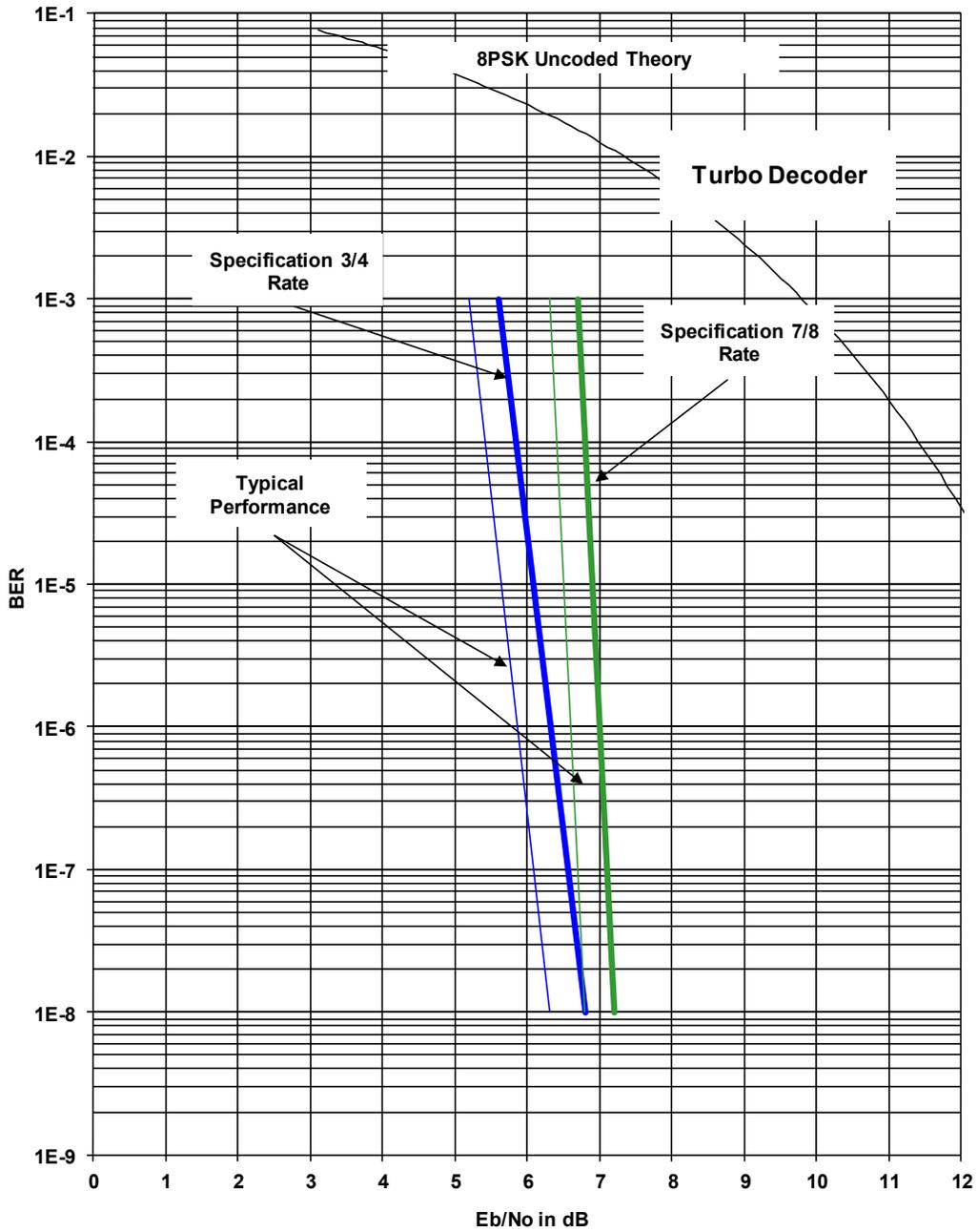
Figure 7-12. DMD2050E 8PSK BER Performance (Turbo)
