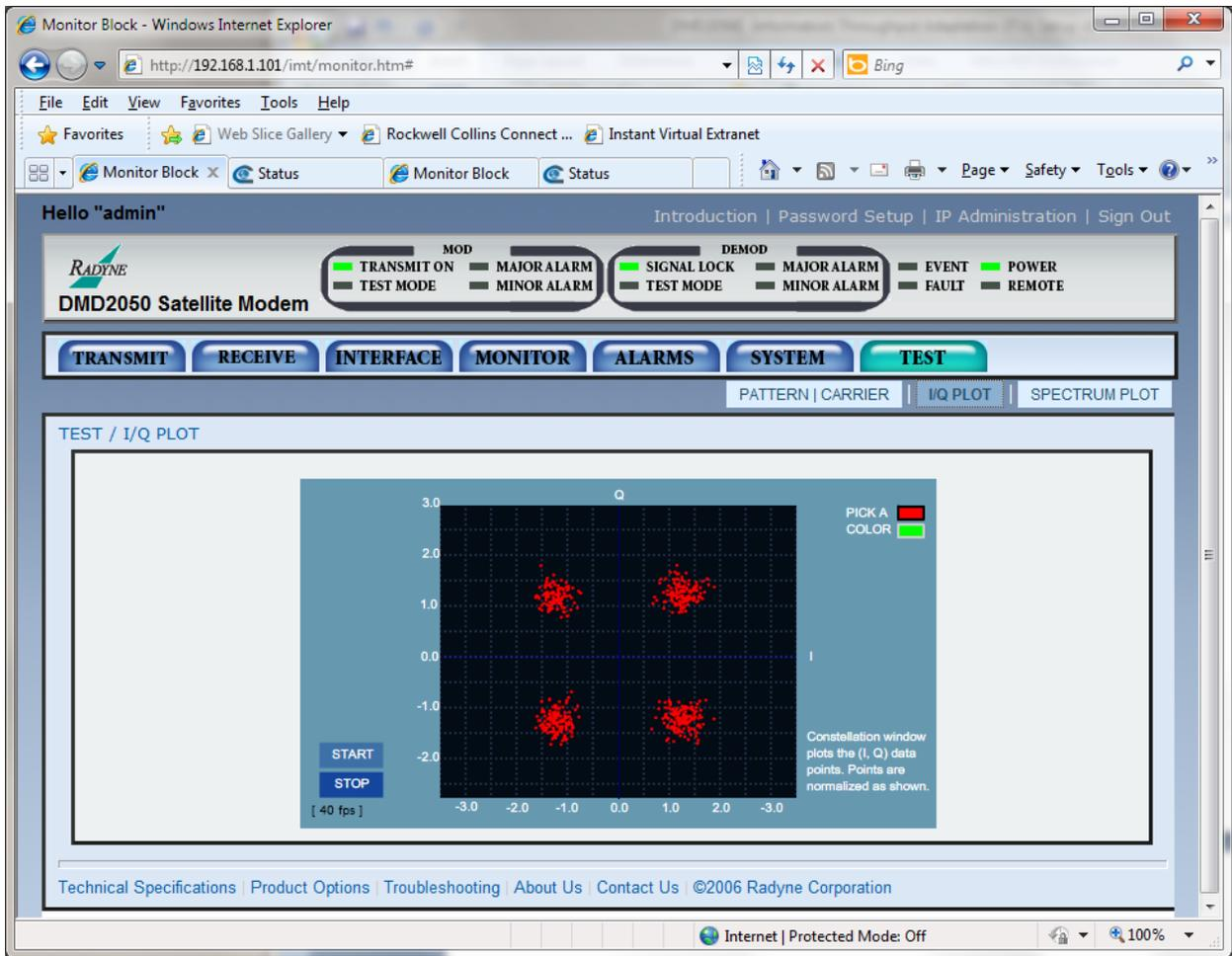
Figure J-13 –DMD2050E I/Q for QPSK 2/3
