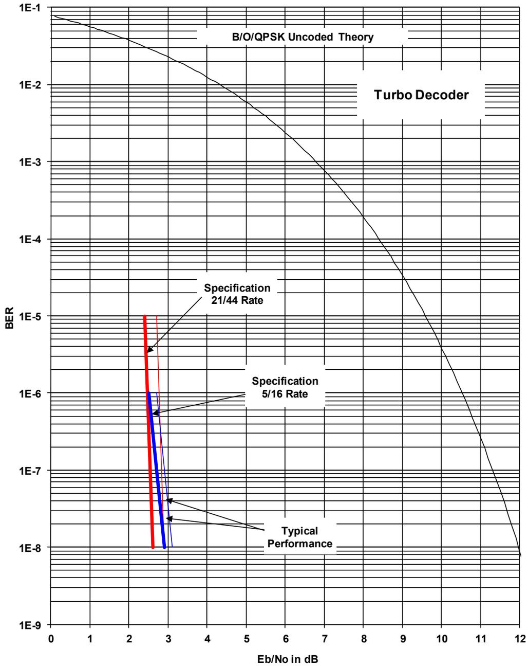
Figure 7-11. DMD2050E BPSK BER Performance (Turbo)
