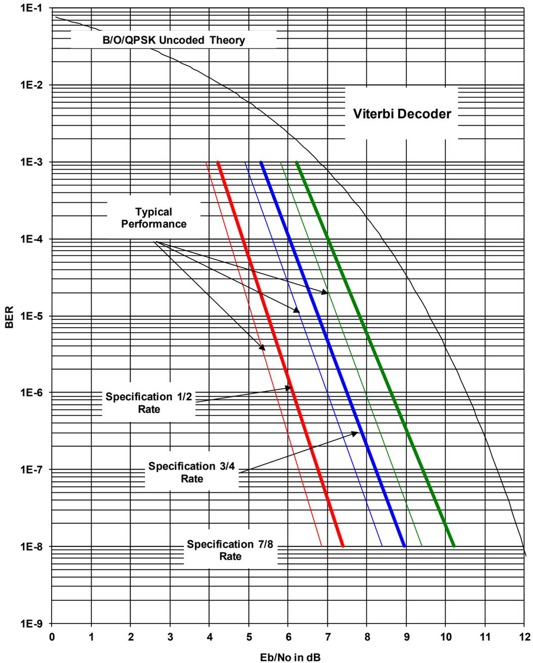
Figure 7-1. DMD2050E B/O/QPSK BER Performance (Viterbi)
