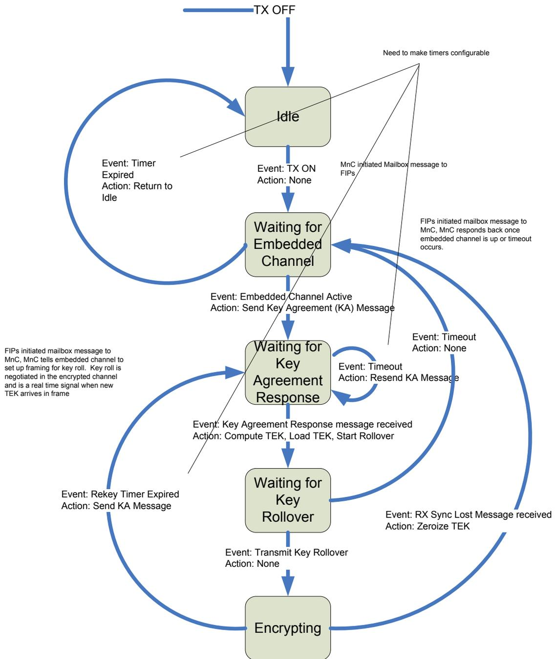
Figure 3-9. Traffic Encryption Key Negotiation
