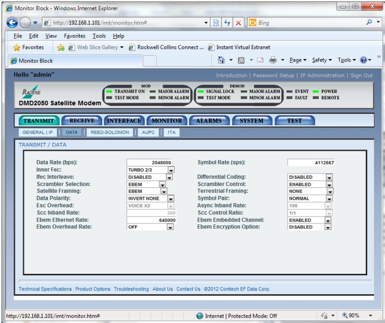
Figure J-2 - Initial Setup DMD2050E, Modulator Data
