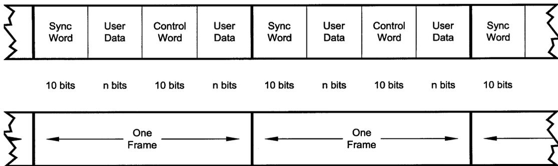
Figure 3-23. 1 to 1 Control Ratio
