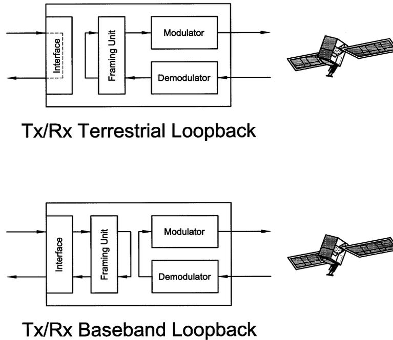
Figure 3-7. Loopback Functional Block Diagram
