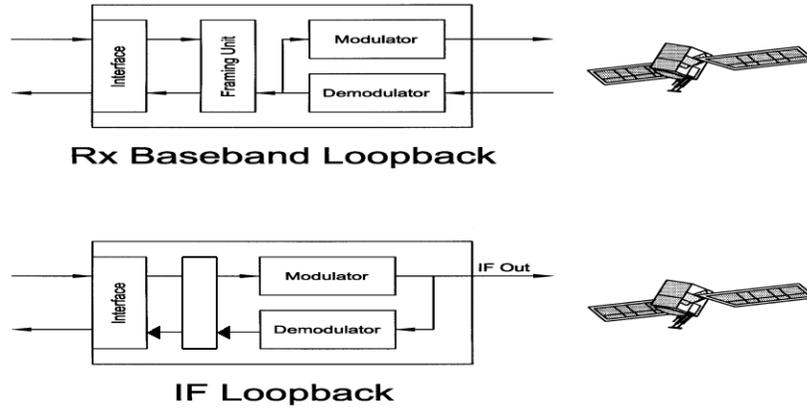
Figure 3-6. Loopback Functional Block Diagram
