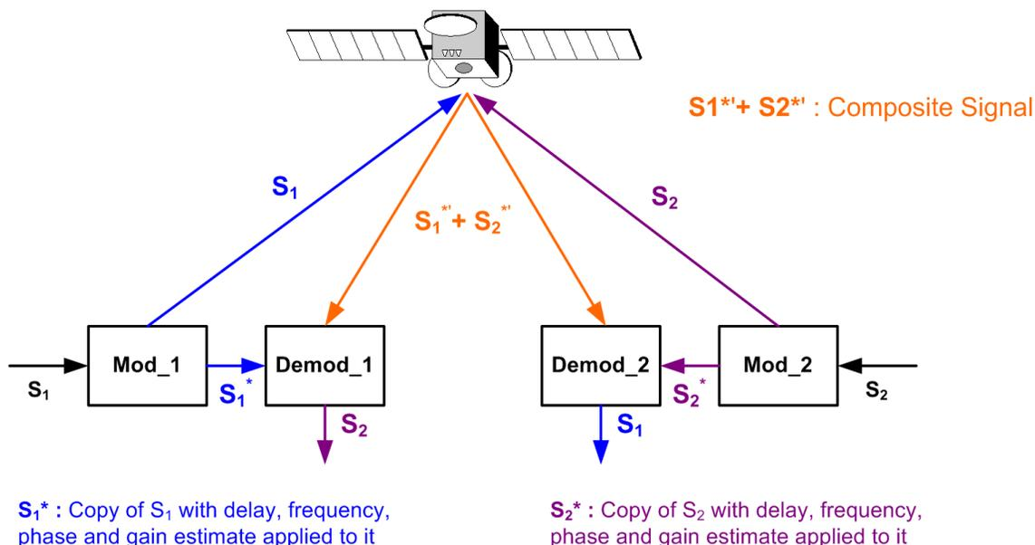
Figure 3-17. DoubleTalk Carrier-in-Carrier Signals
