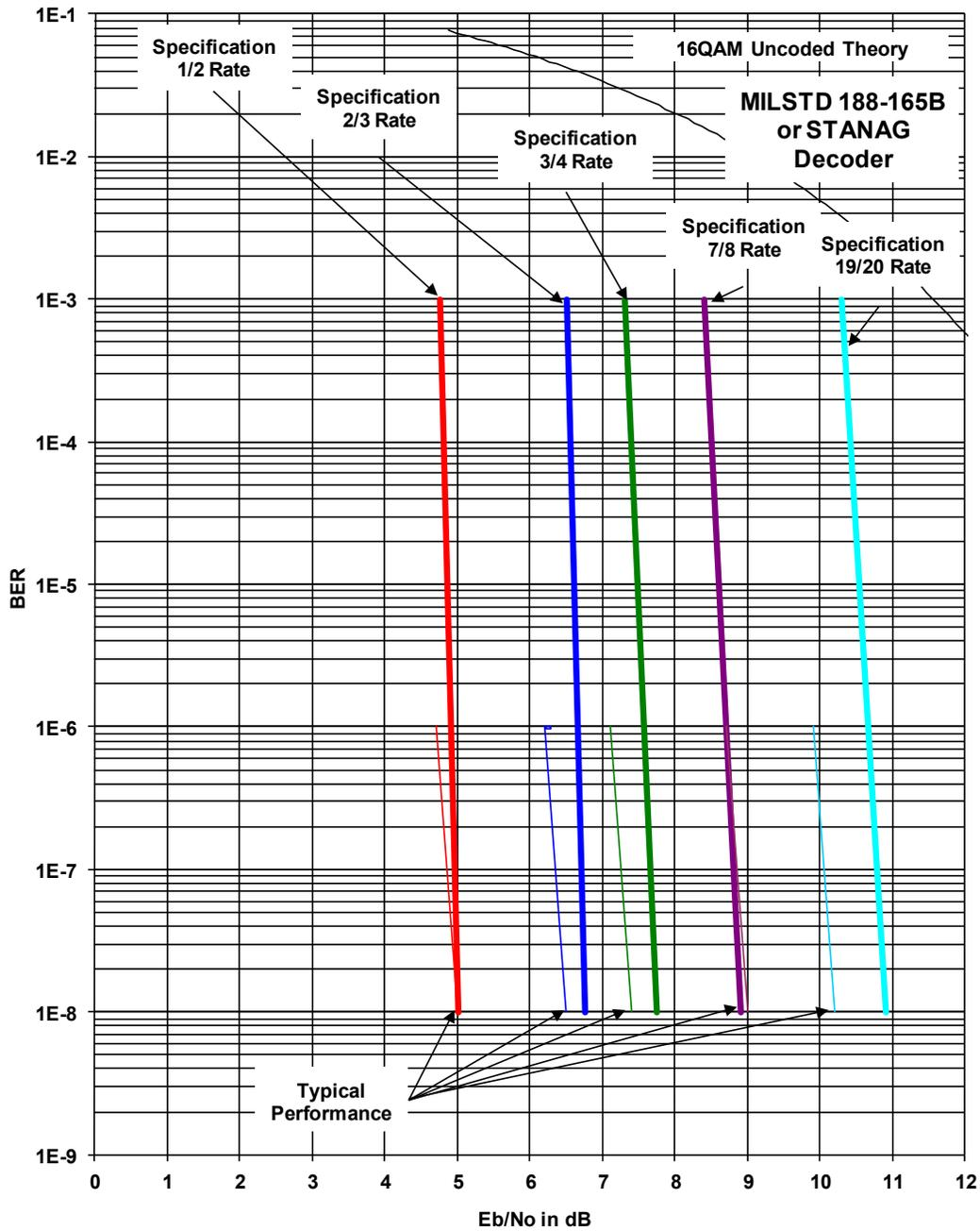
Figure 7-19. DMD2050E BER Performance 16APSK (MILSTD 188-165B or STANAG)
