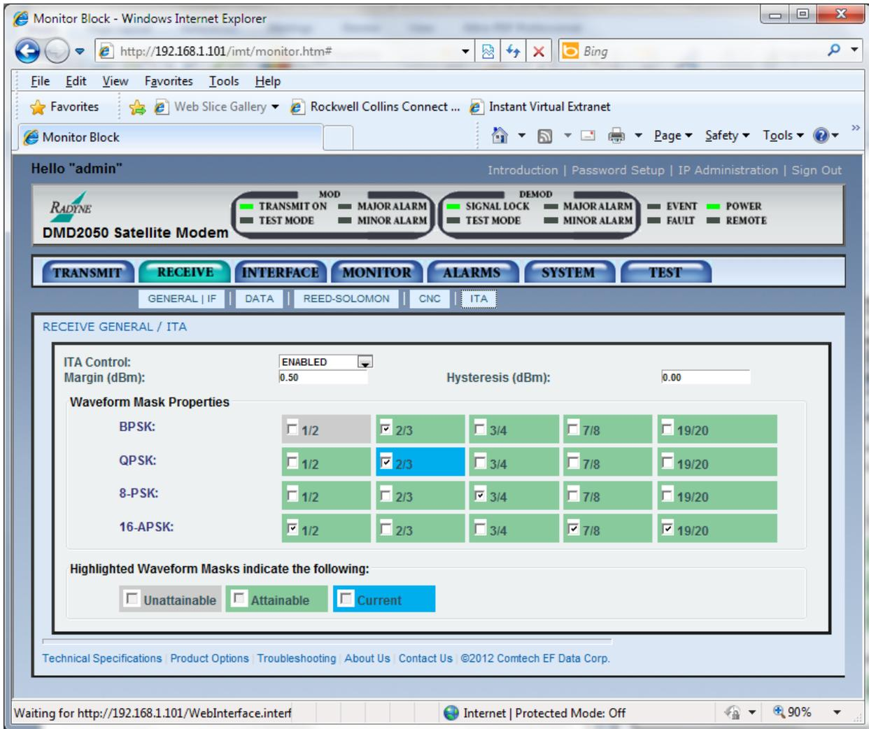
Figure J-12 –DMD2050E ITA Status for QPSK 2/3
