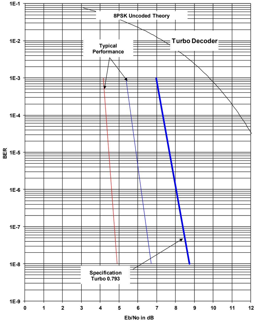
Figure 7-6. DMD2050E 8PSK BER Performance (Turbo)
