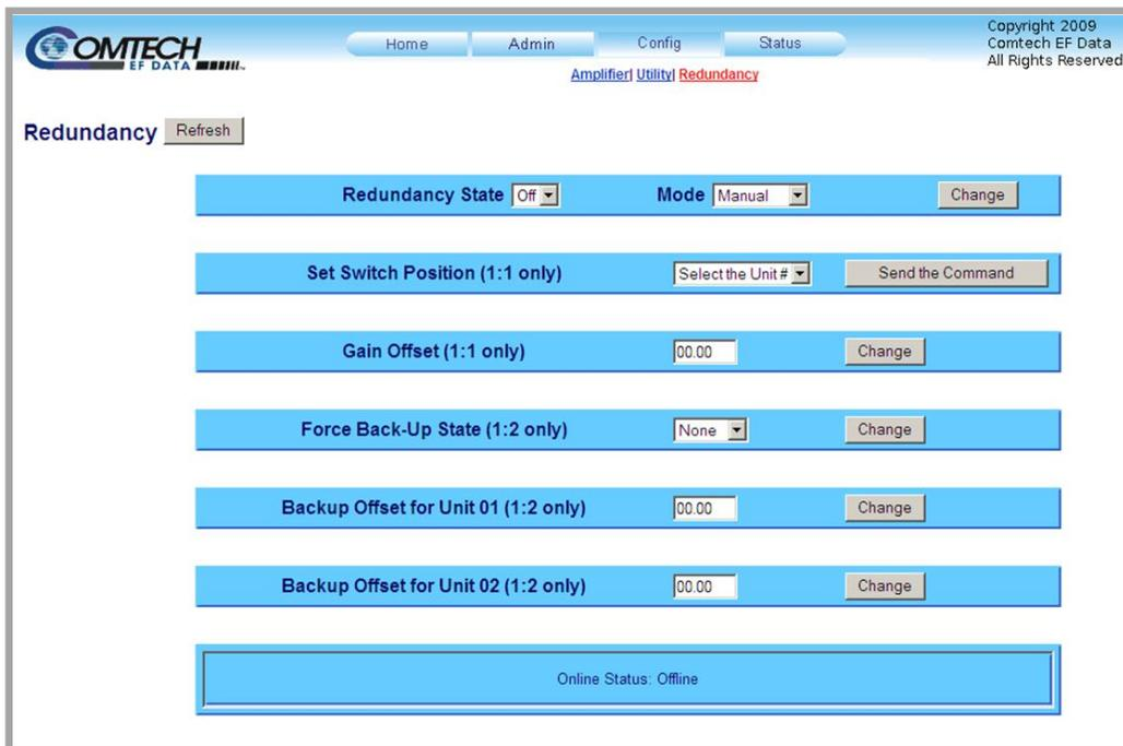
**Figure B-2. SSPA Web Server Interface – ‘Config | Redundancy’ Page**
