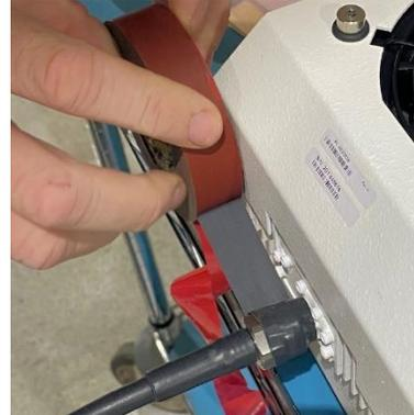
2. Pull the tape tight and use several layers. Make sure to start at the end of the connector connection.
