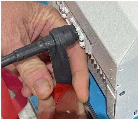
3. Verify the tape covers all of the connector and makes contact with the unit.
