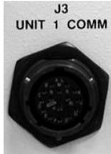
Use the **J3 | UNIT 1 COMM** connector to connect the MBT-4000B Base Module Unit 1 section to the BUC-4000 Block Up Converter Module **J6 | COMM** connector via the 15-15 Power & Signal Harness (CEFD P/N CA/WR10963-1), shown in **Figure 3-3**.
