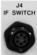
Use the **J4 | IF SWITCH** 6-pin circular connector to connect an IF switch in a 1:1 configuration to the MBT-4000B Base Module to
