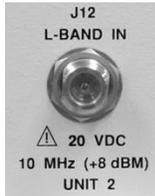
Use the **J12 | L-BAND IN** Type ‘N’ female connector to provide the down converted IF Input (via a low-noise block down converter (LNB)) to the MBT-4000B Base Module.
