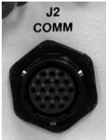
Use the **J2 | COMM** 19-pin circular connector for serial-based remote monitor and control of the MBT-4000B Multi-Band Transceiver System.
