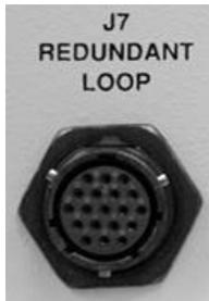
Use the **J7 | REDUNDANT LOOP** 19-pin circular connector to connect the MBT-4000B Base Module, via the Redundant Loop Bus Cable (CEFD P/N CA/WR11224), to another MBT-4000B Base Module in a 1:1 Redundancy configuration.
