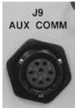
Use the **J9 | AUX COMM** 8-pin circular connector to connect a Solid-State Power Amplifier (SSPA) to the MBT-4000B Base Module.
