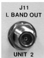
Use the **J11 | L-BAND OUT UNIT 2** Type ‘N’ female connector to connect the MBT-4000B Base Module L-Band output signal output either to the modem Rx, or the Rx IF switch or 1:2 splitter/combiner in a 1:1 configuration.
