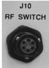
Use the **J10 | RF SWITCH** 6-pin circular connector to connect an RF Switch in a 1:1 configuration (e.g., connecting to two LNBS or SSPAs) to the MBT-4000B Base Module.
