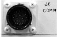
Use the **J6 | COMM** 15-pin circular connector, located on the BUC-4000 Block Up Converter Module, to connect the module, via the 15-15 Power & Signal Harness (CEFD P/N CA/WR10963-1), to the MBT-4000B Base Module **J3 | UNIT 1 COMM** connector. See **Figure 3-3**.
