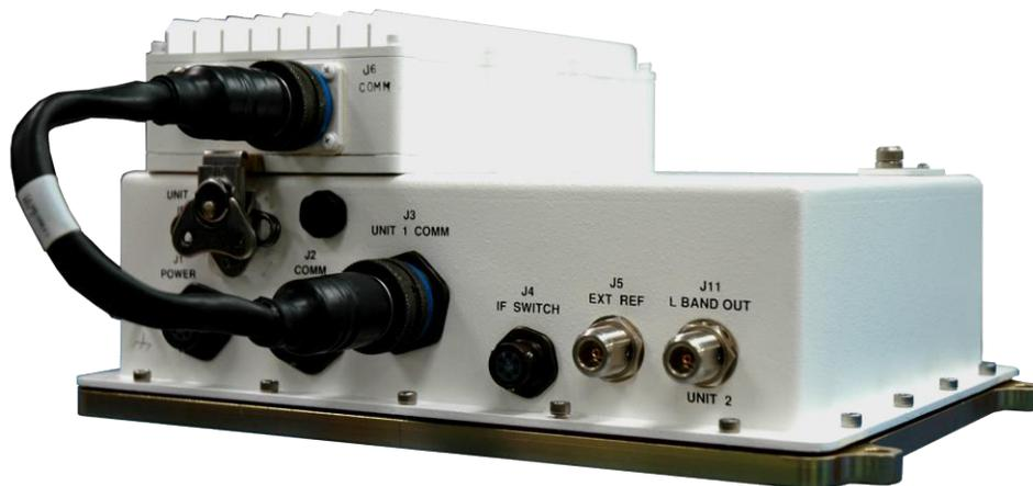
**Figure 1-1. MBT-4000B Multi-Band RF Transceiver**
