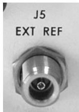
Use the **J5 | EXT REF** Type ‘N’ female connector to connect a 5 MHz or 10MHz External Reference Input to the MBT-4000B Base Module.
