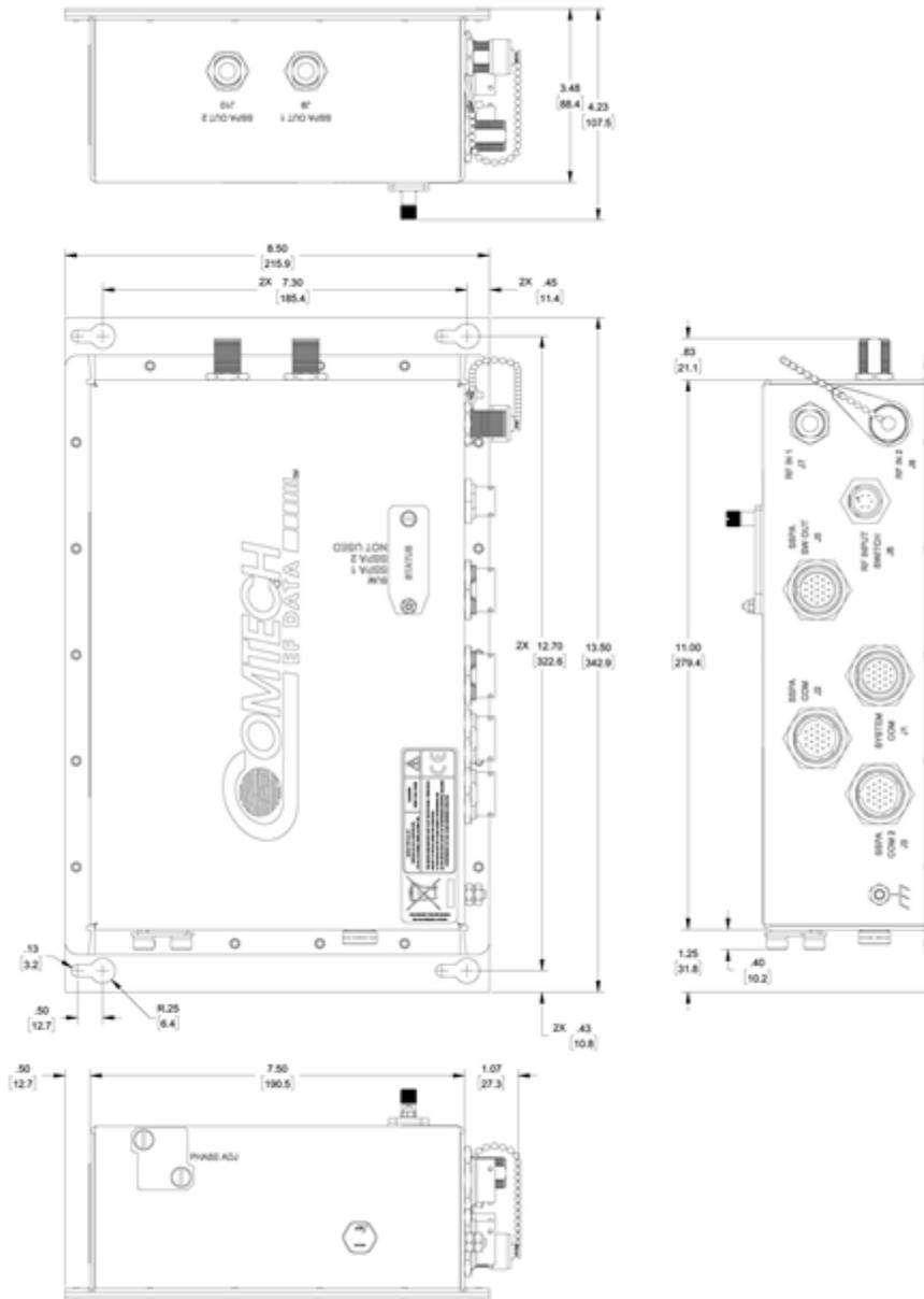
**Figure 1-4. PCB-4000A Dimensional Envelope**
