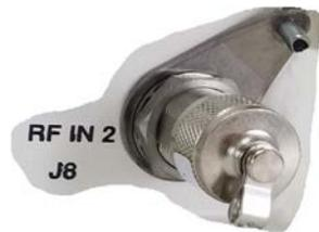
The Type 'N' **RF IN 1 | J7** and **RF IN 2 | J8** connectors serve as RF signal input interfaces to the PCCB. Note that:
