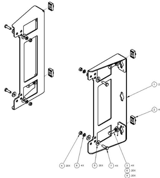
Figure A-9. Vertical Frame Uni-Strut Mount HPOD Mounting Bracket Kit (KT-0021261)
