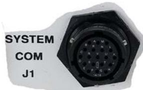
The 19-pin circular **SYSTEM COM | J1** connector, type MS3112E14-19S, serves as the primary input between the user and the PCCB for controlling and monitoring both SSPAs. Its pinout specification is provided in Table 2-2.
