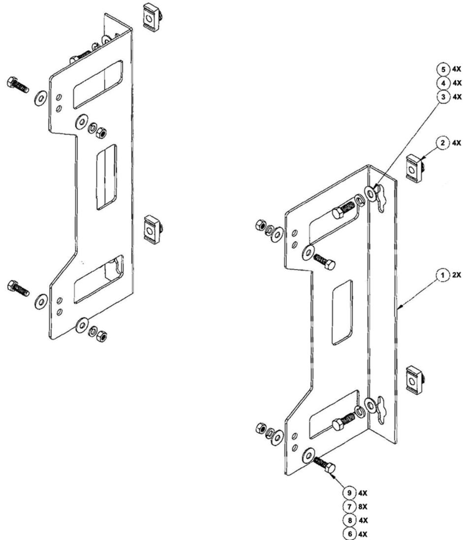
**Figure A-8. Uni-Strut Mount HPOD Mounting Bracket Kit (KT/12300-1)**
