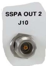
The Type 'N' **SSPA OUT 2 | J10** connector, located on the right side panel of the PCCB, provides the RF signal output from the PCCB to SSPA #2.
