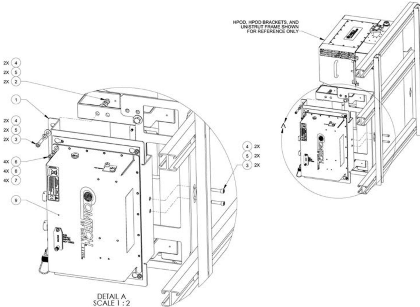
**Figure A-3. Phase Combiner Box and Bracket Kit (KT-0021171)**
