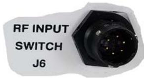
The PCCB contains a built-in selector switch – a latching 28 VDC coaxial unit. The switch position is selected by the 6-pin circular **RF INPUT SWITCH | J6** connector (P/N CN/MS-PT07M6PC). Its pinout specification is provided in Table 2-5.
