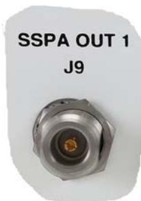
The Type 'N' **SSPA OUT | J9** connector, located on the left side panel of the PCCB, provides the RF signal output from the PCCB to SSPA #1.
