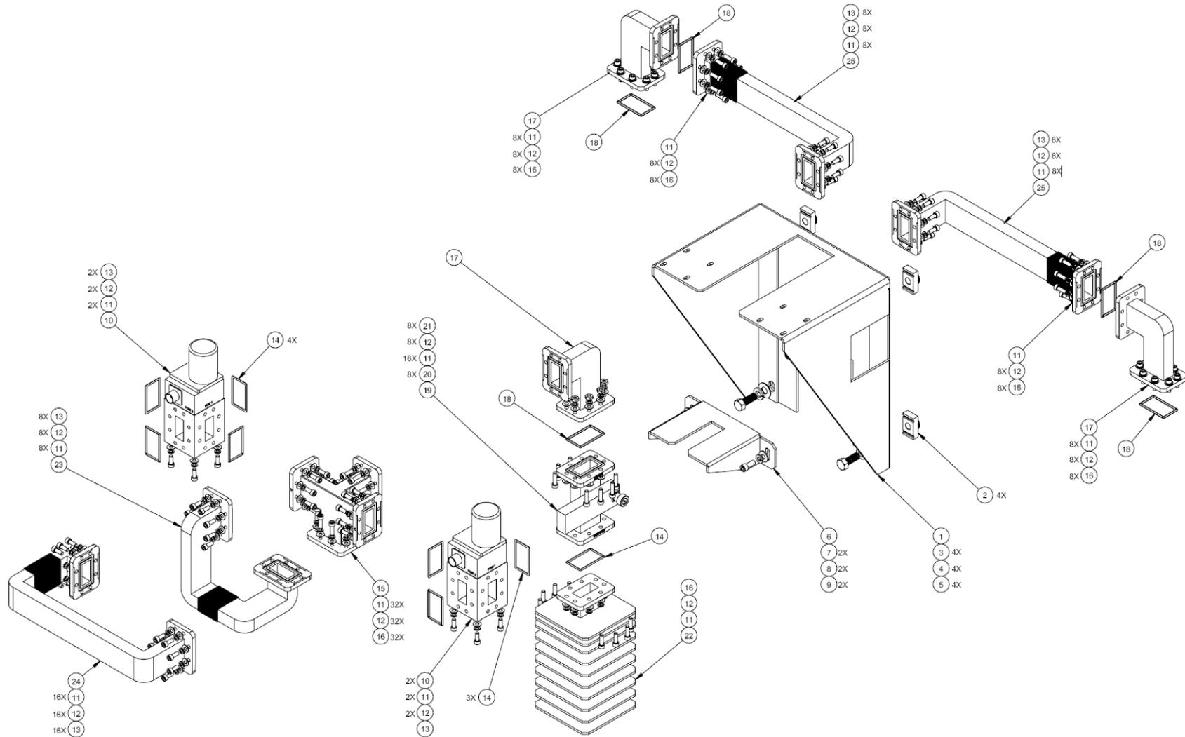
Figure A-4. C-Band 1:1 Phase Combined Waveguide and Switches, HPOD (KT-000054)
