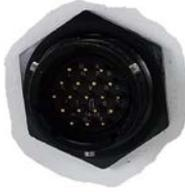
The 19-pin circular **SSPA COM 1 | J2** and **SSPA COM 2 | J3** connectors, type MS3112E14-19S, serve as the primary input/output interfaces between the PCCB and its specified SSPA. The typical pinout specification is provided in Table 2-3.
