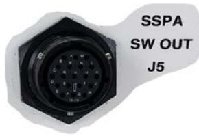
The 19-pin circular **SSPA SW OUT | J5** connector, type MS3112E14-19S, connects via a “Y” cable to the SSPA #1 and SSPA #2 waveguide switches. The typical pinout specification is provided in Table 2-4.
