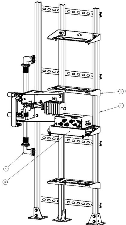
Figure A-5. Vertical Mounting Frame Kit (KT-0021179)
