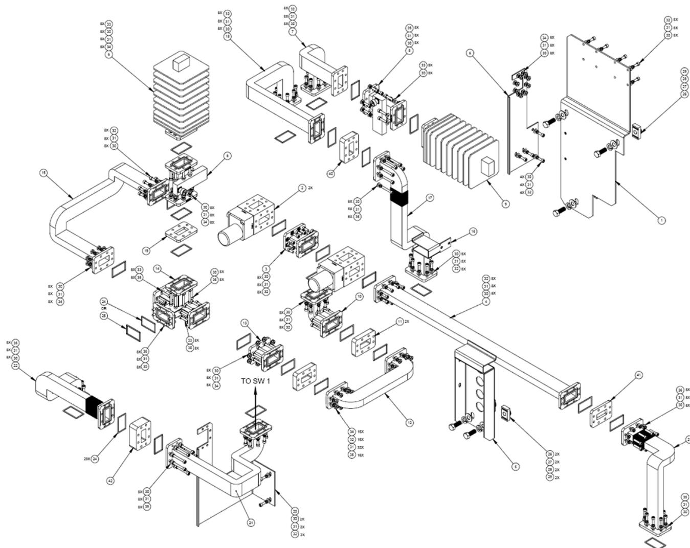
Figure A-5. C-Band 1:2 Phase Combined System Waveguide Kit (Exploded) – HPOD (KT-0000107)
