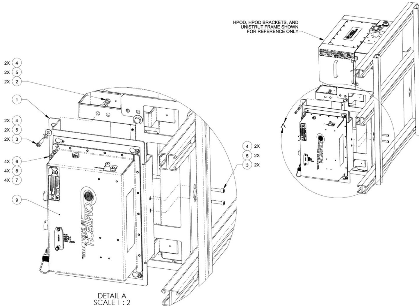
**Figure A-6. C-Band 1:2 Phase Combiner Box and Bracket Kit (KT-0021154)**
