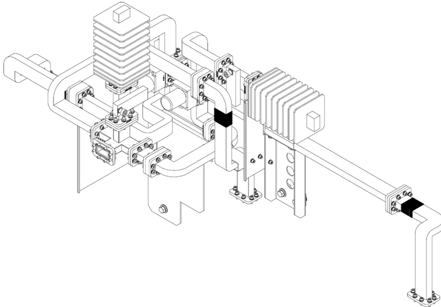
**Figure A-4. C-Band 1:2 Phase Combined System Waveguide Kit (Assembled) – HPOD (KT-0000107)**
