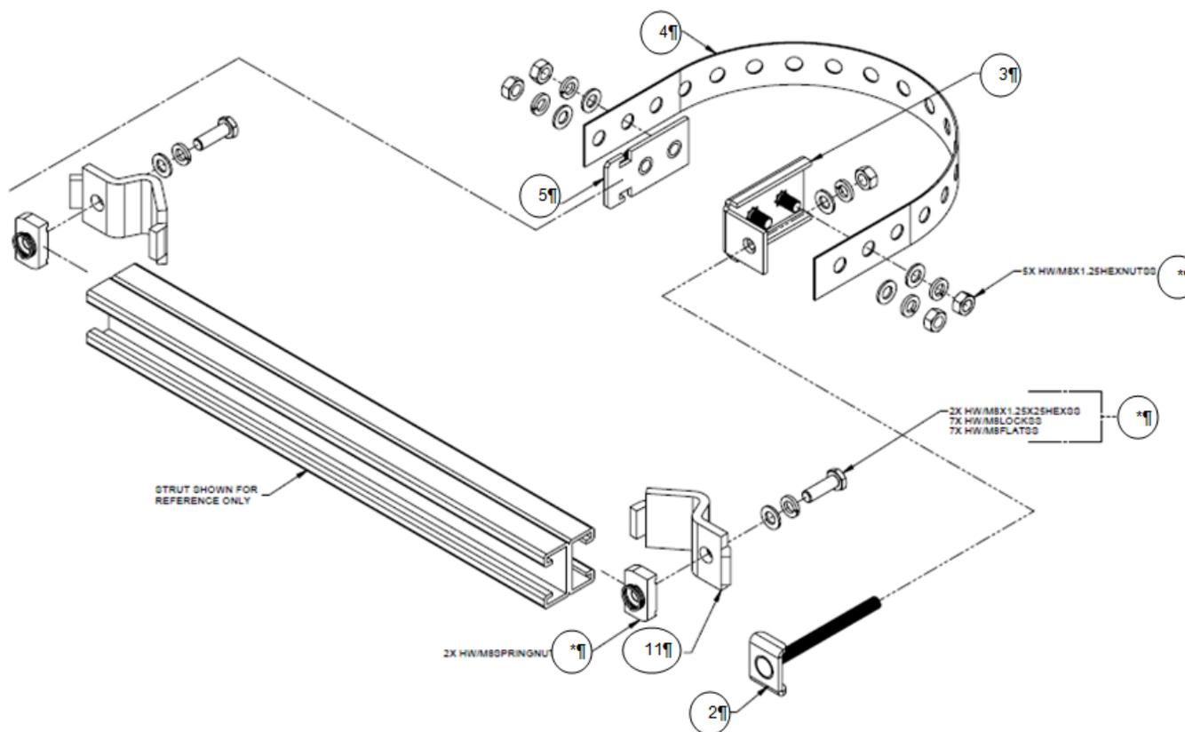
Figure A-8. HPOD 1:1 Redundancy Pole Mount Kit (PL/12319-1)
