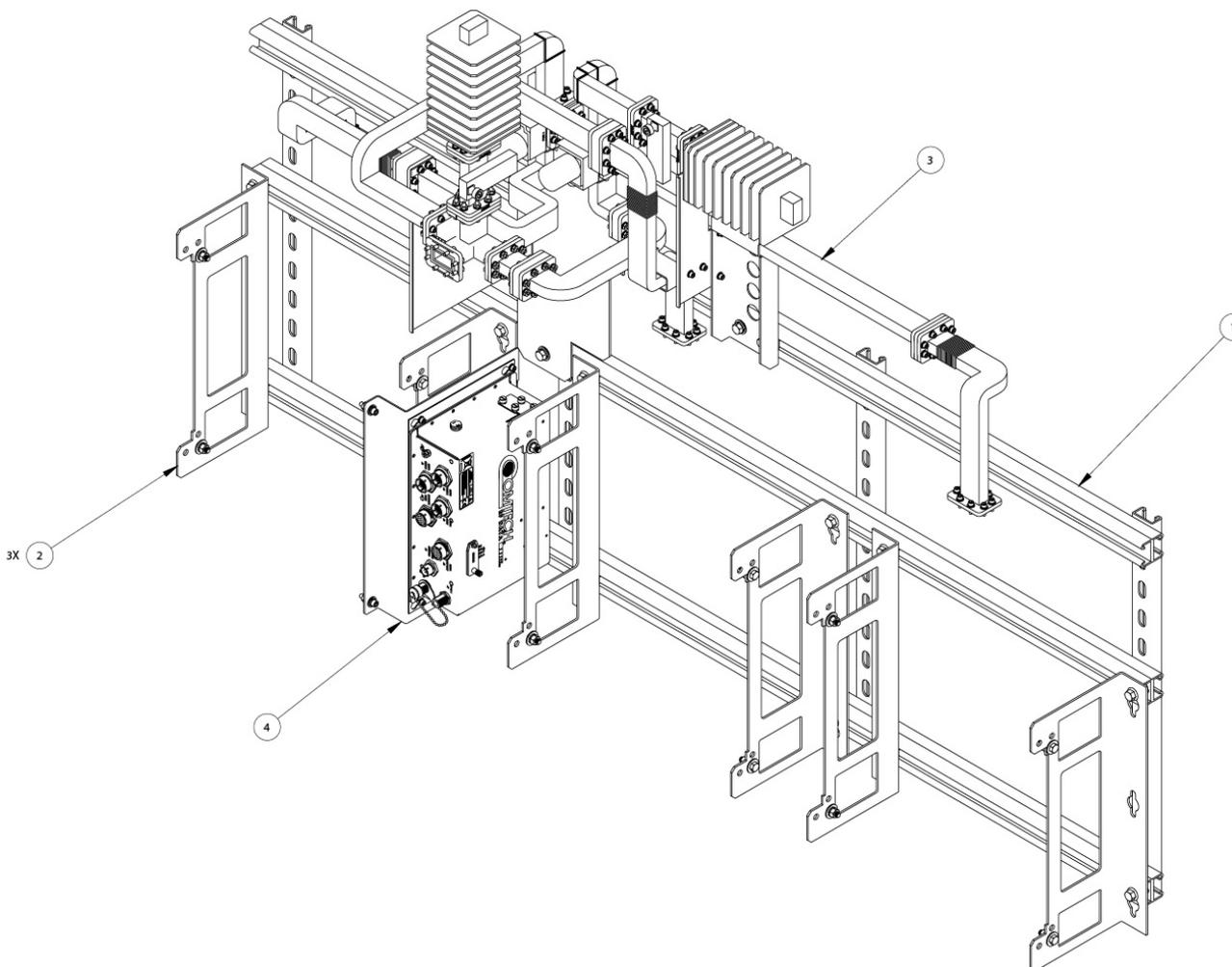
Figure A-2. C-Band 1:2 Phase Combined Top Assembly Kit – 350W HPOD (KT-0000109) (Vertical Load)
