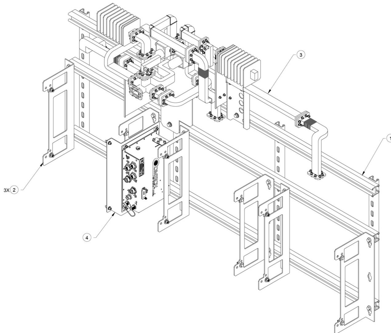
Figure A-3. C-Band 1:2 Phase Combined Top Assembly Kit – 350W HPOD (KT-0021054) (Horizontal Load)
