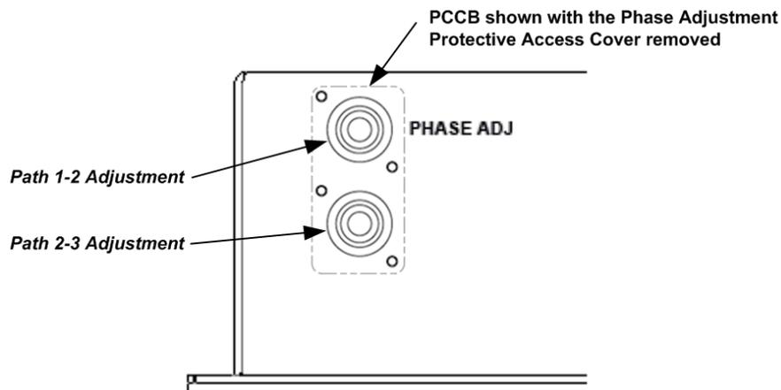
**Figure 3-6. Phase Shifter Adjustment Locations**
