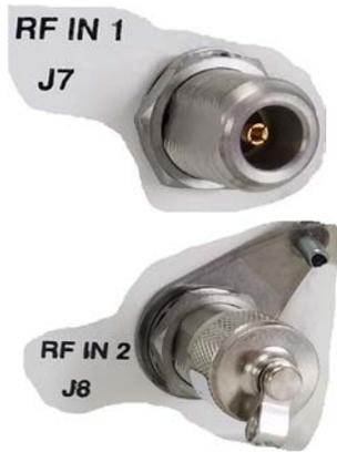
The **RF IN 1 | J7** and **RF IN 2 | J8** connectors are Type 'N' female connectors, each serving as an RF signal input interface to the PCCB. Note the following:
