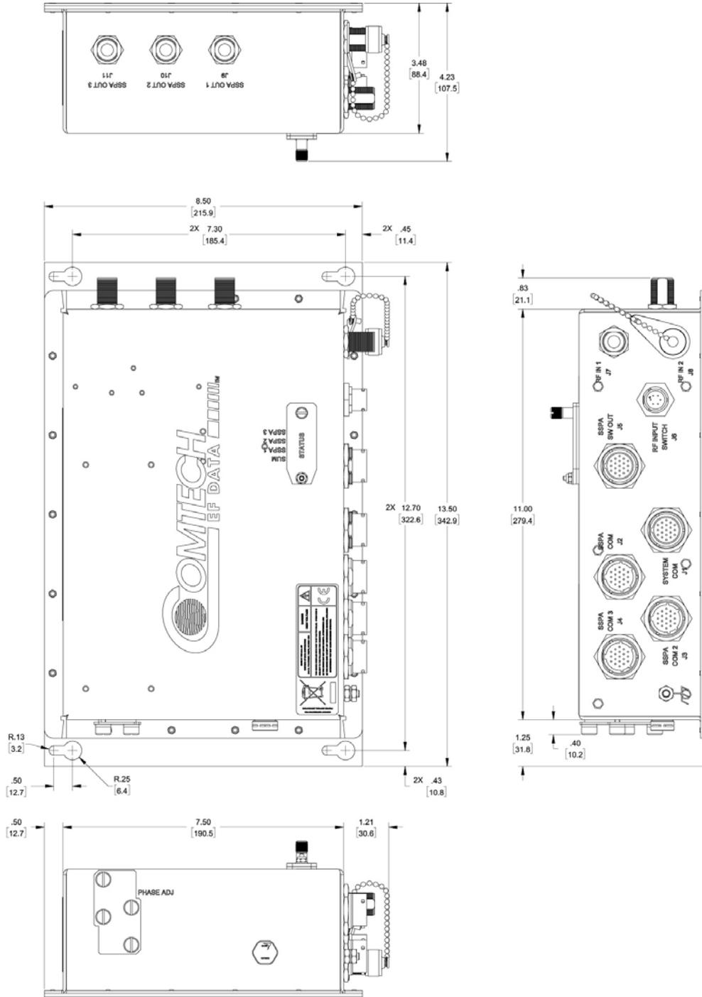
Figure 1-4. PCB-4300A Dimensional Envelope
