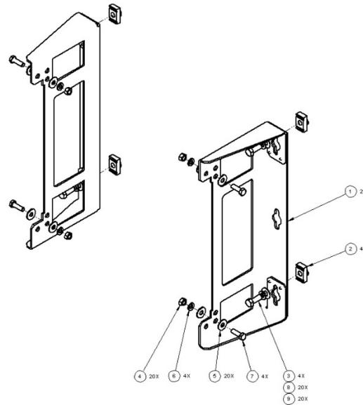
Figure A-11. Vertical Uni-Strut Mount HPOD Mounting Bracket Kit (KT-0021261)
