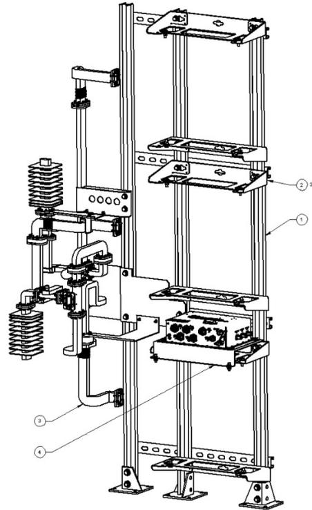
Figure A-7. Vertical Mounting Frame Kit (KT-0021177)
