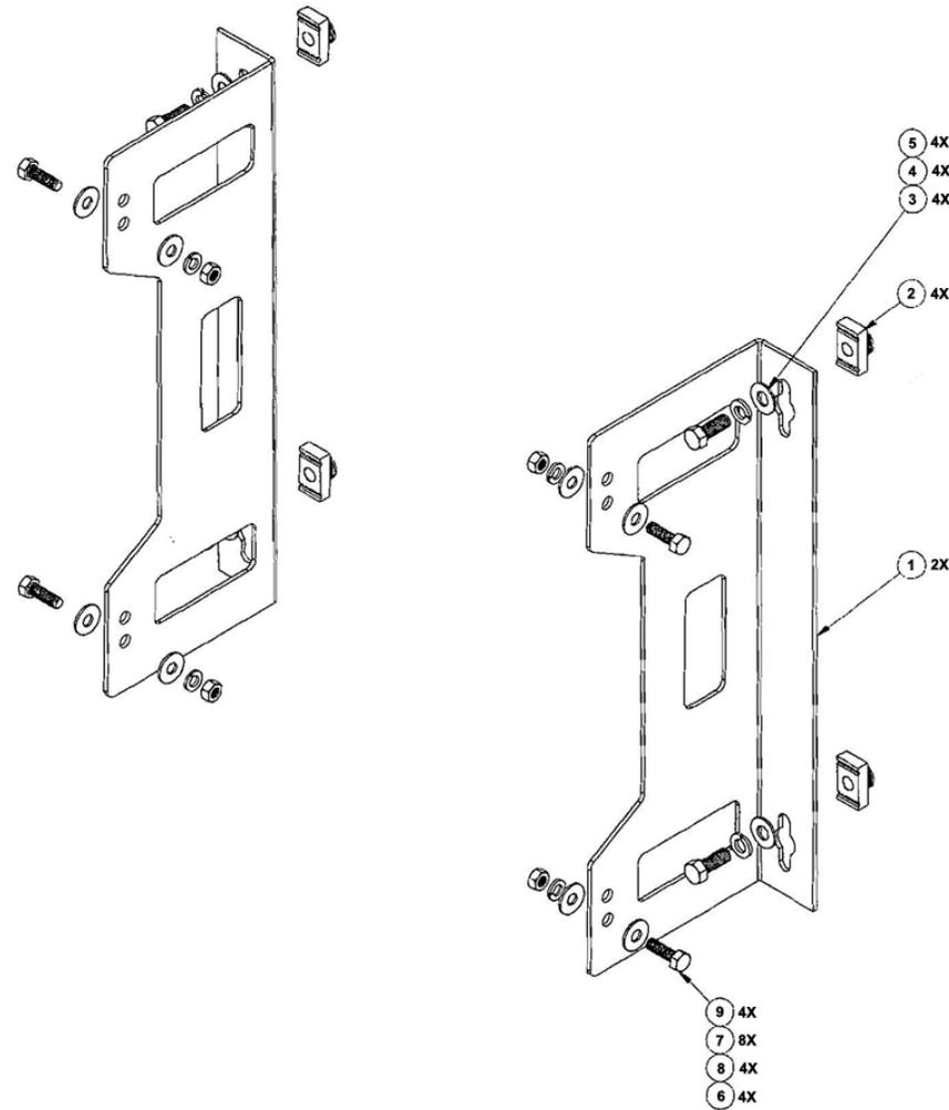
Figure A-10. Uni-Strut Mount HPOD Mounting Bracket Kit (KT/12300-1)
