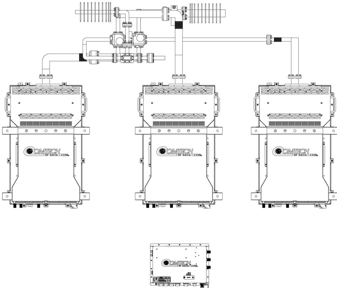
Figure 3-1. PCB-4300A 1:2 Phase Combiner System Assembly Example
