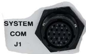
The 19-pin circular **SYSTEM COM | J1** connector, type MS3112E14-19S, serves as the primary input between the user and the PCCB for controlling and monitoring all SSPAs. Its pinout specification is provided in Table 2-2.
