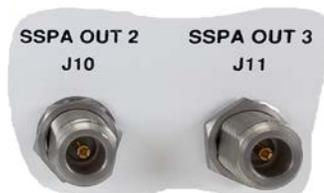
The **SSPA OUT 2 | J10** and **SSPA OUT 3 | J11** connectors, located on the right side panel of the PCCB, are Type 'N' female connectors. They provide the RF signal outputs from the PCCB to SSPA #2 and SSPA #3.
