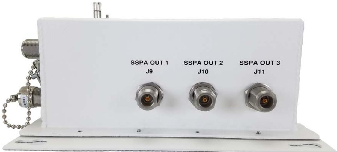
Figure 3-3. PCB-4300A External Connectors – Right Side
