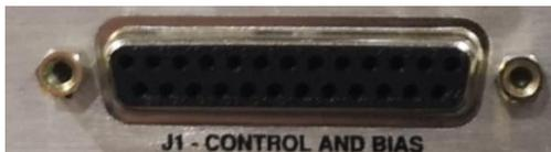
The LNA/LNB J1 connector is a 25-pin D socket and can mate with any 25-pin miniature D connector plug. See Table 2-2 for connector pinouts.
