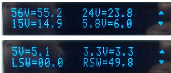
This screen shows the controller internal voltages. These will be shown as “N/A” if not monitored.
