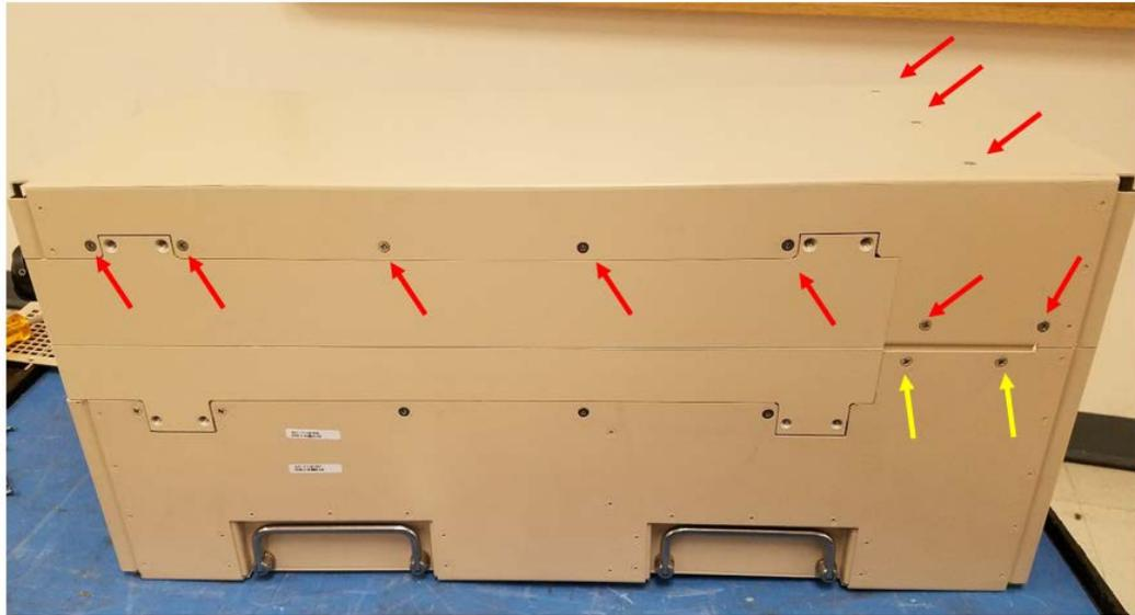
**Figure 6-8. Power Supply Chassis Screw Location
