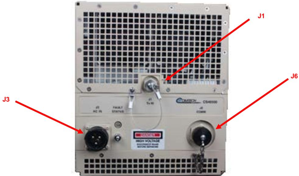
Figure 2-2. TRP500-GaN Interface Connectors – Back
