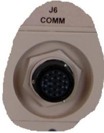
The ‘J6 | COMM 1’ Remote Communications/Discrete Control connector is a 19-pin circular connector, type MS3112E14-19S. It is the primary input for remote M&C of the SSPA.
