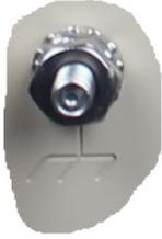
A #10-32 stud is provided at the location, shown in Figure 2-3, for connecting a common chassis ground among equipment.
