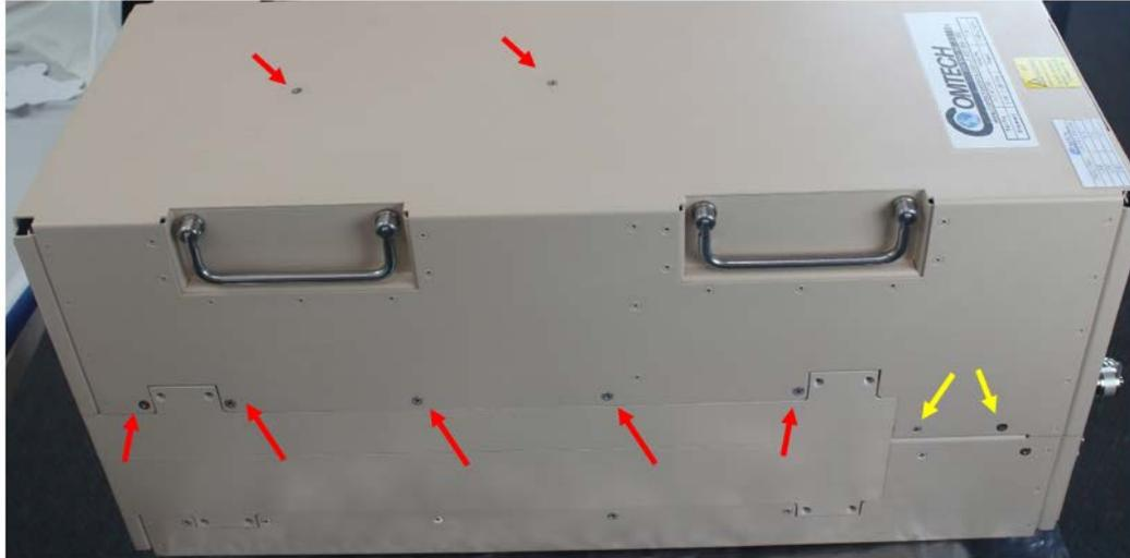
**Figure 6-6. RF Chassis Cover Screw Locations**
