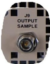
The output Sample Port connector is found on the left-hand side of the front chassis. It is a Type ‘N’ female connector that provides a nominal -50 dB sample of the output signal. A calibration label, provided near the connector, shows the actual coupling values vs. frequency.
