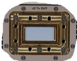
The ‘J2 | RF OUT’ connector is a CPR187G waveguide flange interface. Be careful not to allow any unwanted material to enter the waveguide output while the interface is open. The opening is covered with a protective material during shipment. Assuming the mating flange is also a type CPR187G interface, use the supplied gasket to ensure a watertight connection, and make sure the screws used to secure the mating flange do not bottom out.
