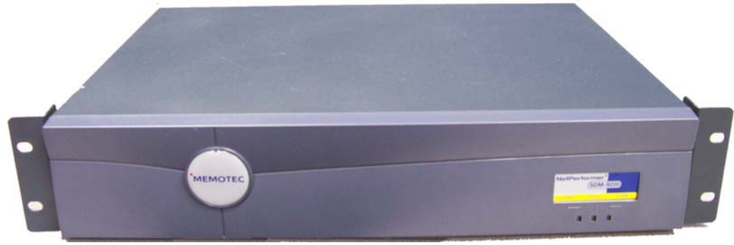
Figure 4-9: SDM-9220/9230 Installed with Rackmount Brackets
