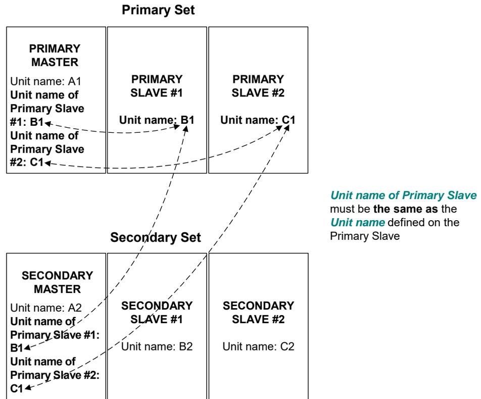
Figure 7-4: Assigning the Unit Name of Primary Slave
