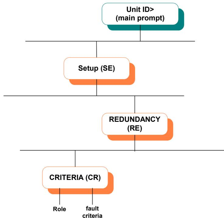
Figure 3-4: SETUP/REDUNDANCY/CRITERIA Path in the CLI Tree
