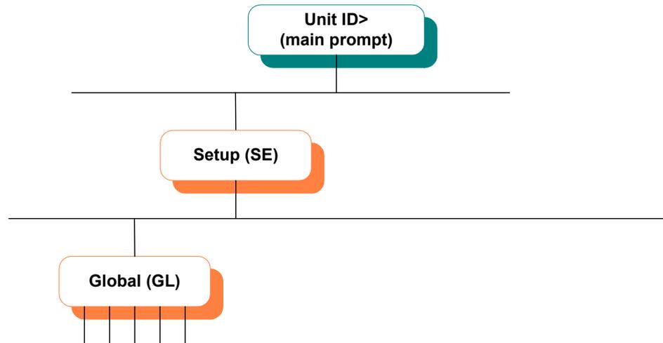
Figure 3-1: SETUP/GLOBAL Path in the CLI Tree
