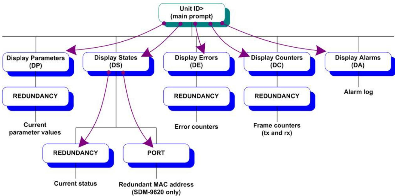
Figure 6-1: Redundancy Display Commands on the CLI Path
