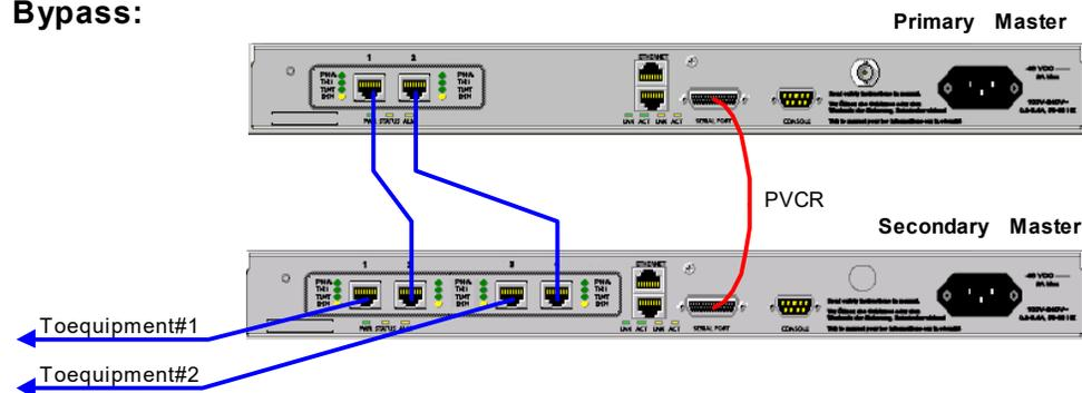
Figure 4-1: Redundant SDM-9210 Units with Digital Link Bypass and 1:1 Redundancy
