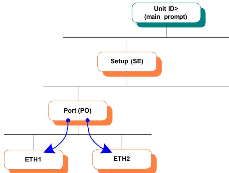
Figure 5-2: SETUP/PORT/ETH1 and SETUP/PORT/ETH2 Path in the CLI Tree
