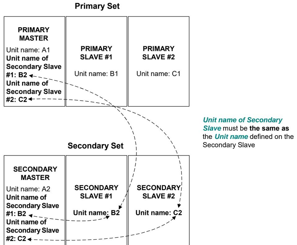
Figure 7-5: Assigning the Unit Name of Secondary Slave
