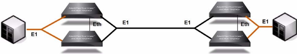
Figure 4-5: 1:1 Redundancy Mode at Both Sides of the Network
