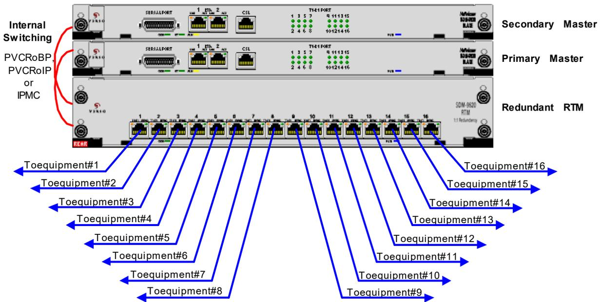
Figure 5-1: SDM-9620 Units with 1:1 Redundancy
