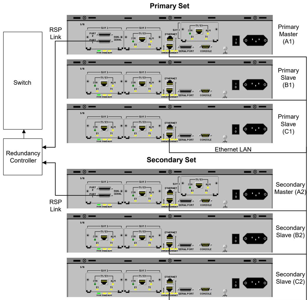
Figure 1-3: Redundant System using Standalone Units
