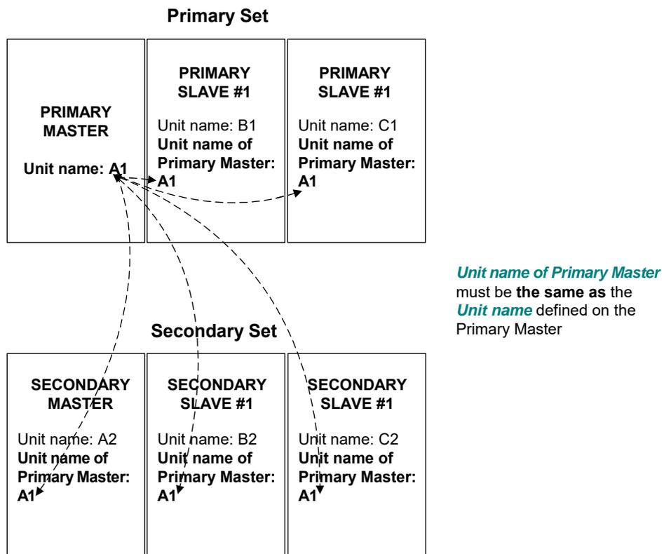
Figure 7-2: Assigning the Unit Name of Primary Master
