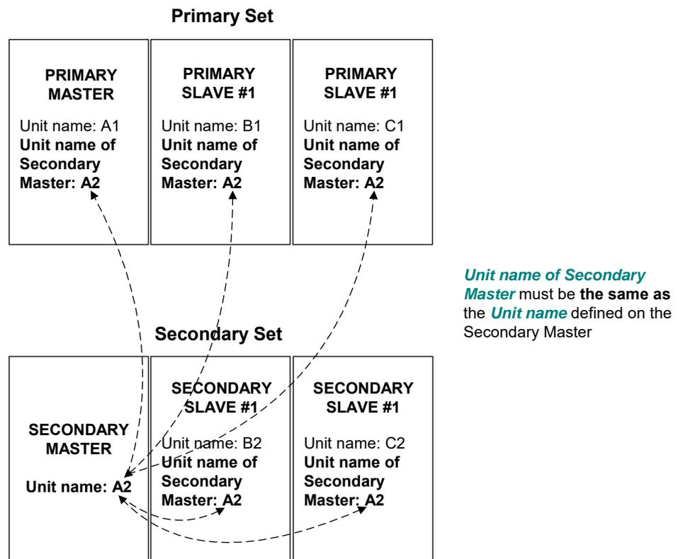
Figure 7-3: Assigning the Unit Name of Secondary Master
