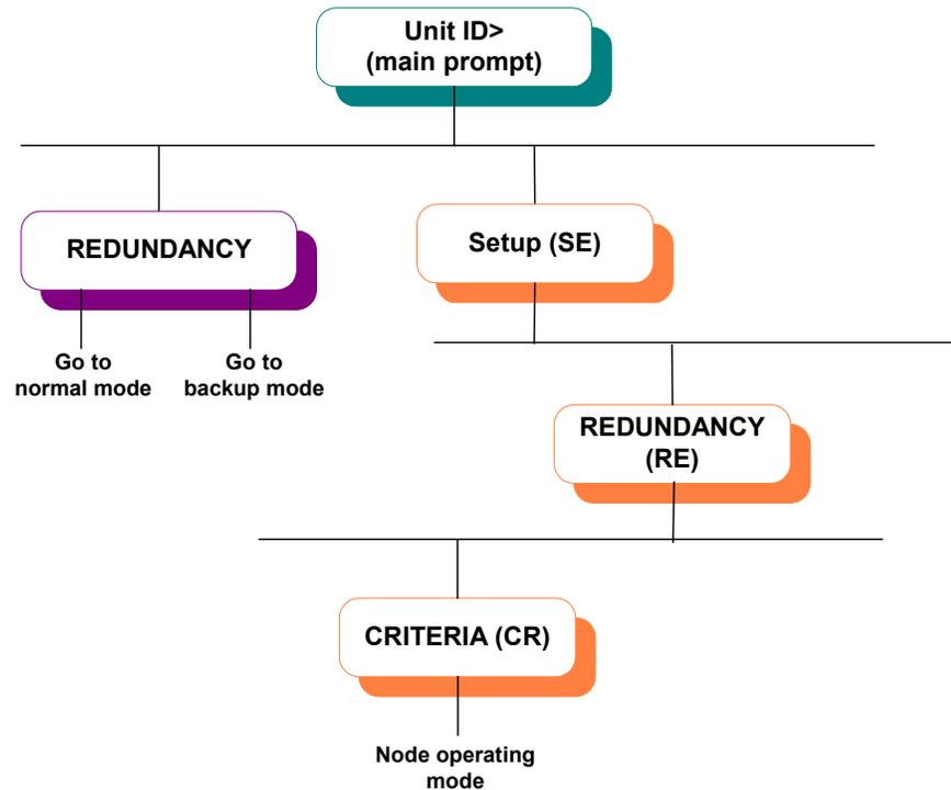
Figure 2-1: Command Paths in the CLI Tree for Switching the Mode of a Redundant System
