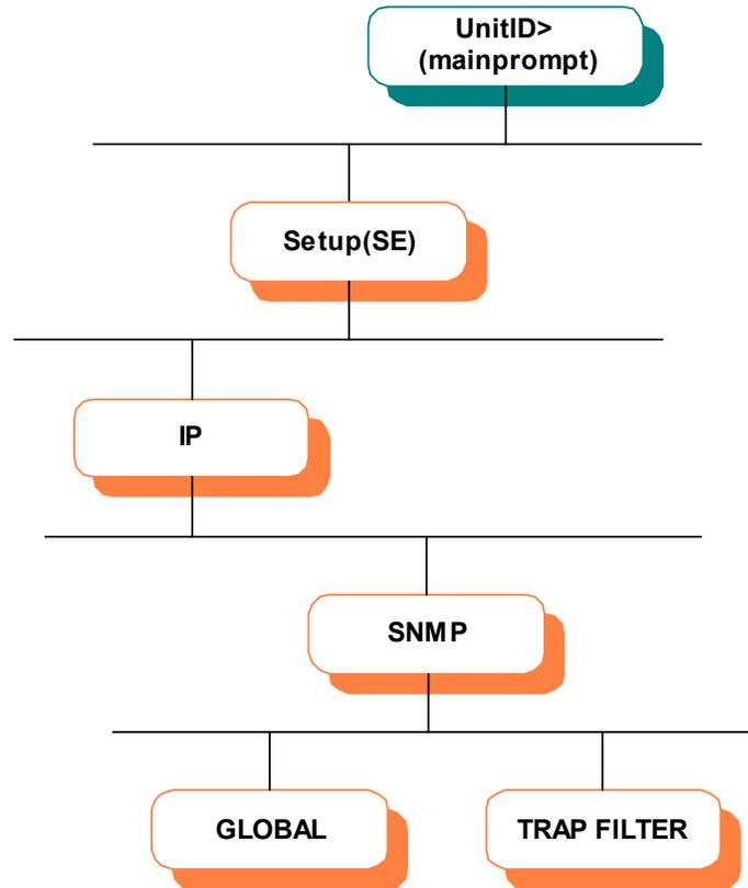
Figure 3-6: SETUP/IP/SNMP/TRAP FILTER Path in the CLI Tree
