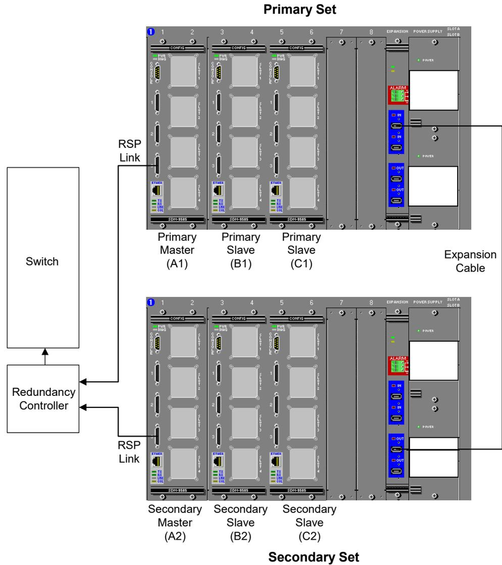
Figure 1-2: Redundant System using SDM-9500 Chassis
