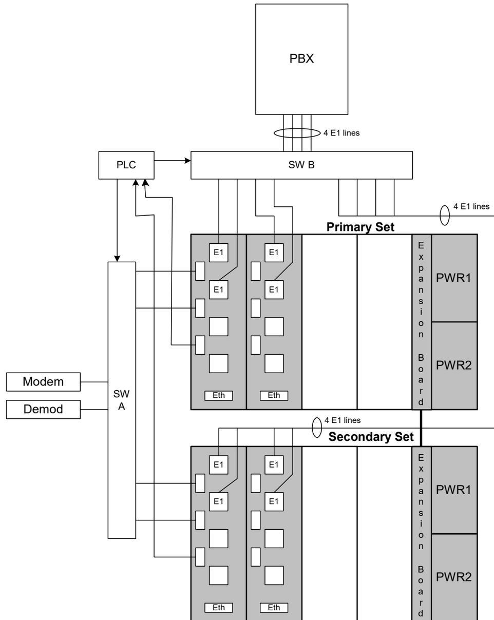
Figure 1-1: Typical Equipment Setup for Redundancy Controller
