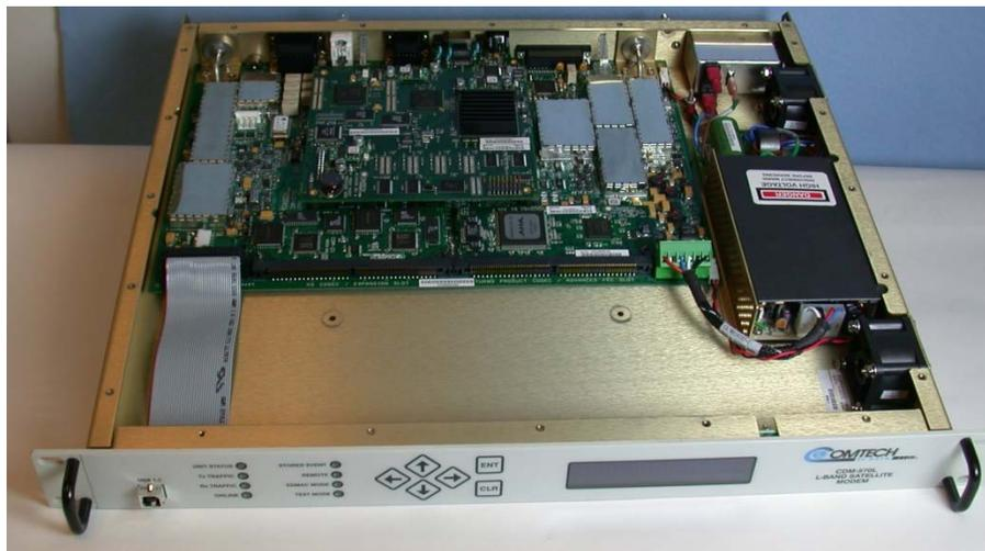
Figure 1. MPP70 correctly installed in the CDM-570L modem
