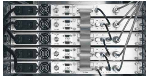
Typical 1+4 Downlink Switching
