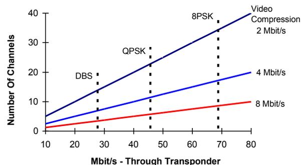
Figure 1. Number of Channels versus Transponder Capacity
