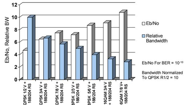
Figure 4. Power ( $E_b/N_0$ ) And Bandwidth Versus Modulation And Coding
