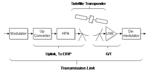
Figure 2. Transmission Model
