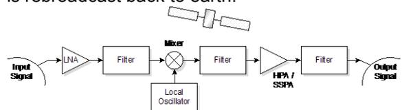
Figure 5. Satellite Transponder Model
