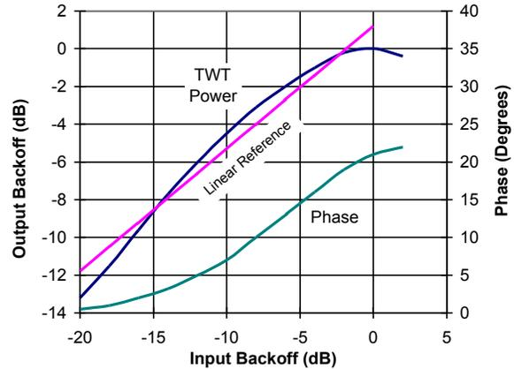
Figure 6. TWT Amplitude And Phase
