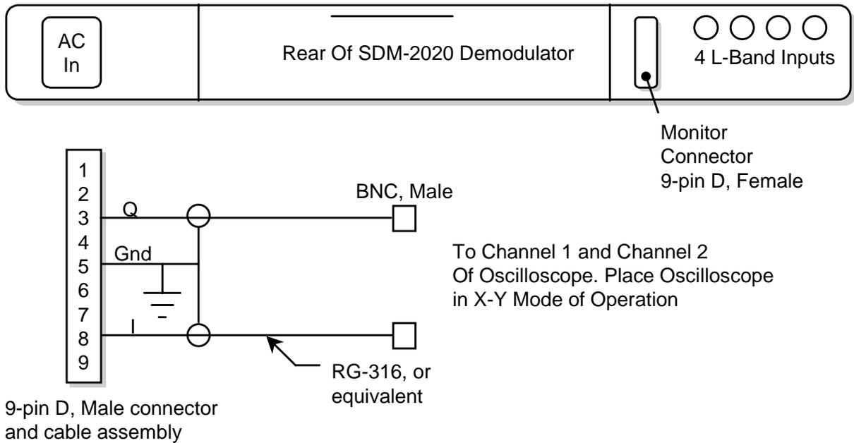
Figure 4 Monitor Connector for Viewing I/Q Constellation on an Oscilloscope
