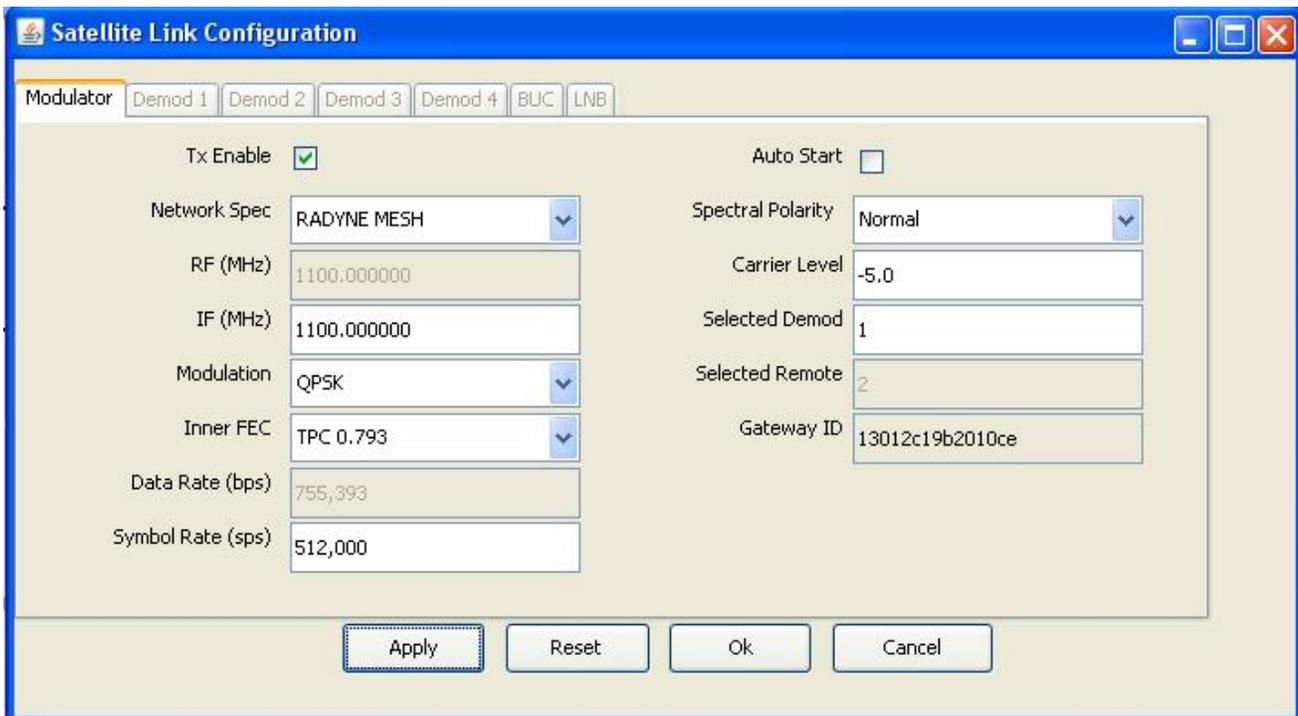
Figure 4-3 Modulator Tab Edit Mode
