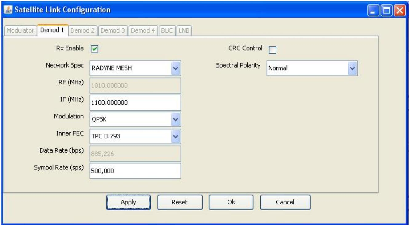
Figure 4-4 Demodulator 1 Tab Edit Mode
