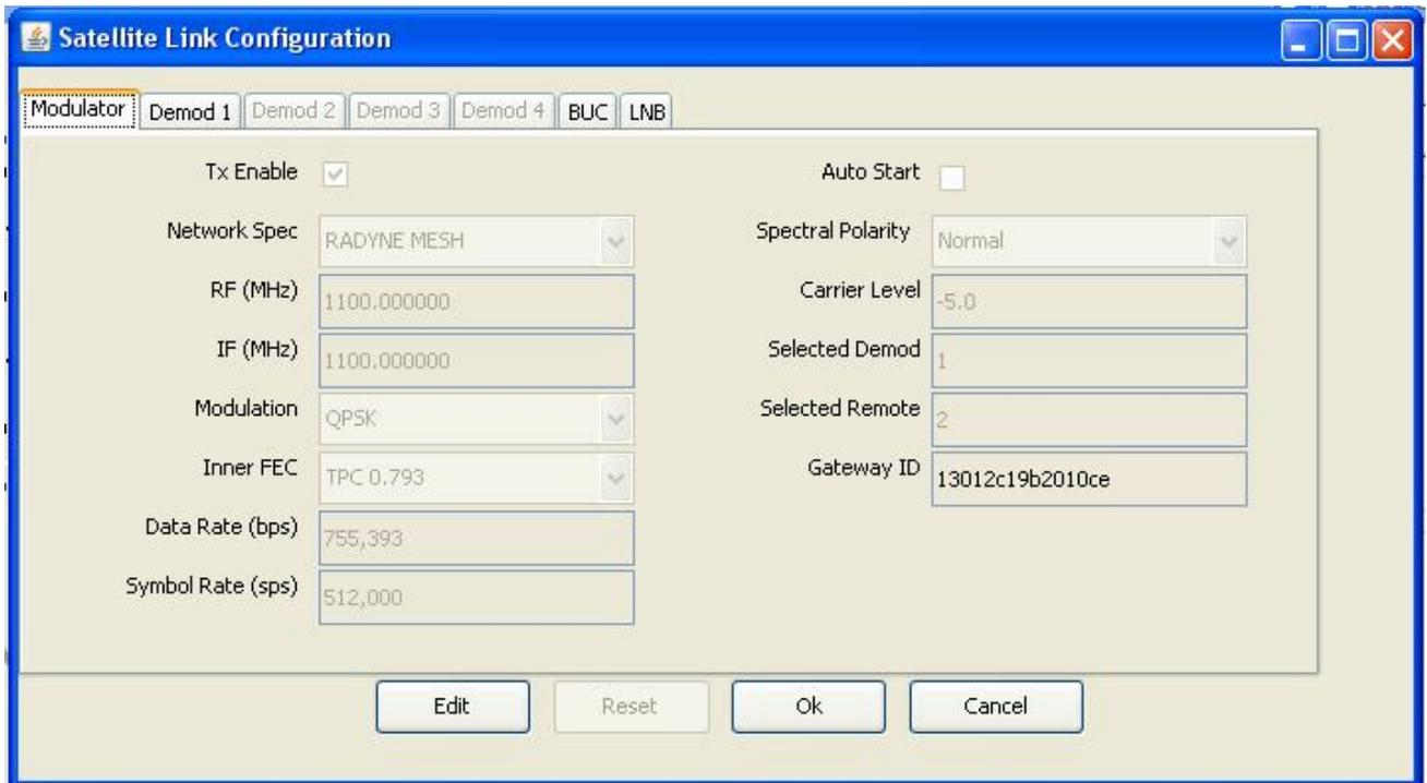
Figure 4-2 Modulator Tab Satellite Link Configuration
