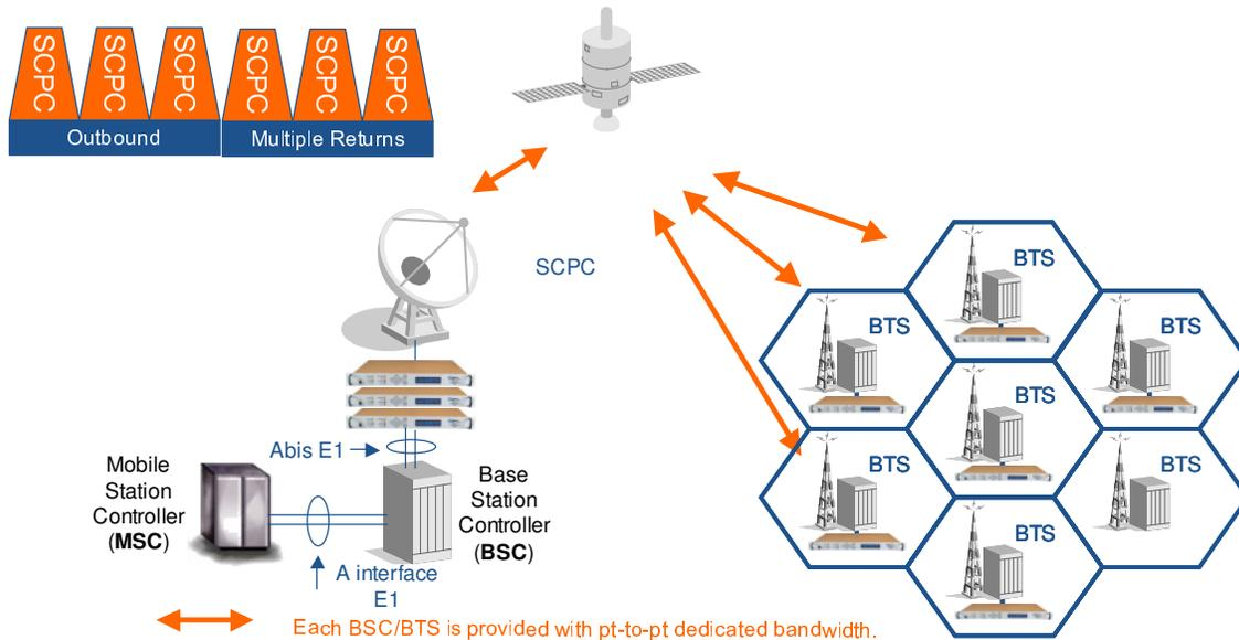
**Figure 2: The Point-to-point SCPC topology.**
