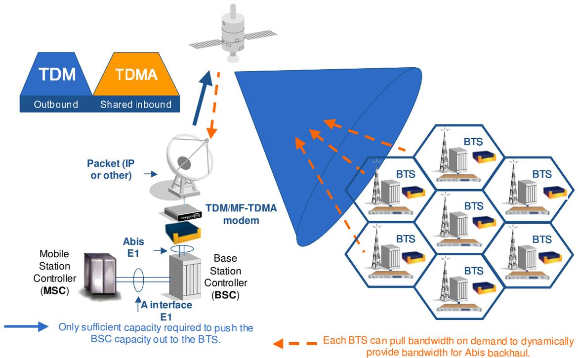
Figure 6: Point-to-multipoint TDM/MF-TDMA solution
