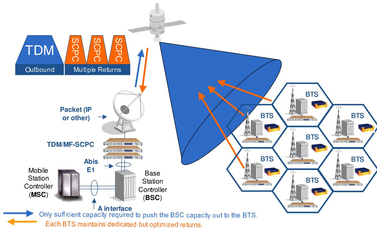
**Figure 5: Point-to-multipoint TDM/MF-SCPC solution (AbisXtender)**
