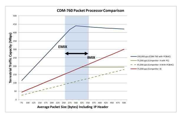
The above graphs depicts the real world impact of user throughput when comparing the CDM-760 modem with available header compression (HC) and payload compression (PC) vs. competitors with various options available.
