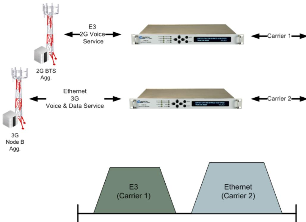
Using Multistream operation, these independent services can be combined into a single carrier while retaining data and clock integrity.
